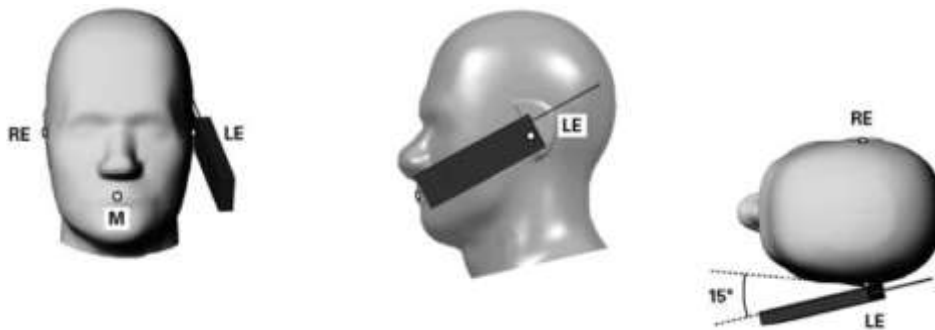
Figure 8.5. Tilt 15° position of the wireless device
