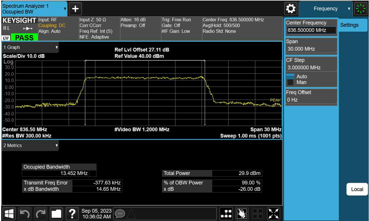
Sub6 n5. Occupied Bandwidth Plot (15 M BW Ch.167300 64QAM_ Full RB_0)
