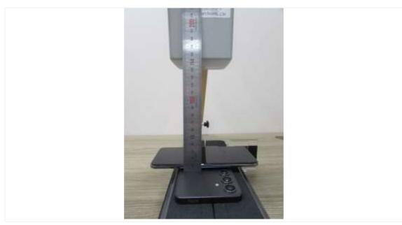
**Top : 20 cm** (The distance between the DUT and the center of the probe is 20 cm.)
