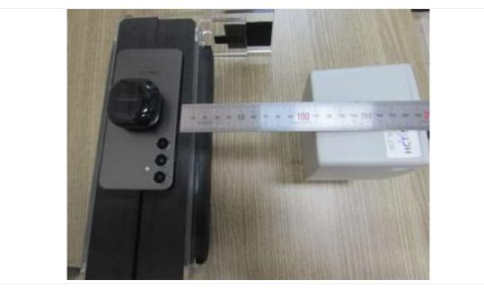
Edge 1:15 cm (The distance between the DUT and the center of the probe is 15 cm.)
