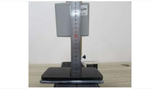
**Bottom : 15 cm** (The distance between the DUT and the center of the probe is 15 cm.)
