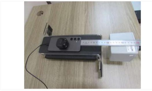
Edge 4 + TA : 15 cm (The distance between the DUT and the center of the probe is 15 cm.)
