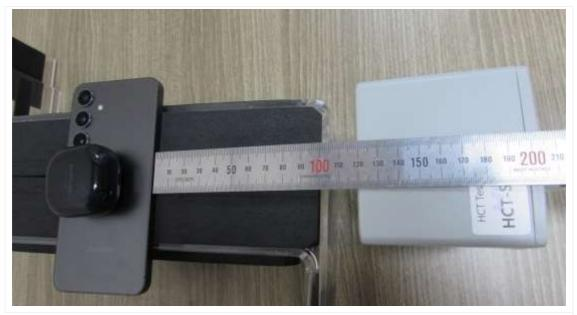
Edge 3:15 cm (The distance between the DUT and the center of the probe is 15 cm.)
