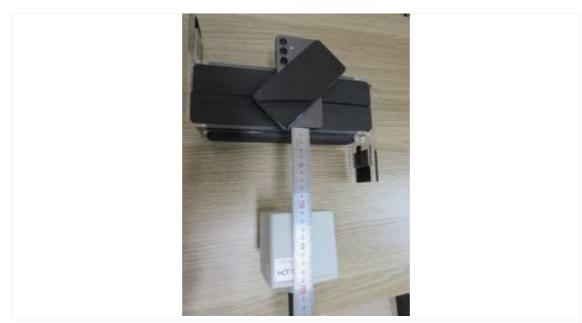
Edge 2: 15 cm (The distance between the DUT and the center of the probe is 15 cm.)
