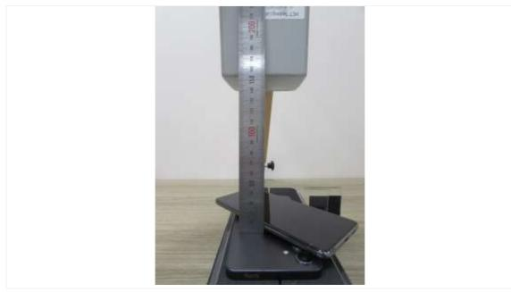
**Top: 20 cm** (The distance between the DUT and the center of the probe is 20 cm.)
