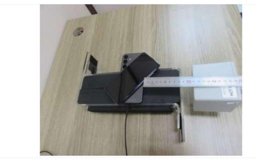
Edge 3 + TA : 15 cm (The distance between the DUT and the center of the probe is 15 cm.)
