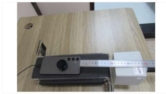
Edge4 + TA : 15 cm (The distance between the DUT and the center of the probe is 15 cm.)
