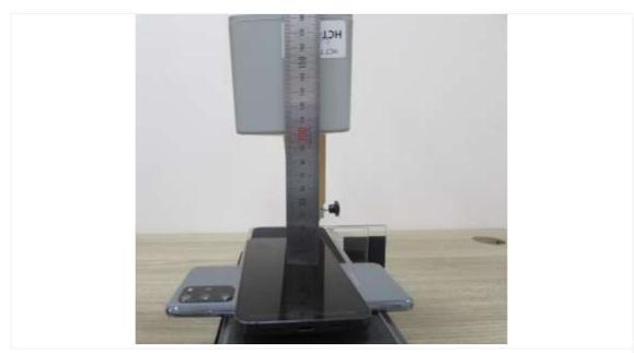
**Bottom : 15 cm** (The distance between the DUT and the center of the probe is 15 cm.)
