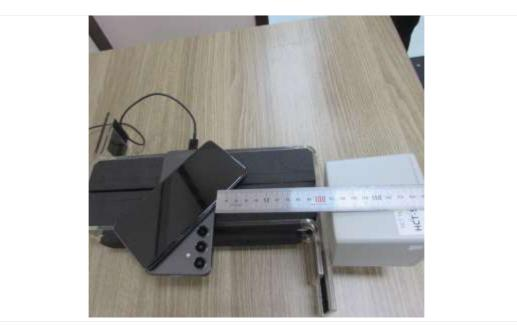
Edge 1 + TA : 15 cm (The distance between the DUT and the center of the probe is 15 cm.)
