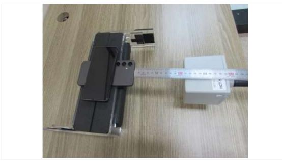
Edge 4:15 cm (The distance between the DUT and the center of the probe is 15 cm.)
