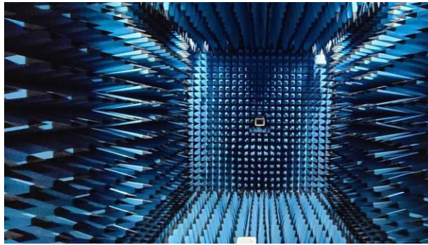
Figure 2: Geometry of Anechoic Chamber for Radiation patterns.
