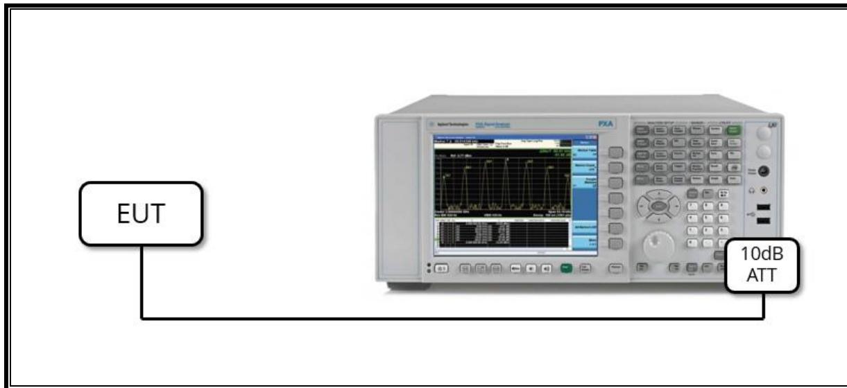
**SETUP DIAGRAM FOR TESTS (RADIATED TEST SETUP)**
