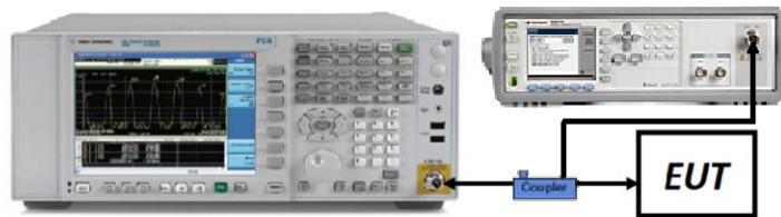
Figure 7-3. Test Instrument & Measurement Setup
