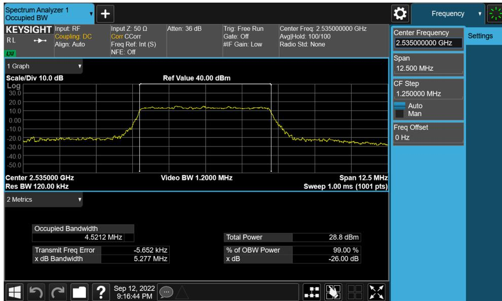
Plot 7-64. Occupied Bandwidth Plot (NR Band n7 - 5MHz 16-QAM - Full RB - Ant B)
