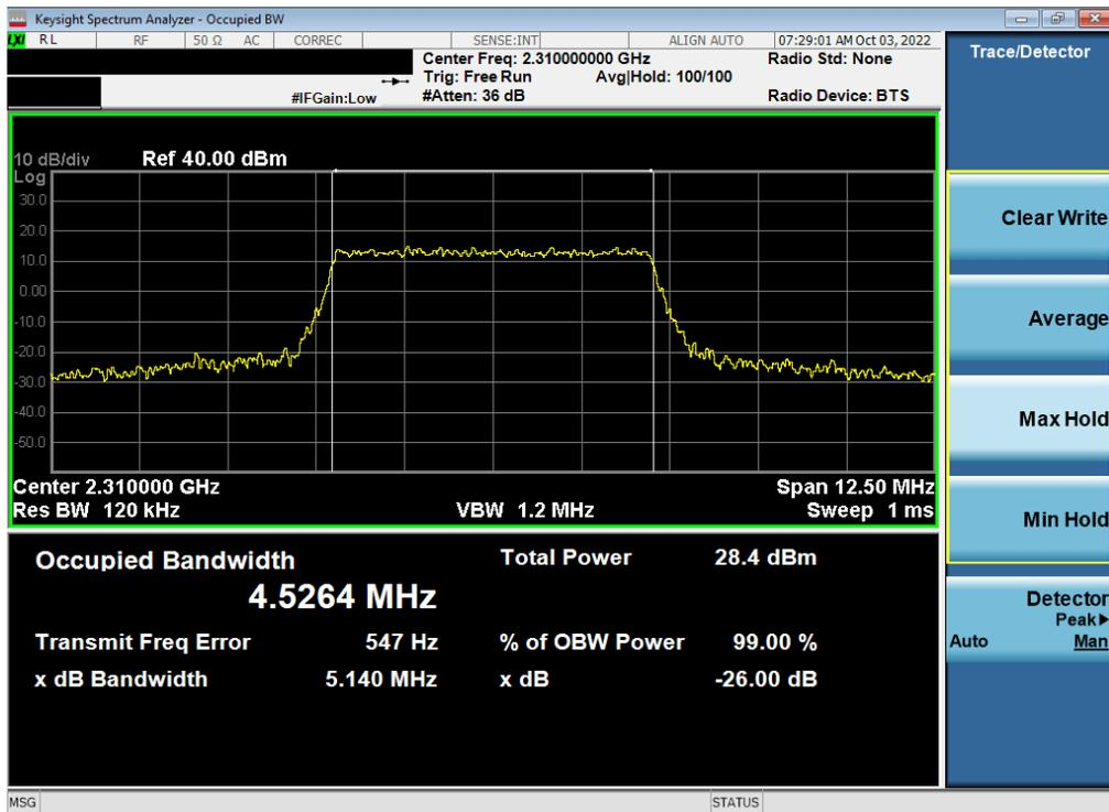
Plot 7-8. Occupied Bandwidth Plot (LTE Band 30 - 5MHz 16-QAM - Full RB - Ant F)
