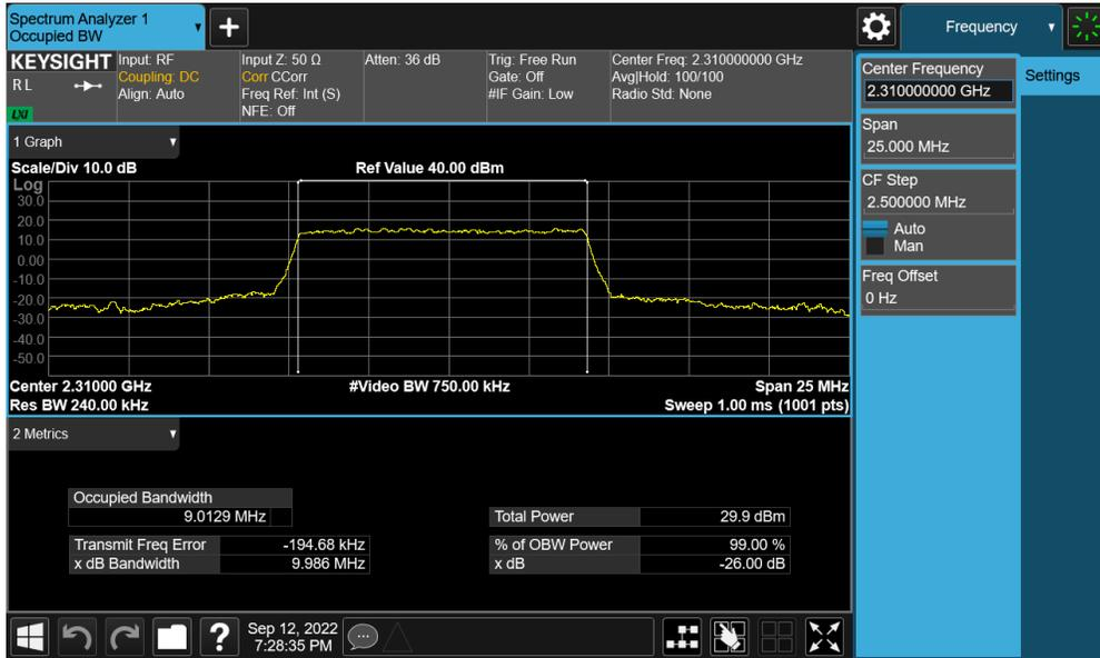
Plot 7-41. Occupied Bandwidth Plot (NR Band n30 - 10MHz  $\pi/2$  BPSK - Full RB - Ant A)
