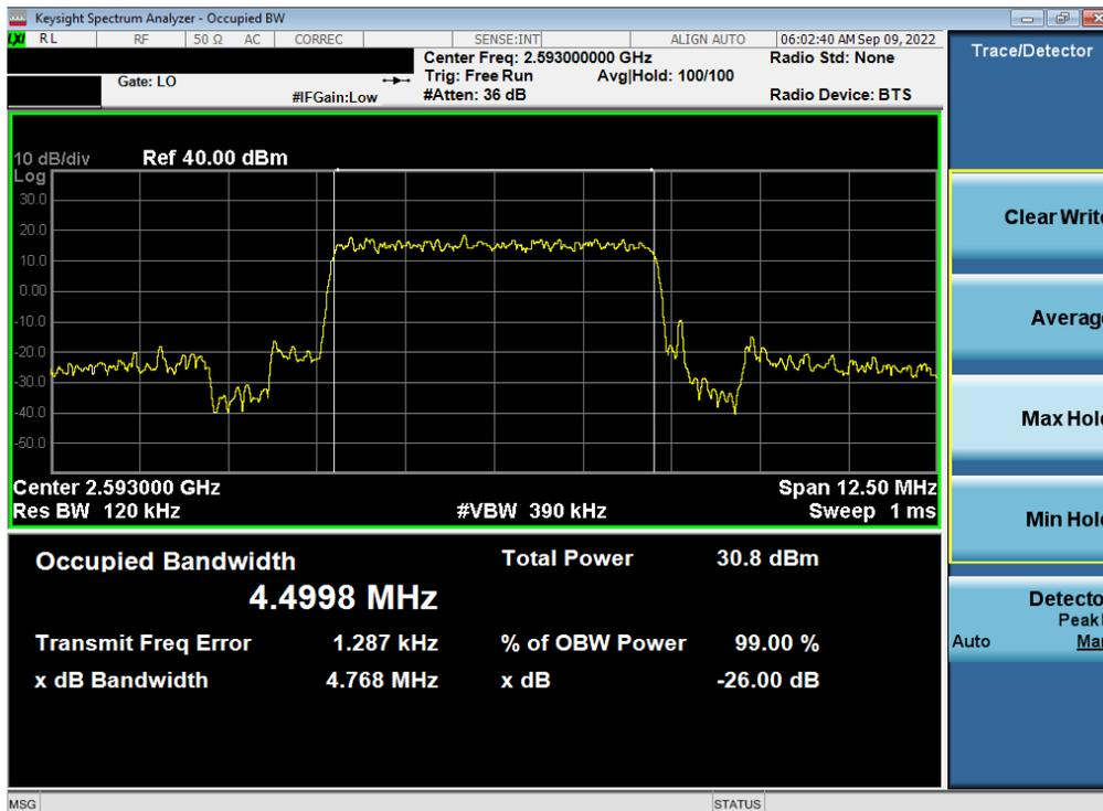
Plot 7-32. Occupied Bandwidth Plot (LTE Band 41(PCI) - 5MHz 16-QAM - Full RB - Ant B)
