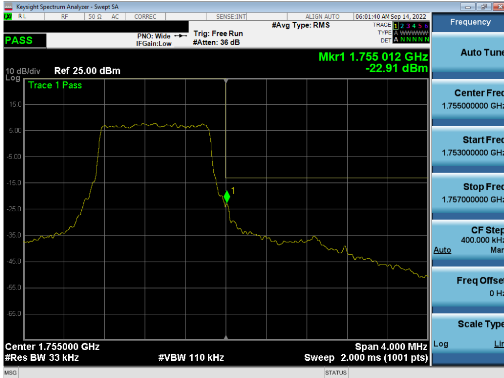
Plot 7-291. Upper Band Edge Plot (LTE Band 4 – 1.4MHz QPSK – Full RB - Ant A)
