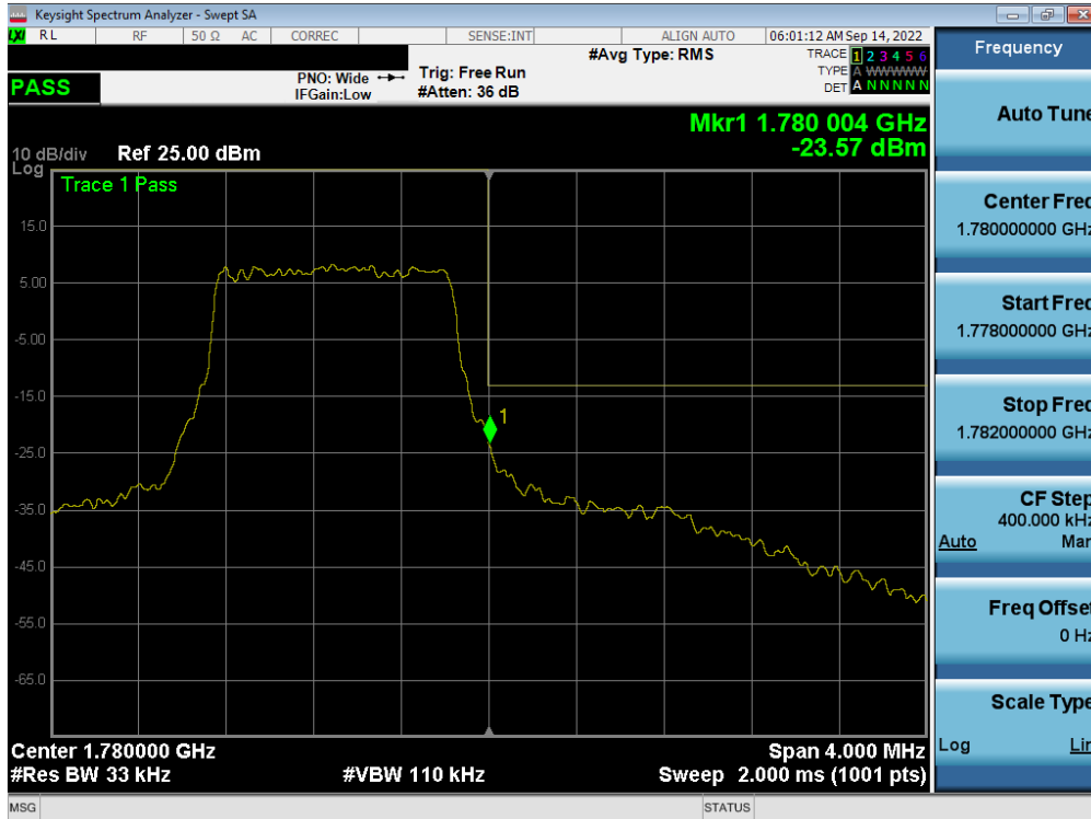
Plot 7-293. Upper Band Edge Plot (LTE Band 66 – 1.4MHz QPSK – Full RB - Ant A)
