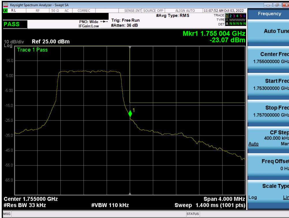
Plot 7-359. Upper Band Edge Plot (LTE Band 4 – 1.4MHz QPSK – Full RB - Ant F)
