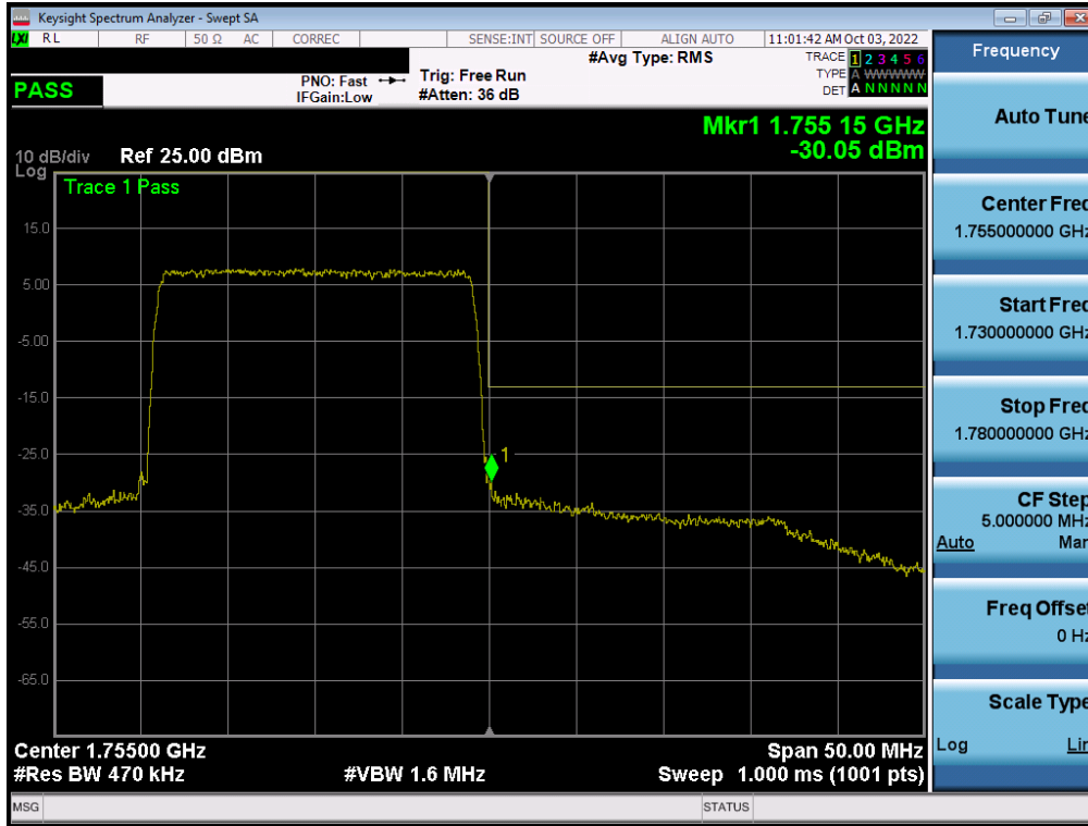
Plot 7-329. Upper Band Edge Plot (LTE Band 4 - 20MHz QPSK – Full RB - Ant F)
