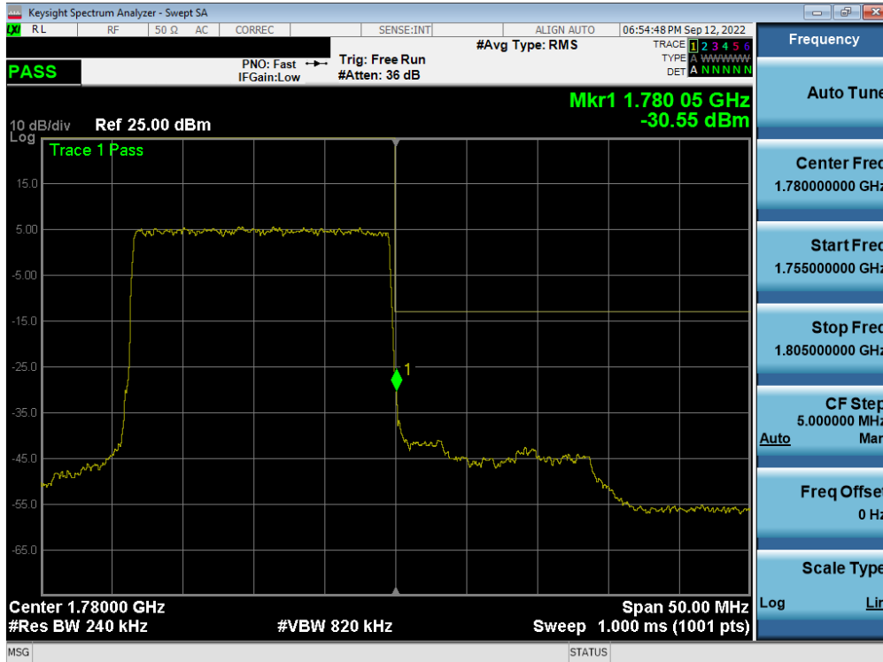
Plot 7-309. Upper Band Edge Plot (NR Band n66 – 20.0MHz - Full RB - Ant A)
