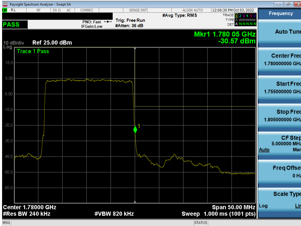
Plot 7-377. Upper Band Edge Plot (NR Band n66 – 20.0MHz - Full RB - Ant F)
