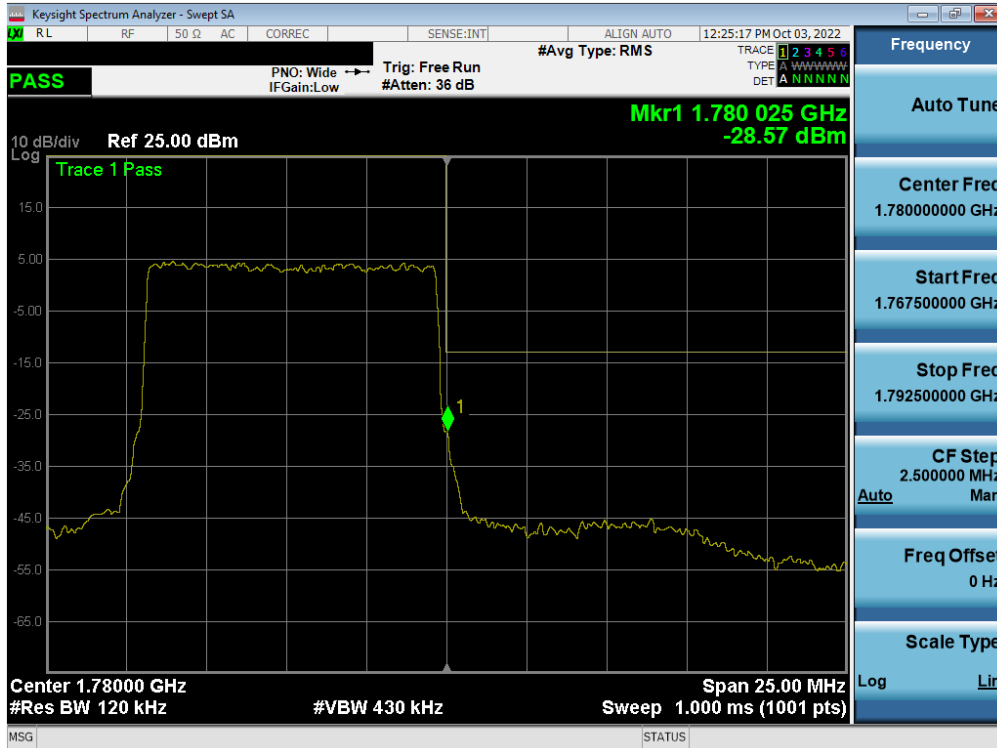
Plot 7-385. Upper Band Edge Plot (NR Band n66 – 10.0MHz - Full RB - Ant F)
