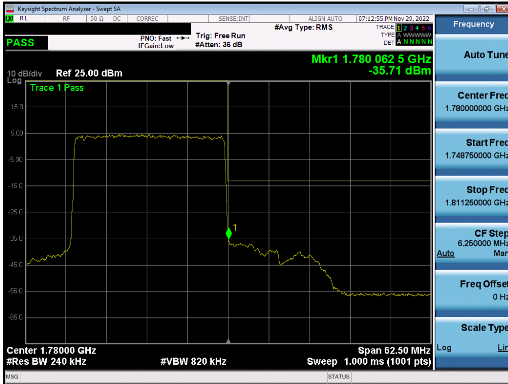
Plot 7-305. Upper Band Edge Plot (NR Band n66 – 25.0MHz - Full RB - Ant A)
