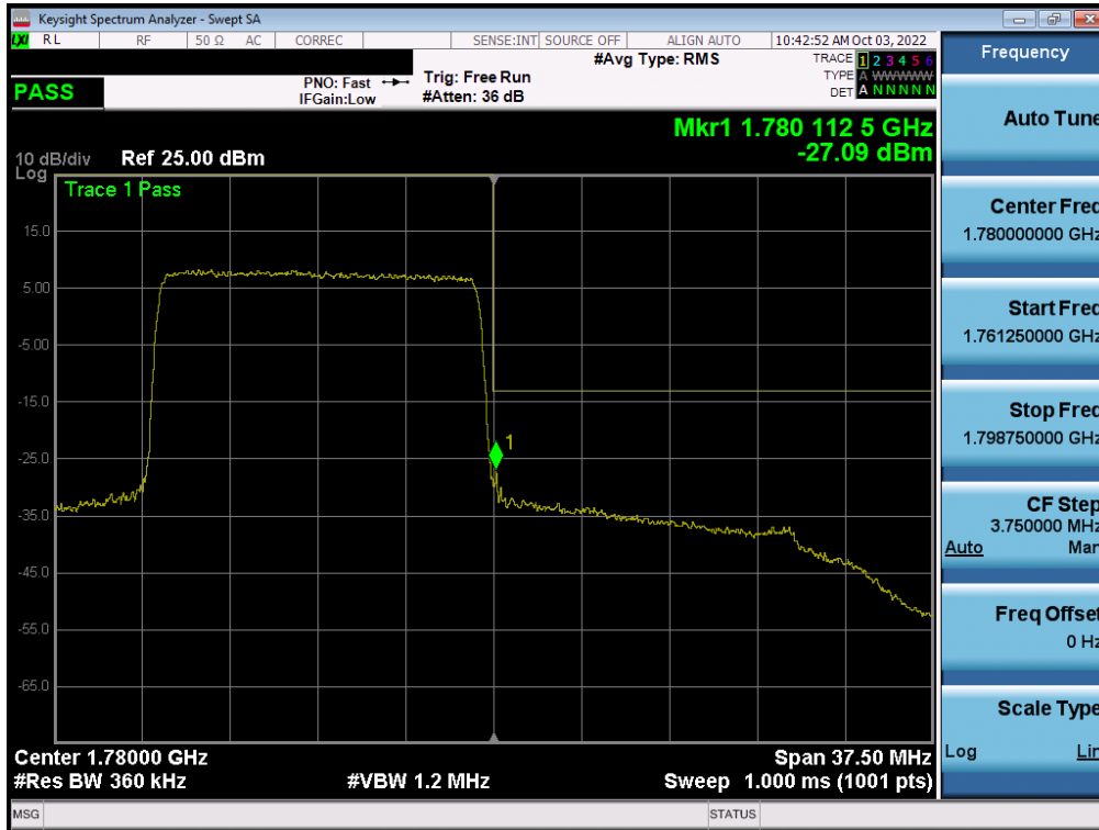
Plot 7-337. Upper Band Edge Plot (LTE Band 66 - 15MHz QPSK – Full RB - Ant F)
