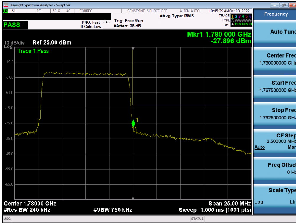
Plot 7-343. Upper Band Edge Plot (LTE Band 66 - 10MHz QPSK – Full RB - Ant F)
