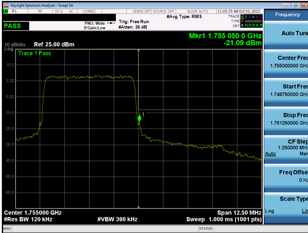
Plot 7-347. Upper Band Edge Plot (LTE Band 4 - 5MHz QPSK – Full RB - Ant F)
