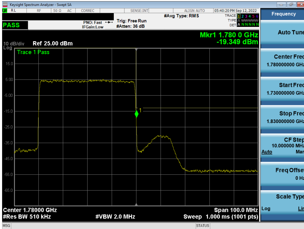
Plot 7-297. Upper Band Edge Plot (NR Band n66 – 40.0MHz - Full RB - Ant A)
