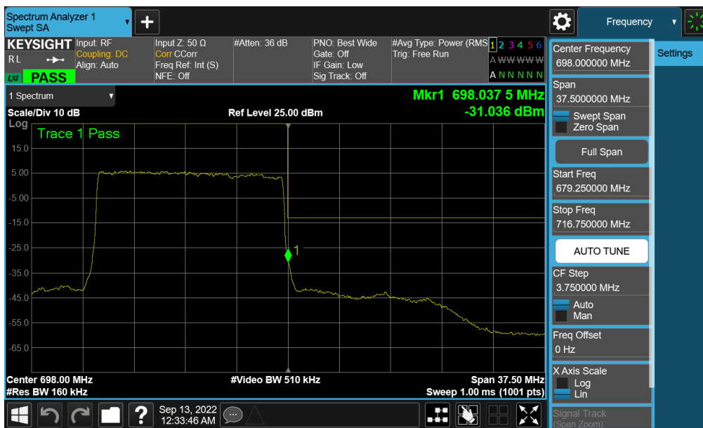
Plot 7-244. Upper Band Edge Plot (NR Band n71 – 15.0MHz - Full RB - Ant A)
