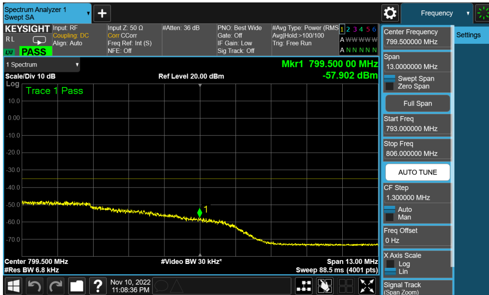
Plot 7-236. Upper Emission Mask Plot (LTE Band 13 - 10MHz QPSK – Full RB - Ant A)
