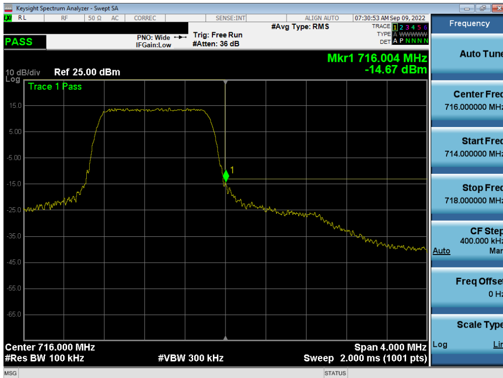
Plot 7-232. Upper Band Edge Plot (LTE Band 12 – 1.4MHz QPSK – Full RB - Ant A)
