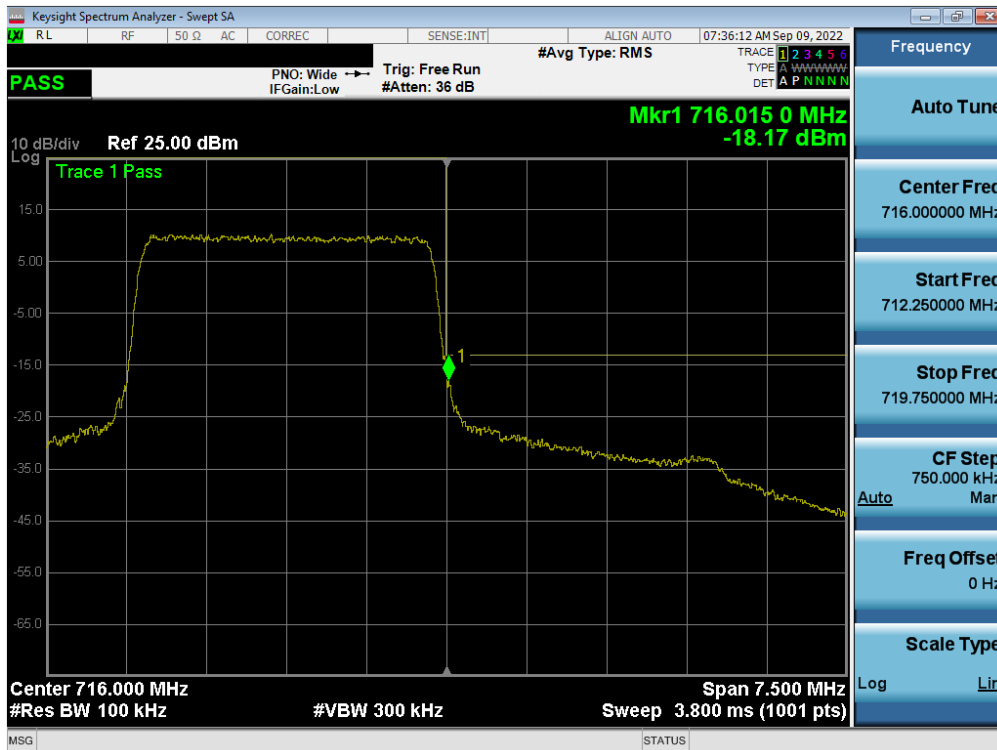
Plot 7-230. Upper Band Edge Plot (LTE Band 12 - 3MHz QPSK – Full RB - Ant A)
