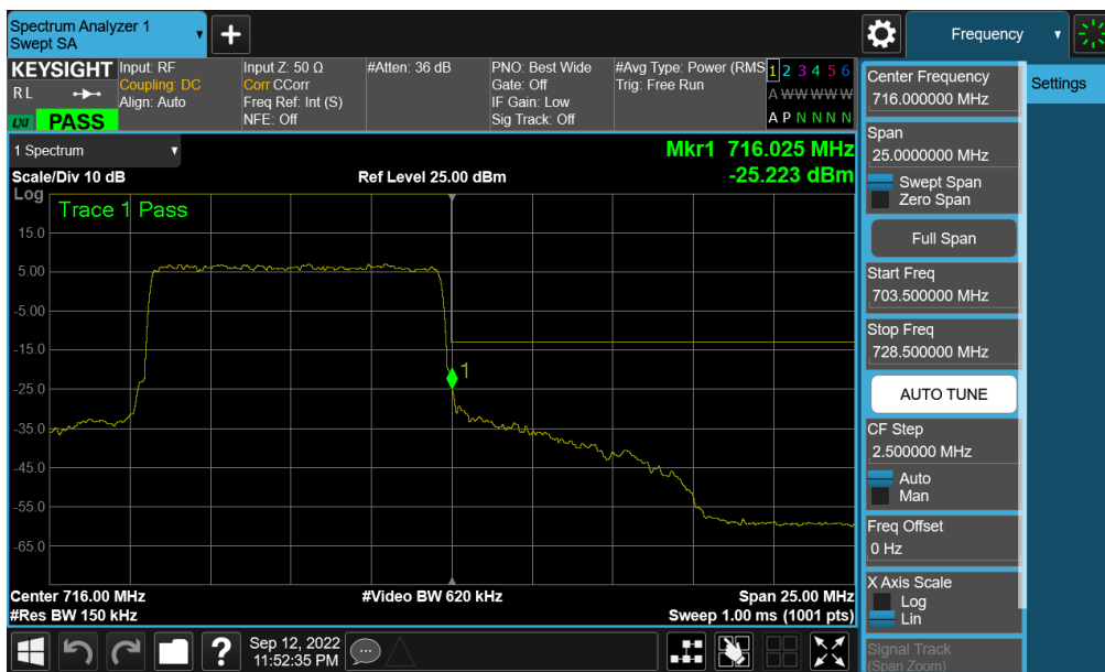
Plot 7-252. Upper Band Edge Plot (NR Band n12 – 10.0MHz - Full RB - Ant A)
