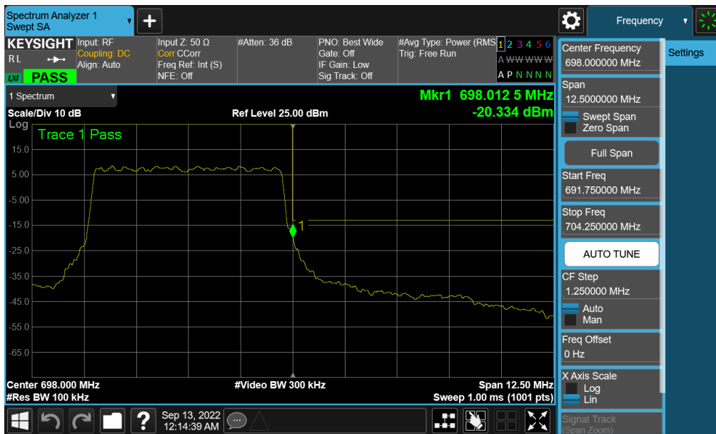
Plot 7-248. Upper Band Edge Plot (NR Band n71 - 5.0MHz - Full RB - Ant A)
