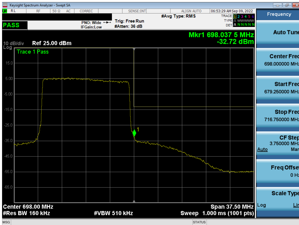
Plot 7-220. Upper Band Edge Plot (LTE Band 71 - 15MHz QPSK – Full RB - Ant A)
