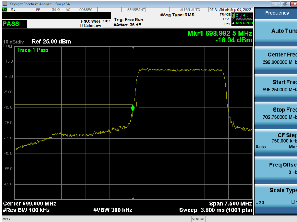
Plot 7-229. Lower Band Edge Plot (LTE Band 12 - 3MHz QPSK – Full RB - Ant A)
