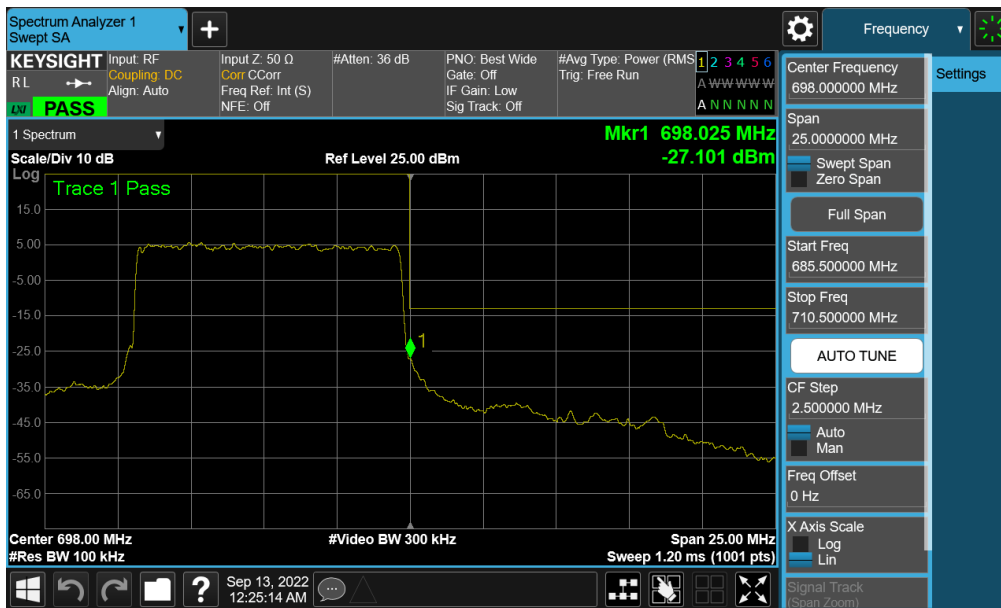
Plot 7-246. Upper Band Edge Plot (NR Band n71 – 10.0MHz - Full RB - Ant A)
