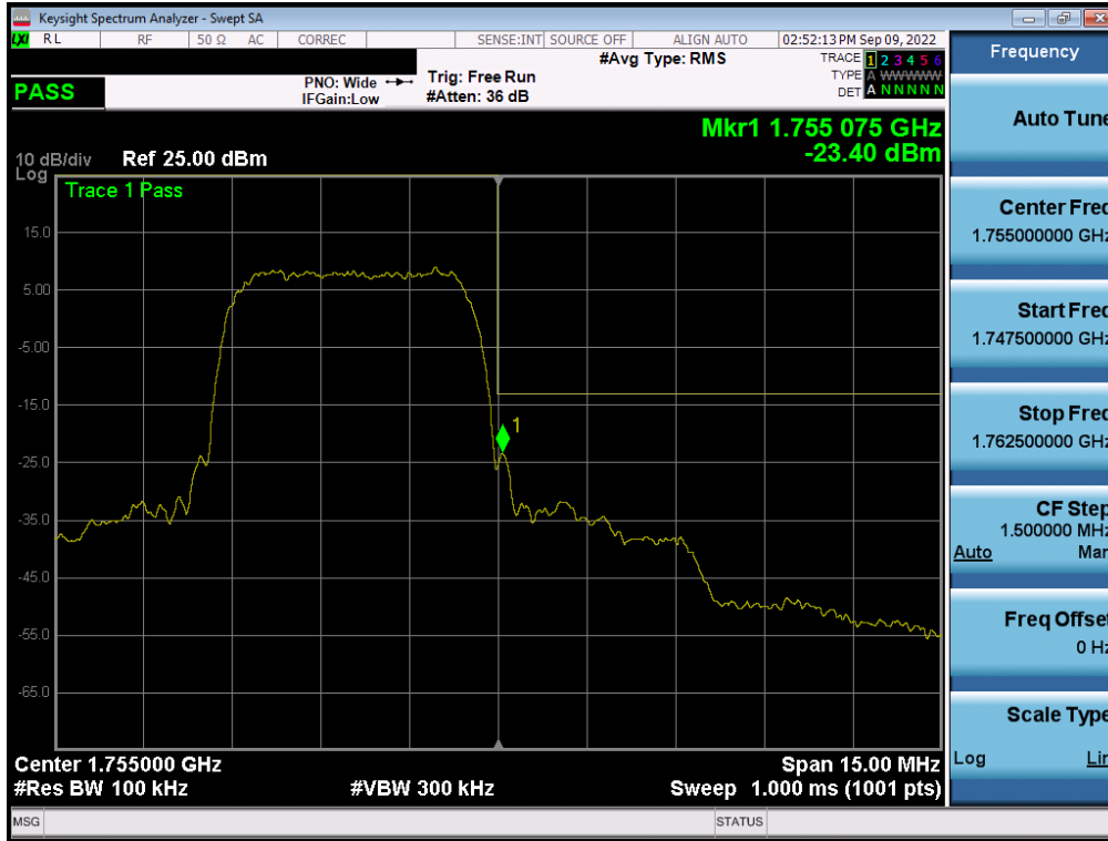
Plot 7-257. Upper Band Edge Plot (WCDMA AWS – Ch. 1513 – Ant A)
