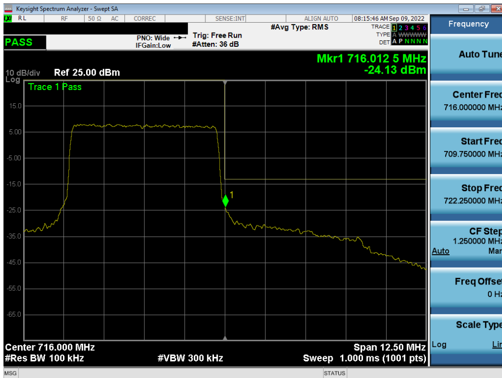
Plot 7-228. Upper Band Edge Plot (LTE Band 12 - 5MHz QPSK – Full RB - Ant A)
