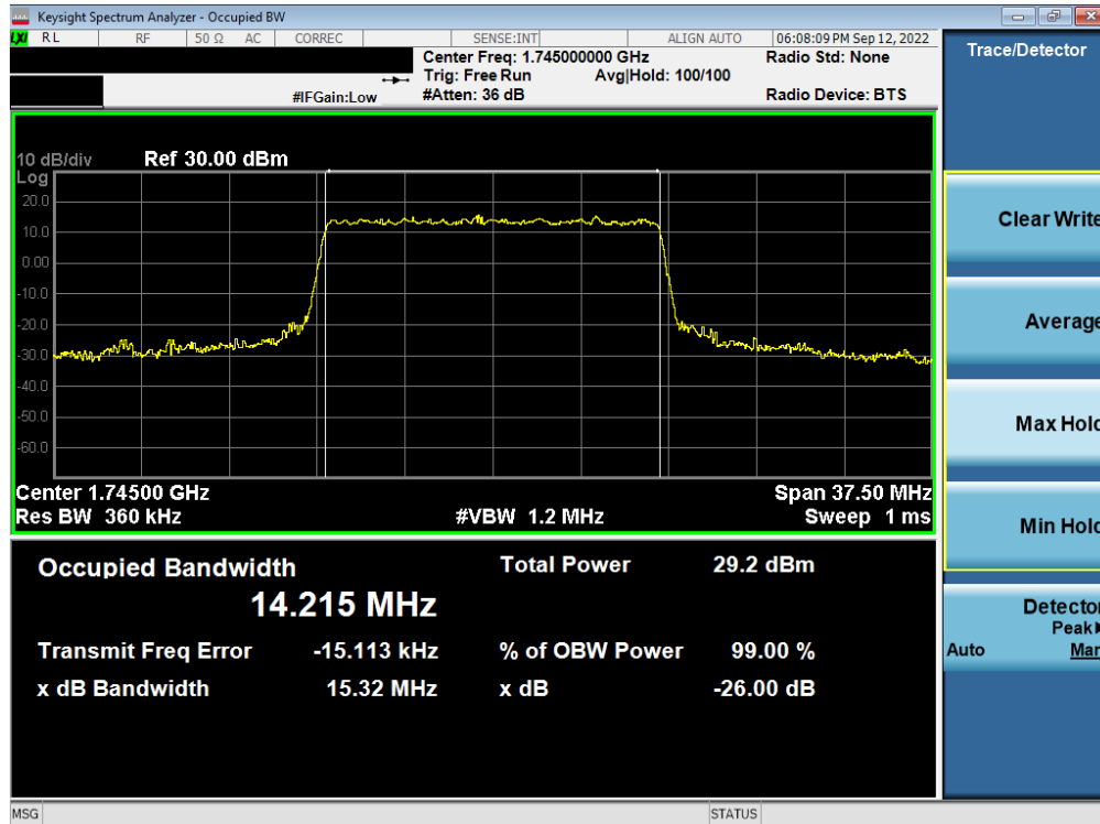
Plot 7-68. Occupied Bandwidth Plot (NR Band n66 - 15.0MHz CP-OFDM QPSK - Full RB – Ant A)
