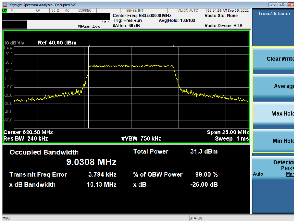
Plot 7-6. Occupied Bandwidth Plot (LTE Band 71 - 10MHz 16-QAM - Full RB – Ant A)
