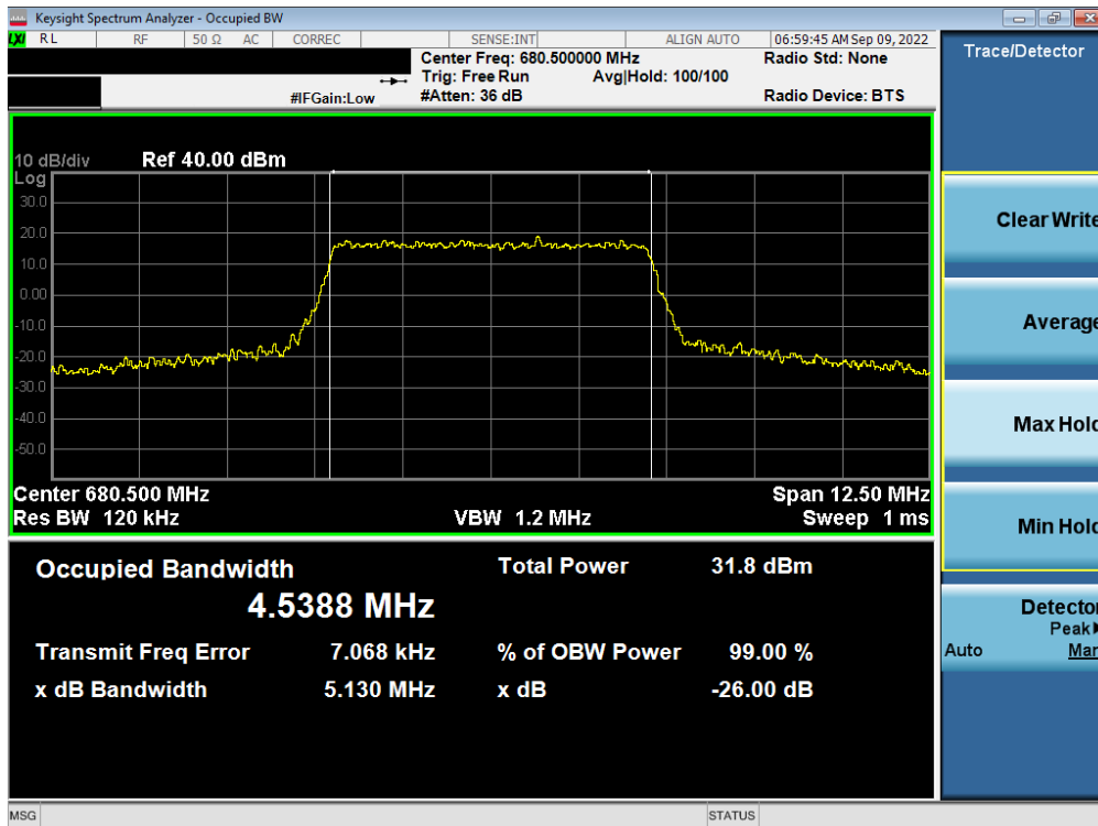
Plot 7-8. Occupied Bandwidth Plot (LTE Band 71 - 5MHz 16-QAM - Full RB – Ant A)
