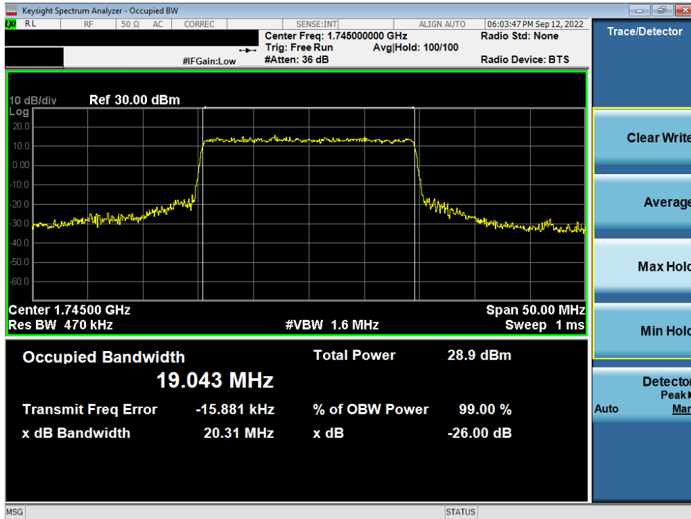
Plot 7-66. Occupied Bandwidth Plot (NR Band n66 - 20.0MHz CP-OFDM 16QAM - Full RB – Ant A)
