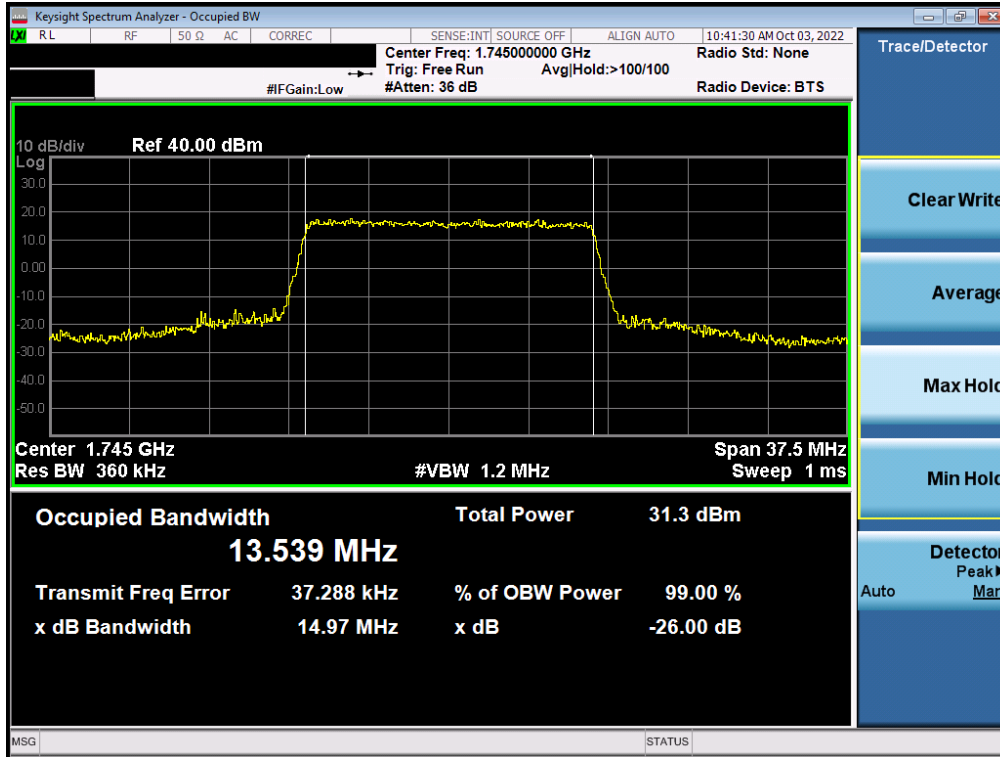
Plot 7-78. Occupied Bandwidth Plot (LTE Band 66/4 - 15MHz QPSK - Full RB - Ant F)
