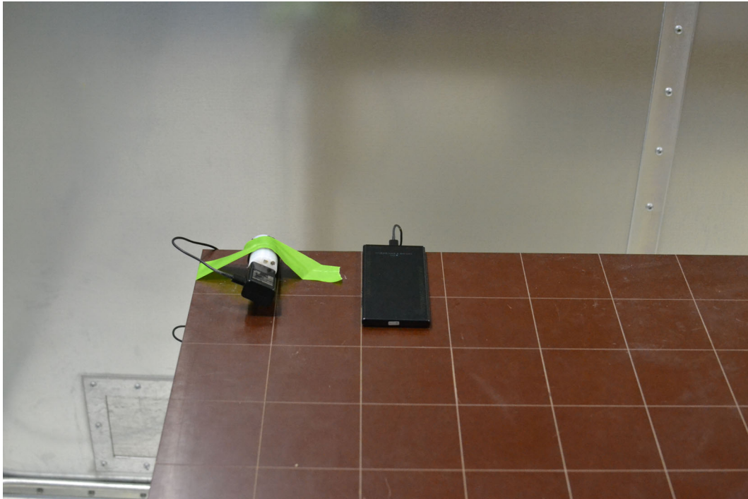
Figure 1. Test Setup – ACLC– <30MHz
