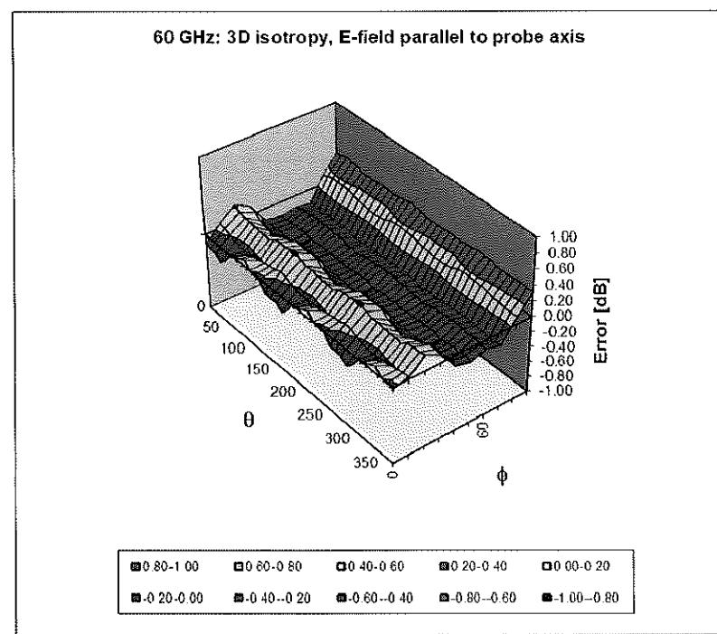
Probe isotropy for  $E_{\text{tot}}$ : probe rotated  $\varphi = 0^\circ$  to  $360^\circ$ , tilted from field propagation direction  $\vec{k}$
