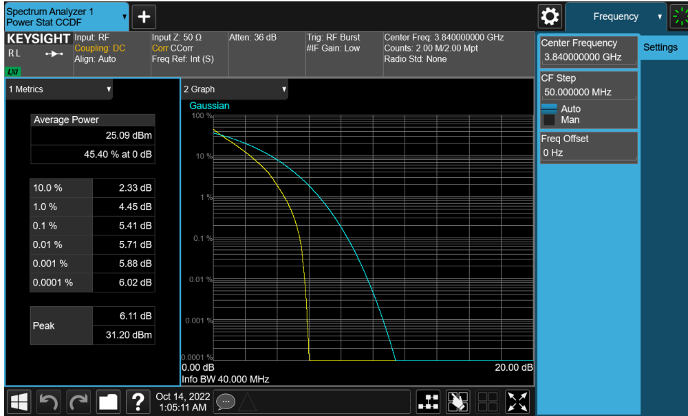
Plot 7-235. PAR Plot (NR Band n77 - C-Band – 40MHz DFT-s-OFDM \pi/2 BPSK - Full RB)
