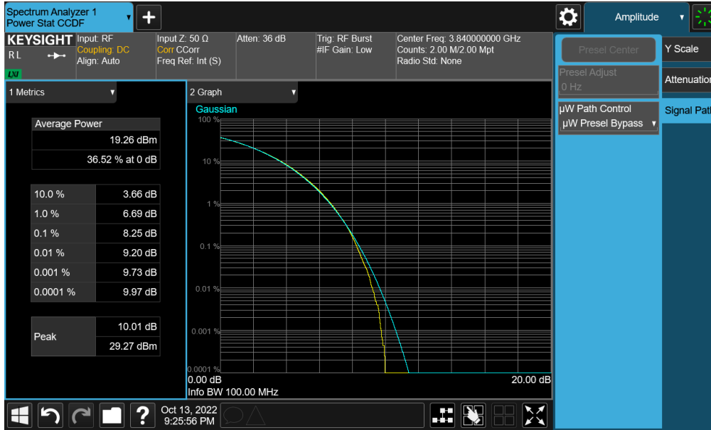
Plot 7-219. PAR Plot (NR Band n77 - C-Band – 100MHz CP-OFDM 256-QAM - Full RB)
