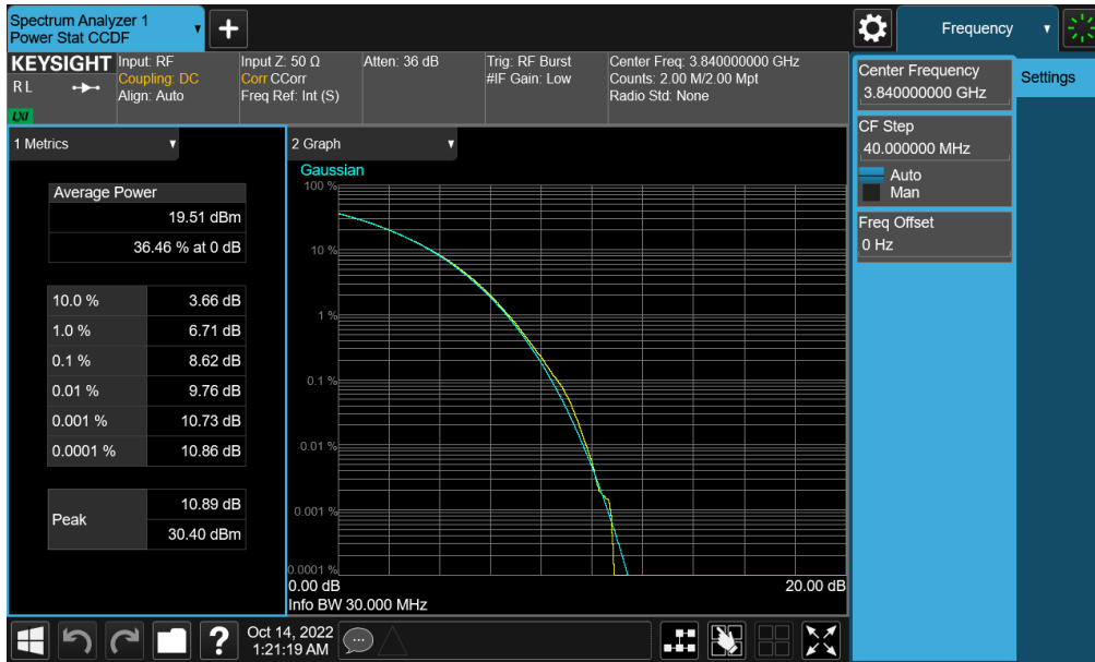
Plot 7-240. PAR Plot (NR Band n77 - C-Band – 30MHz CP-OFDM 256-QAM - Full RB)
