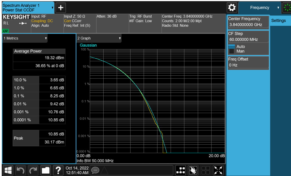
Plot 7-234. PAR Plot (NR Band n77 - C-Band – 50MHz CP-OFDM 256-QAM - Full RB)
