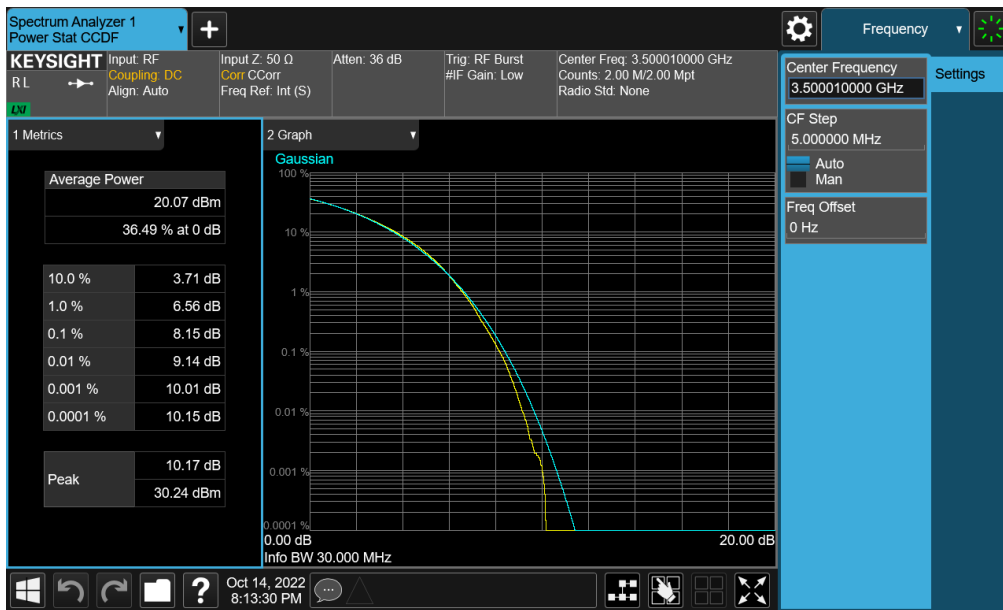
Plot 7-204. PAR Plot (NR Band n77 - DoD Band – 30MHz CP-OFDM 256-QAM - Full RB)
