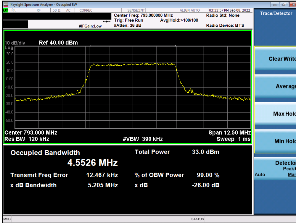
Plot 7-3. Occupied Bandwidth Plot (LTE Band 14 - 5MHz QPSK - Full RB)
