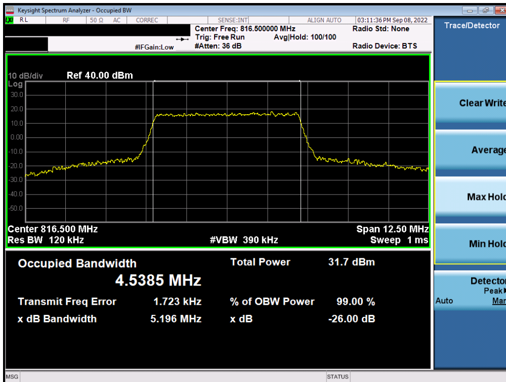
Plot 7-10. Occupied Bandwidth Plot (LTE Band 26 - 5MHz 16-QAM - Full RB)
