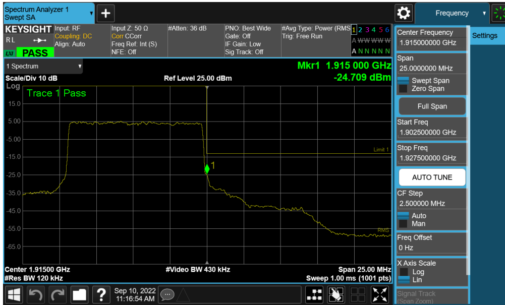
Plot 7-224. Upper Band Edge Plot (NR Band n25 - 10MHz QPSK – Full RB - ANT A)
