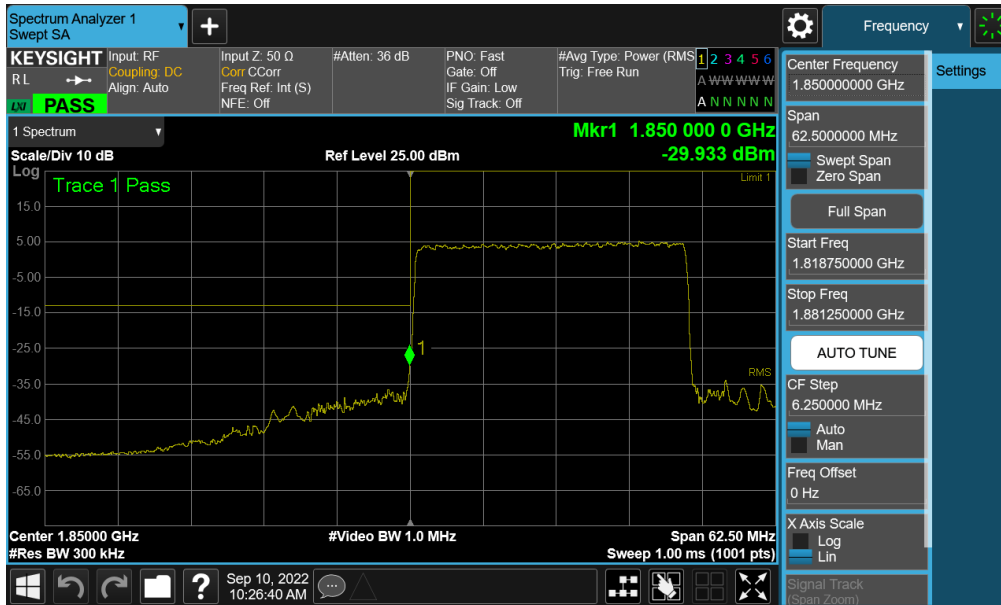
Plot 7-204. Lower Band Edge Plot (NR Band n25 - 25MHz QPSK – Full RB - ANT A)
