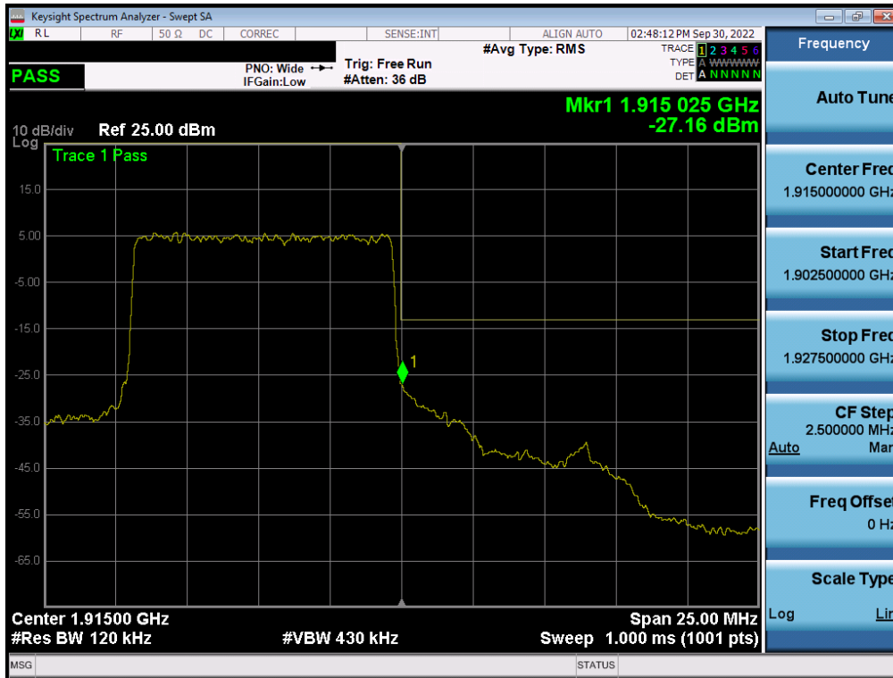
Plot 7-260. Upper Band Edge Plot (NR Band n25 - 10MHz QPSK – Full RB - ANT F)
