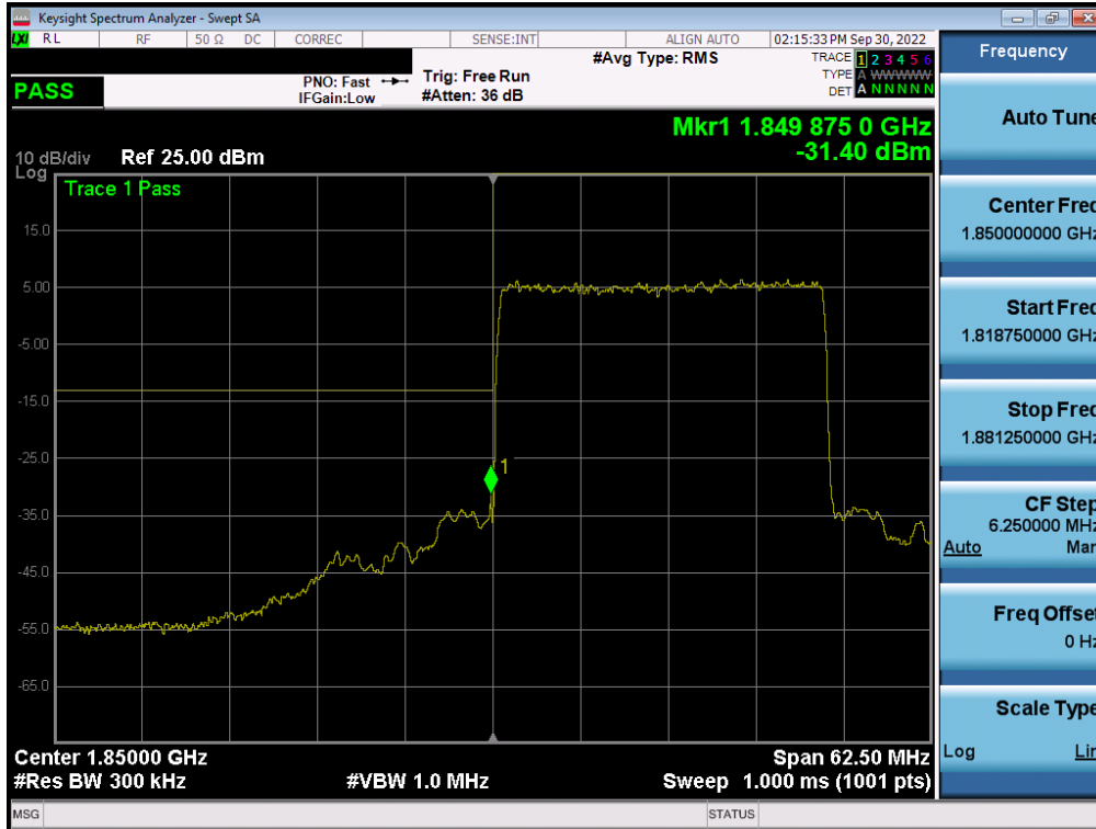
Plot 7-240. Lower Band Edge Plot (NR Band n25 - 25MHz QPSK – Full RB - ANT F)
