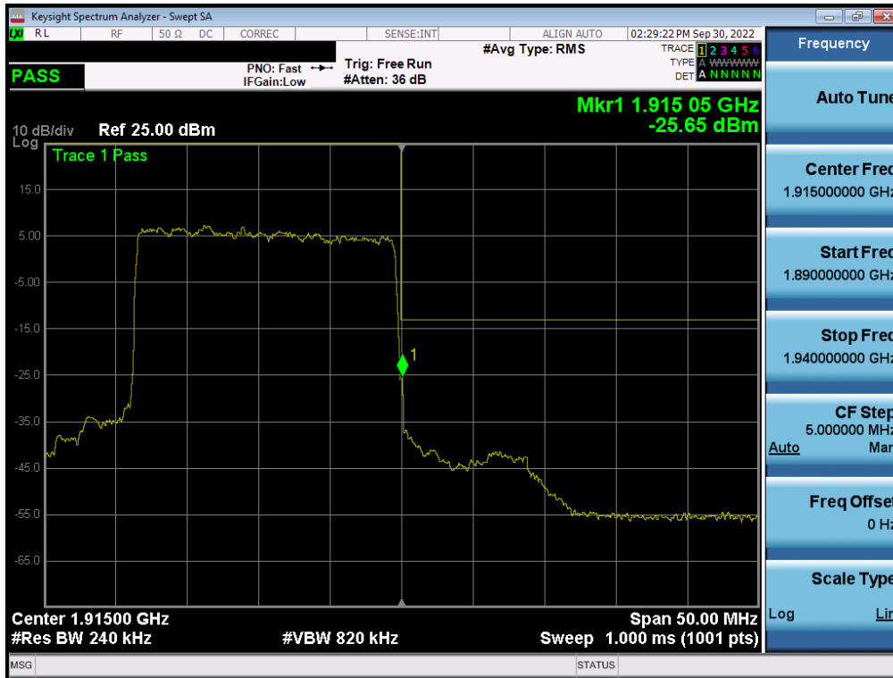
Plot 7-248. Upper Band Edge Plot (NR Band n25 - 20MHz QPSK – Full RB - ANT F)
