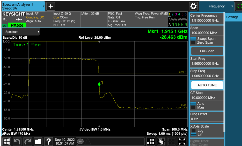
Plot 7-198. Upper Band Edge Plot (NR Band n25 - 40MHz QPSK – Full RB - ANT A)
