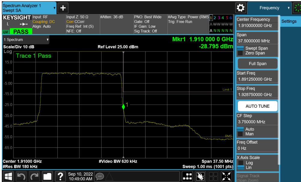
Plot 7-216. Upper Band Edge Plot (NR Band n2 - 15MHz QPSK – Full RB - ANT A)
