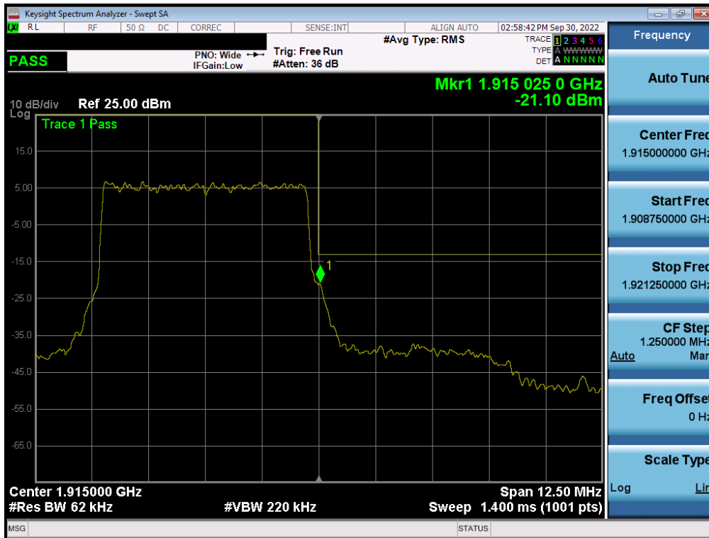
Plot 7-266. Upper Band Edge Plot (NR Band n25 – 5MHz QPSK – Full RB - ANT F)
