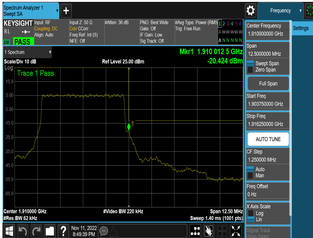
Plot 7-264. Upper Band Edge Plot (NR Band n2 – 5MHz QPSK – Full RB - ANT F)
