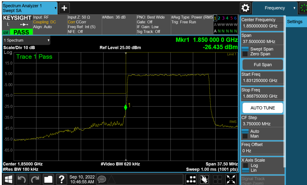
Plot 7-214. Lower Band Edge Plot (NR Band n25/2 - 15MHz QPSK – Full RB - ANT A)
