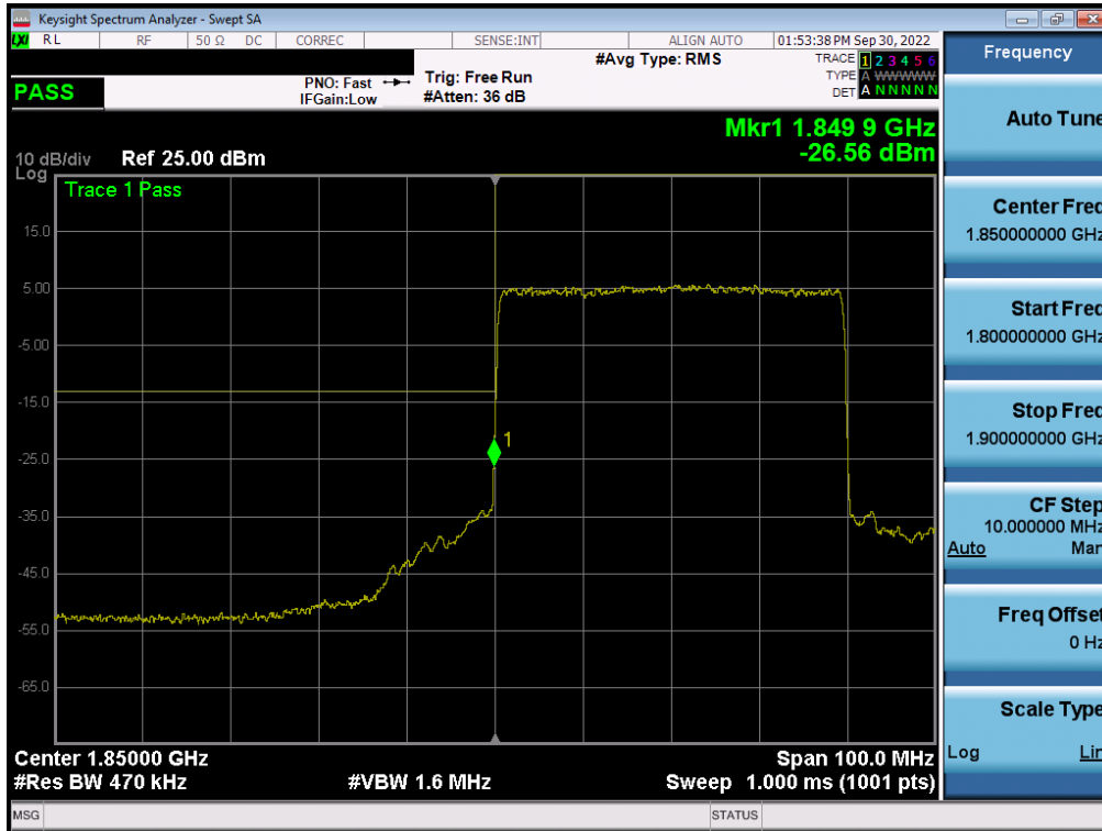
Plot 7-232. Lower Band Edge Plot (NR Band n25 - 40MHz QPSK – Full RB - ANT F)
