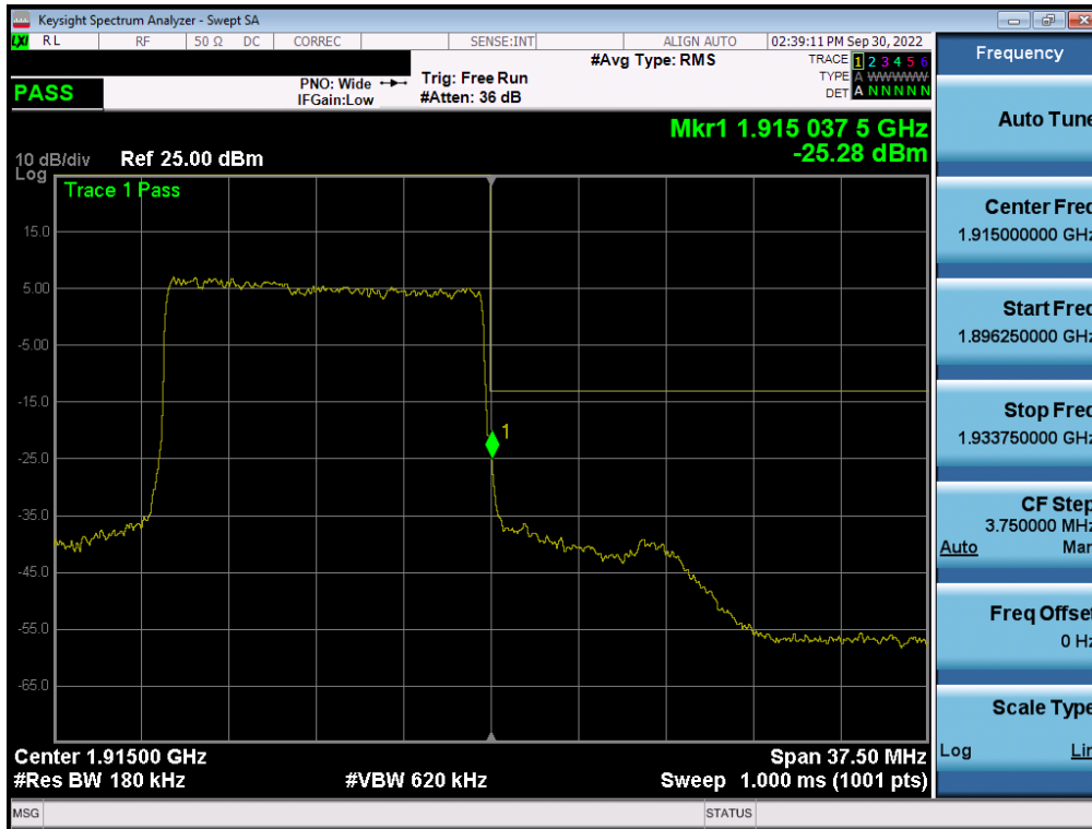
Plot 7-254. Upper Band Edge Plot (NR Band n25 - 15MHz QPSK – Full RB - ANT F)
