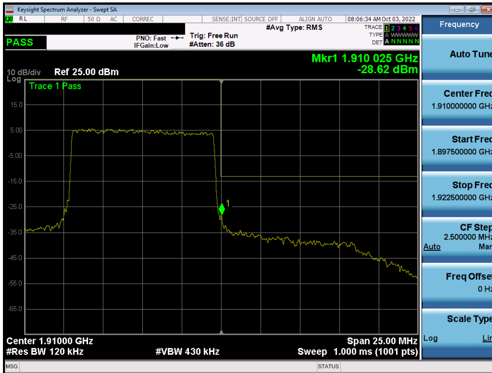
Plot 7-174. Upper Band Edge Plot (LTE Band 2 - 10MHz QPSK – Full RB - ANT F)
