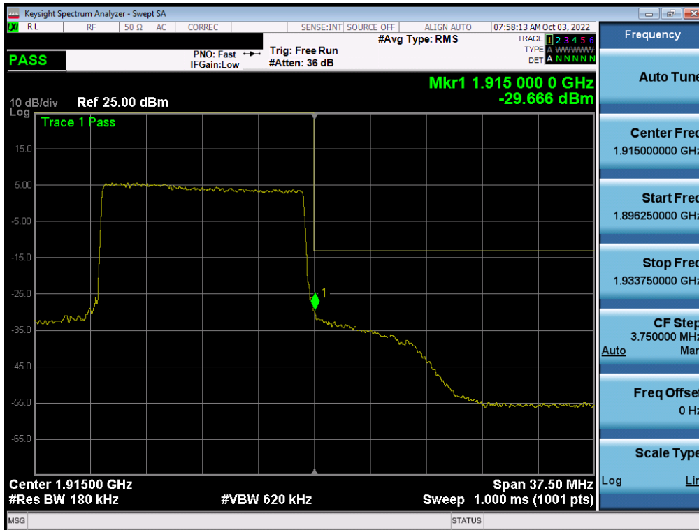
Plot 7-170. Upper Band Edge Plot (LTE Band 25 - 15MHz QPSK – Full RB - ANT F)
