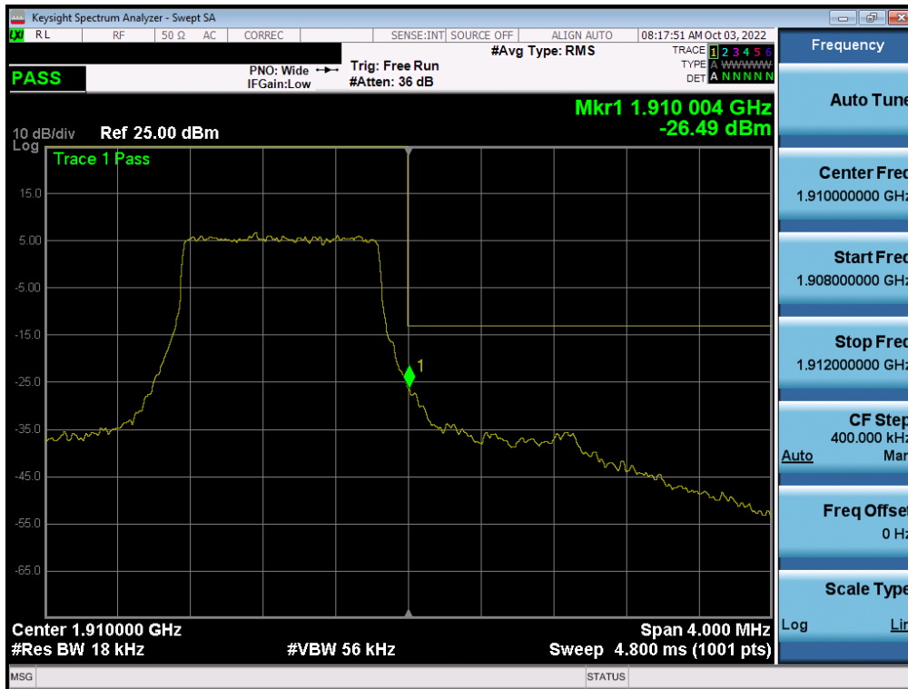
Plot 7-192. Upper Band Edge Plot (LTE Band 2 – 1.4MHz QPSK – Full RB - ANT F)
