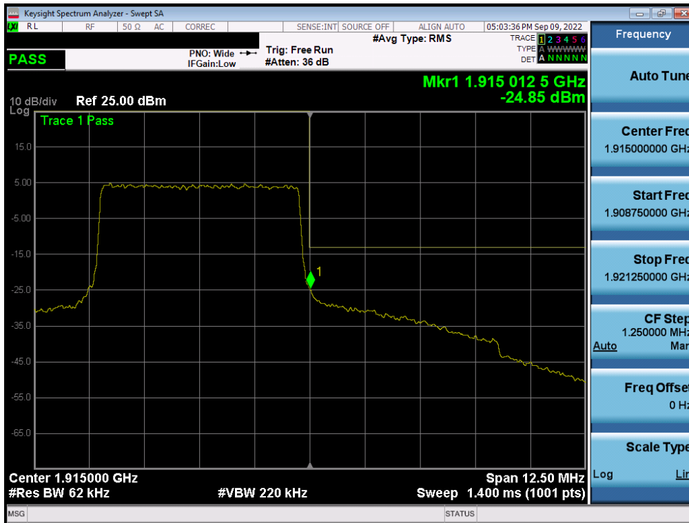
Plot 7-146. Upper Band Edge Plot (LTE Band 25 - 5MHz QPSK – Full RB - ANT A)
