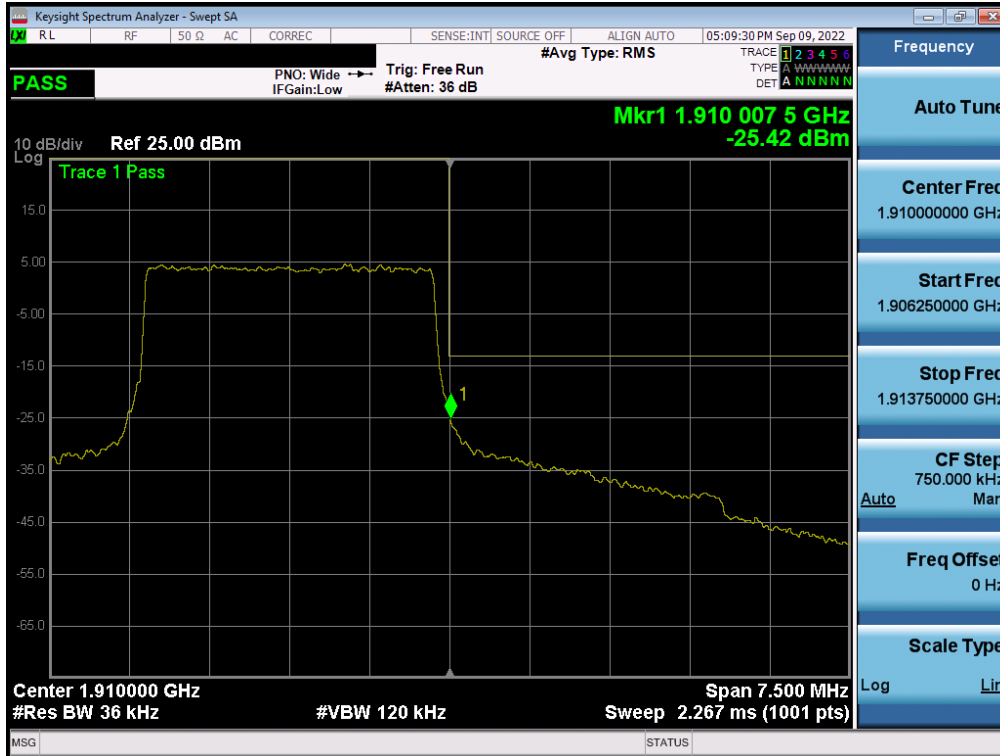
Plot 7-150. Upper Band Edge Plot (LTE Band 2 - 3MHz QPSK – Full RB - ANT A)
