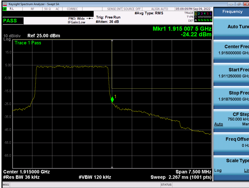
Plot 7-152. Upper Band Edge Plot (LTE Band 25 - 3MHz QPSK – Full RB - ANT A)
