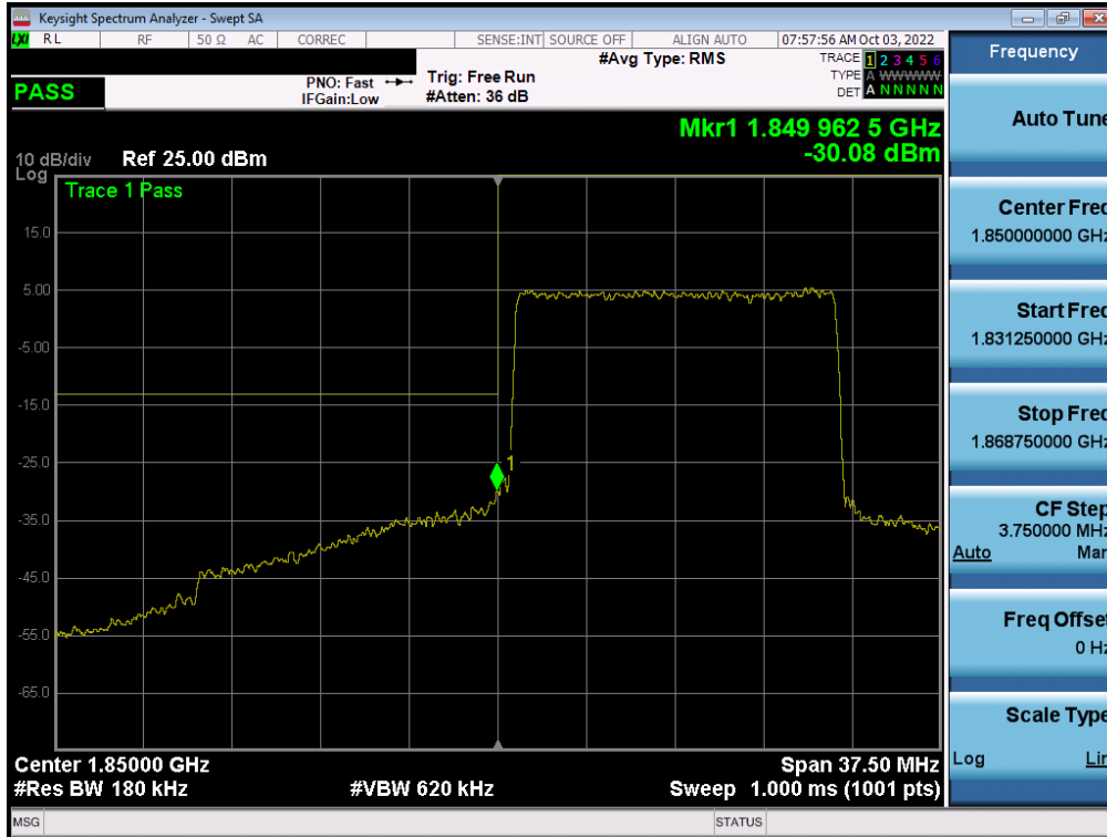
Plot 7-166. Lower Band Edge Plot (LTE Band 25/2 - 15MHz QPSK – Full RB - ANT F)
