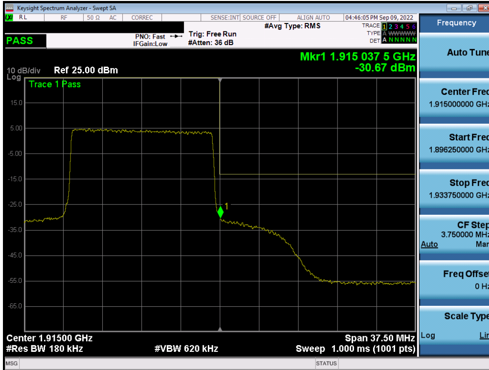
Plot 7-134. Upper Band Edge Plot (LTE Band 25 - 15MHz QPSK – Full RB - ANT A)
