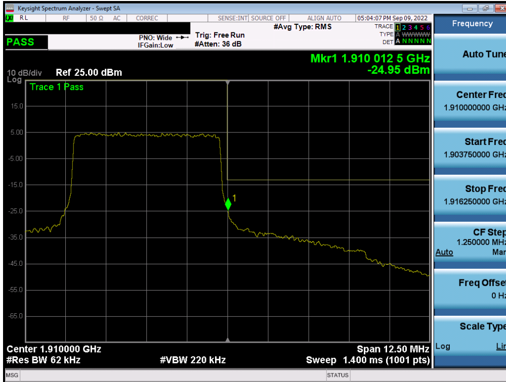
Plot 7-144. Upper Band Edge Plot (LTE Band 2 - 5MHz QPSK – Full RB - ANT A)
