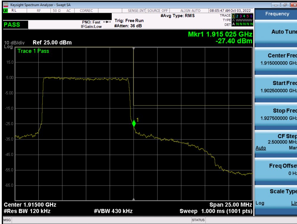
Plot 7-176. Upper Band Edge Plot (LTE Band 25 - 10MHz QPSK – Full RB - ANT F)
