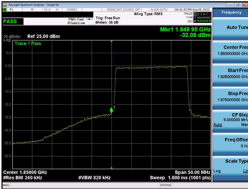
Plot 7-124. Lower Band Edge Plot (LTE Band 25/2 - 20MHz QPSK – Full RB - ANT A)
