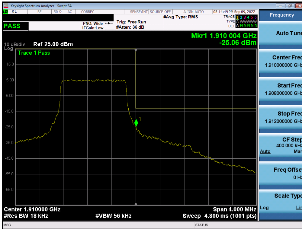
Plot 7-156. Upper Band Edge Plot (LTE Band 2 – 1.4MHz QPSK – Full RB - ANT A)
