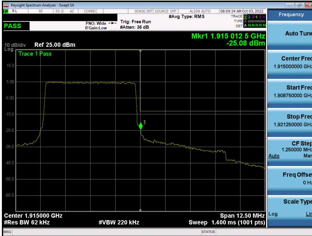
Plot 7-182. Upper Band Edge Plot (LTE Band 25 - 5MHz QPSK – Full RB - ANT F)
