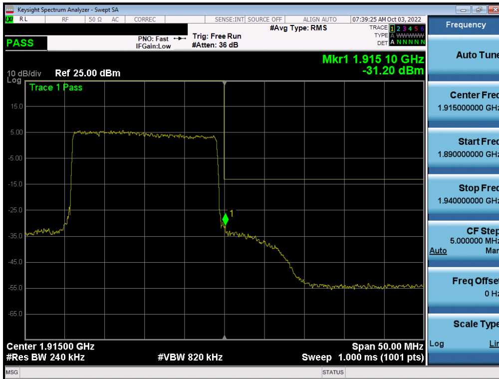
Plot 7-164. Upper Band Edge Plot (LTE Band 25 - 20MHz QPSK – Full RB - ANT F)
