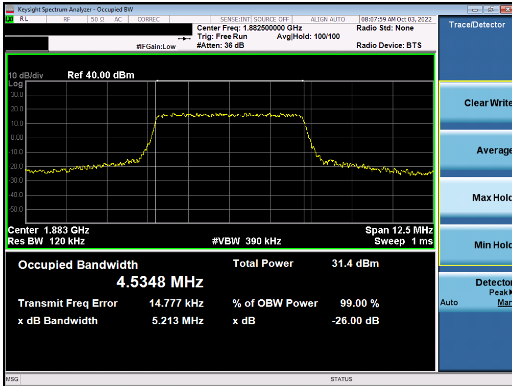
Plot 7-19. Occupied Bandwidth Plot (LTE Band 25/2 - 5MHz QPSK - Full RB - ANT F)
