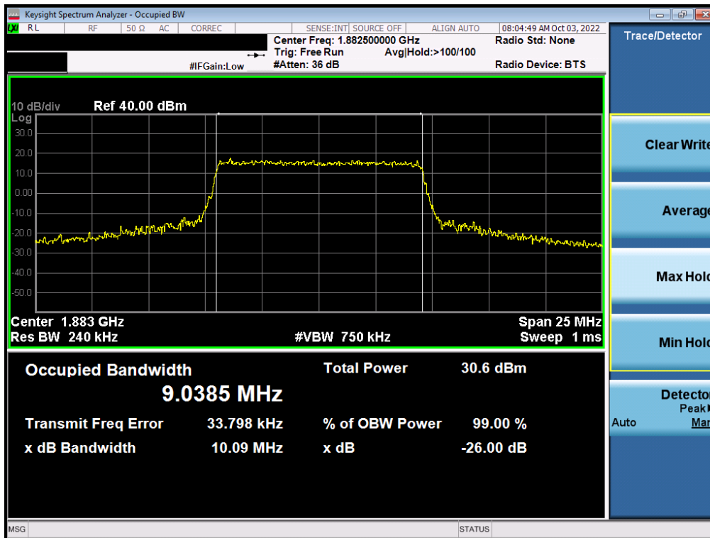
Plot 7-18. Occupied Bandwidth Plot (LTE Band 25/2 - 10MHz 16-QAM - Full RB - ANT F)
