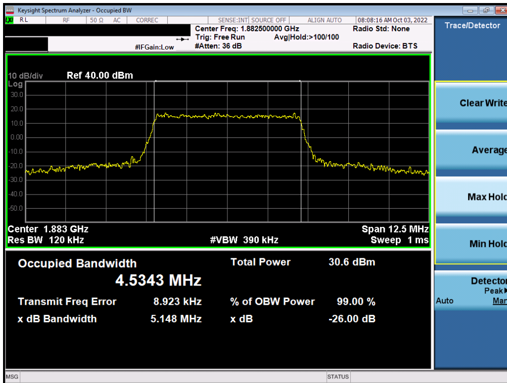
Plot 7-20. Occupied Bandwidth Plot (LTE Band 25/2 - 5MHz 16-QAM - Full RB - ANT F)
