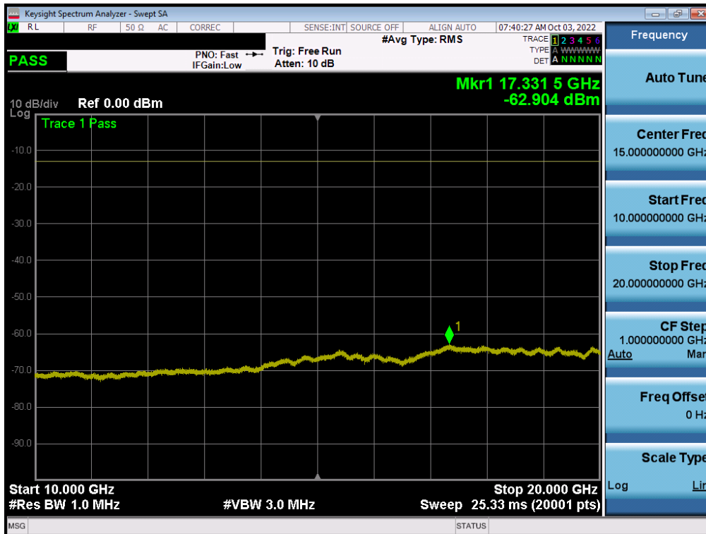
Plot 7-81. Conducted Spurious Plot (LTE Band 25/2 - 20MHz QPSK - 1RB - Low Channel - ANT F)
