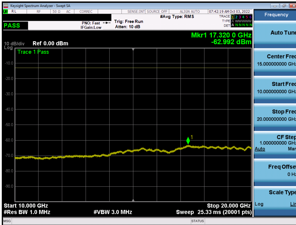
Plot 7-87. Conducted Spurious Plot (LTE Band 25/2 - 20MHz QPSK - 1RB - High Channel - ANT F)
