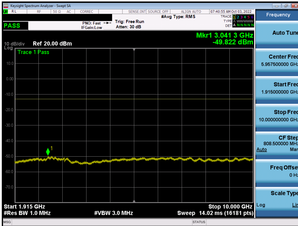
Plot 7-83. Conducted Spurious Plot (LTE Band 25/2 - 20MHz QPSK - 1RB - Mid Channel - ANT F)
