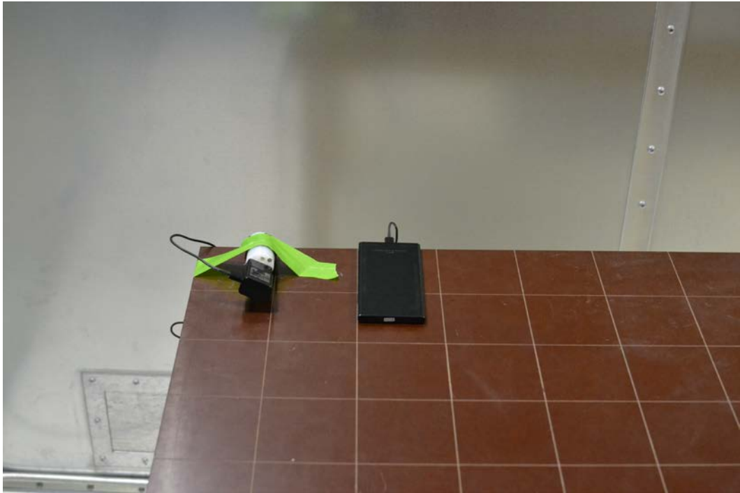
Figure 1. Test Setup – ACLC– <30MHz
