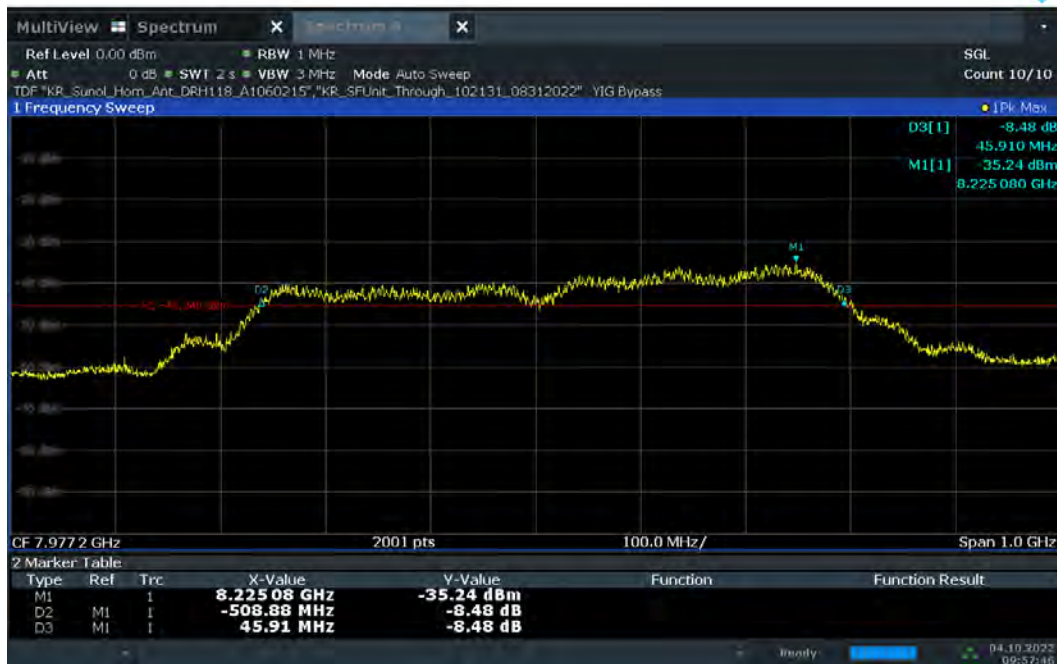
Plot 7-24. 10dBc Bandwidth – CH.9 – SP3 – Preamble 11
