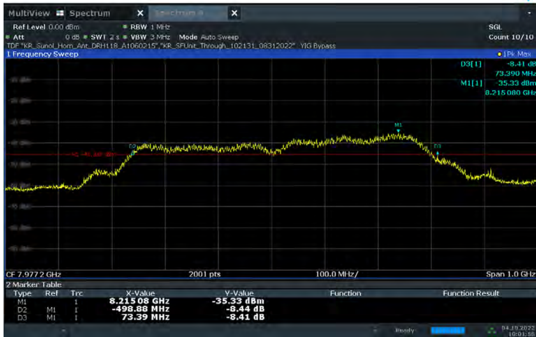
Plot 7-27. 10dBc Bandwidth – CH.9 – SP3 – Preamble 12
