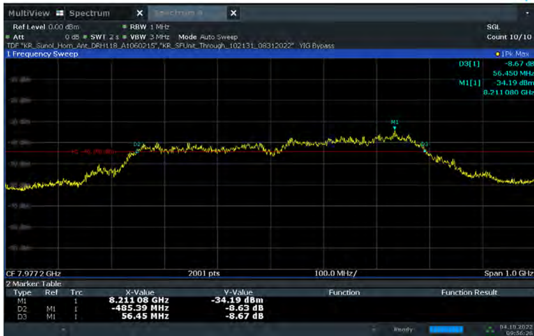
Plot 7-23. 10dBc Bandwidth – CH.9 – SP1 – Preamble 11
