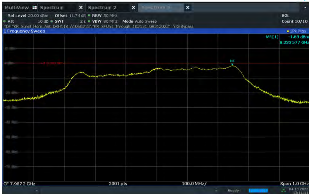
Plot 7-63. UWB Peak Power Measurement - ANT 1 - CH.9 – BPRF
