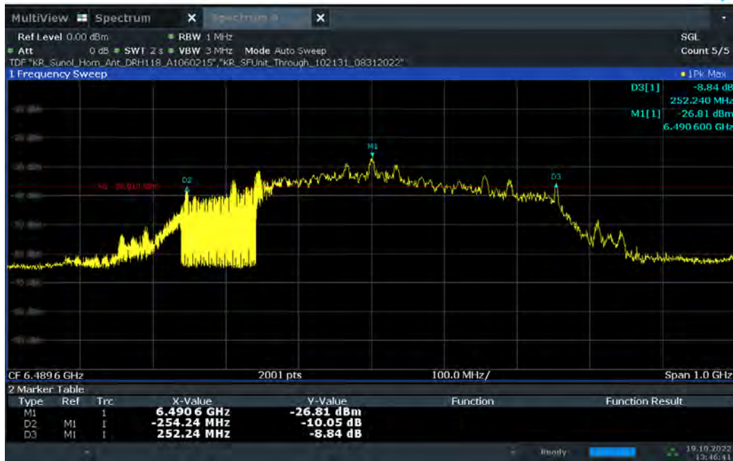
Plot 7-35. 10dBc Bandwidth – CH.5 – SP1 – Preamble 10
