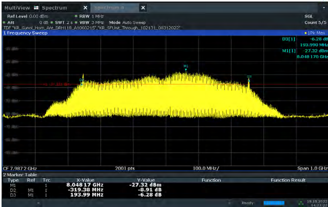
Plot 7-54. 10dBc Bandwidth – CH.9 – SP3 – Preamble 11
