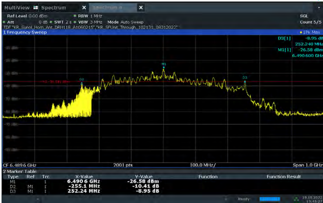
Plot 7-34. 10dBc Bandwidth – CH.5 - SP0 – Preamble 10
