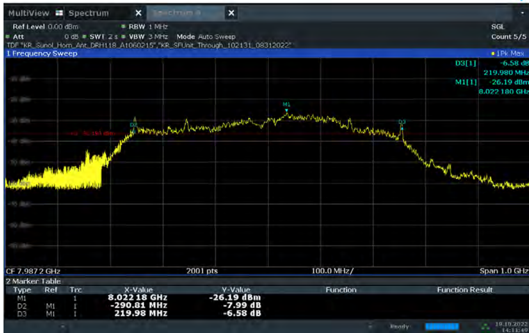
Plot 7-47. 10dBc Bandwidth – CH.9 – SP1 – Preamble 9
