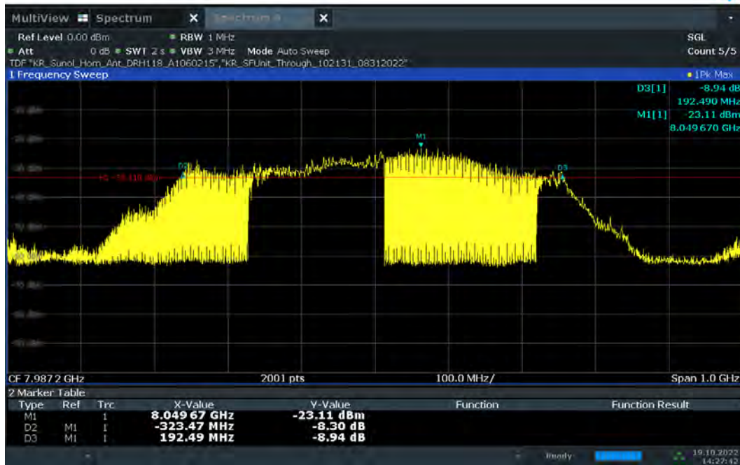
Plot 7-59. 10dBc Bandwidth – CH.9 – SP1 – Preamble 27
