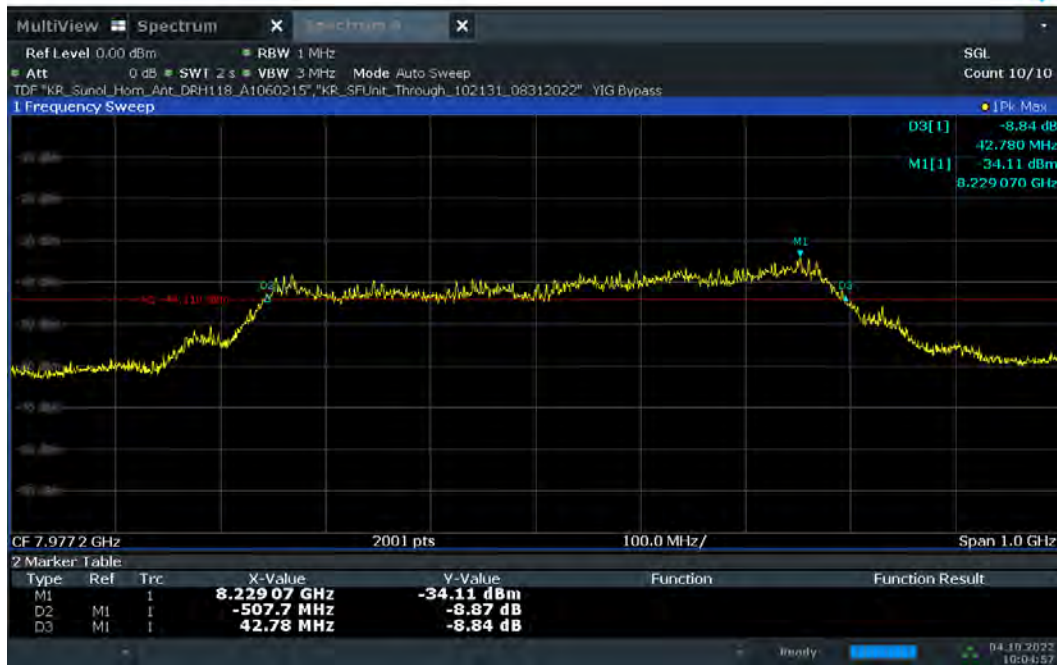
Plot 7-29. 10dBc Bandwidth – CH.9 – SP1 – Preamble 27
