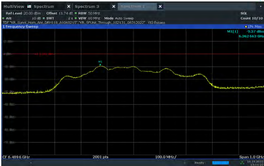
Plot 7-72. UWB Peak Power Measurement - ANT 2 - CH.5 – HPRF
