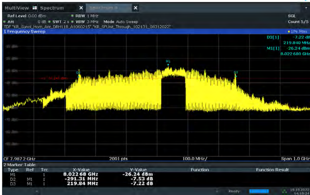
Plot 7-46. 10dBc Bandwidth – CH.9 - SP0 – Preamble 9
