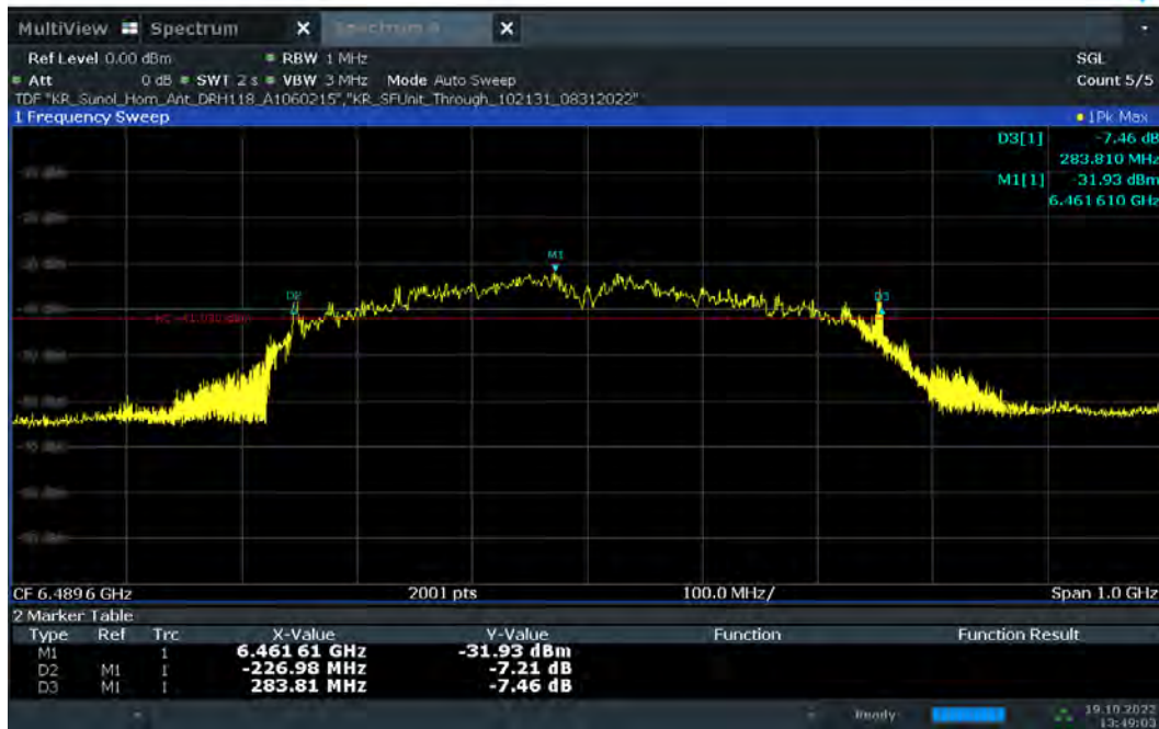
Plot 7-37. 10dBc Bandwidth – CH.5 - SP0 – Preamble 11
