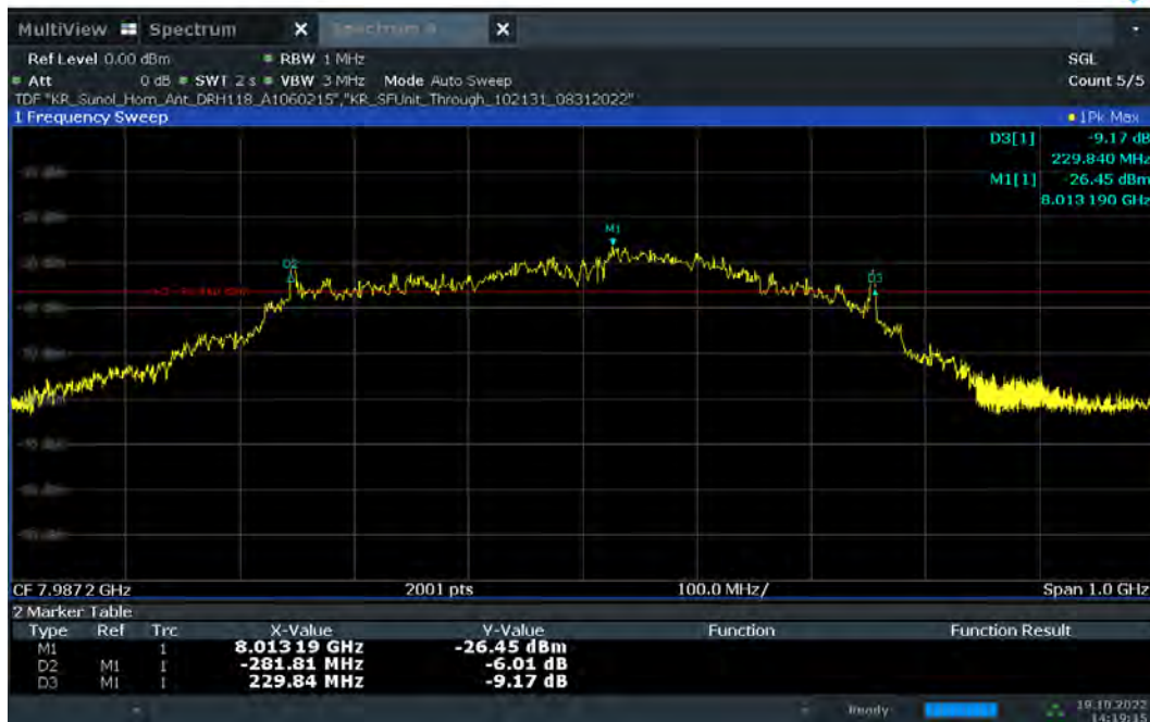
Plot 7-52. 10dBc Bandwidth – CH.9 - SP0 – Preamble 11
