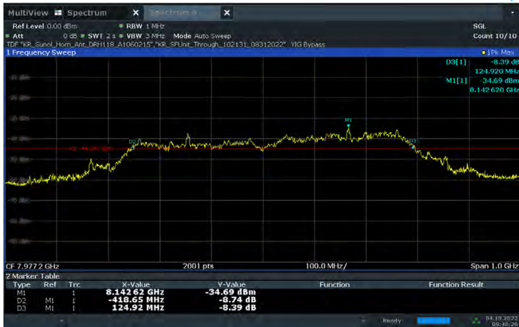
Plot 7-17. 10dBc Bandwidth – CH.9 – SP1 – Preamble 9
