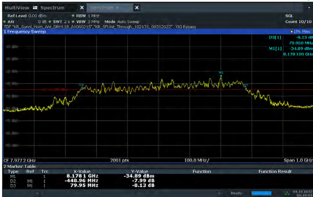
Plot 7-19. 10dBc Bandwidth – CH.9 - SP0 – Preamble 10
