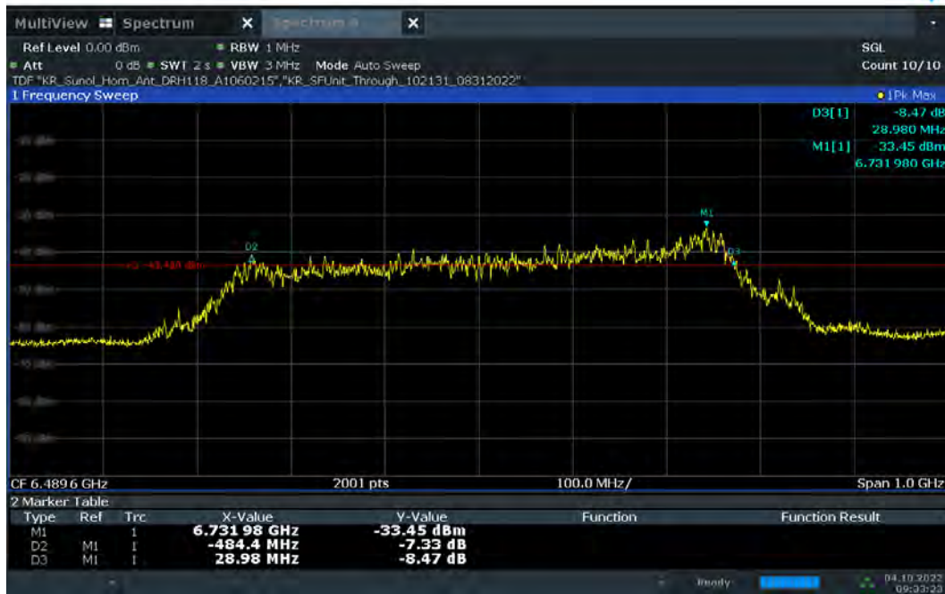
Plot 7-13. 10dBc Bandwidth – CH.5 - SP0 – Preamble 27
