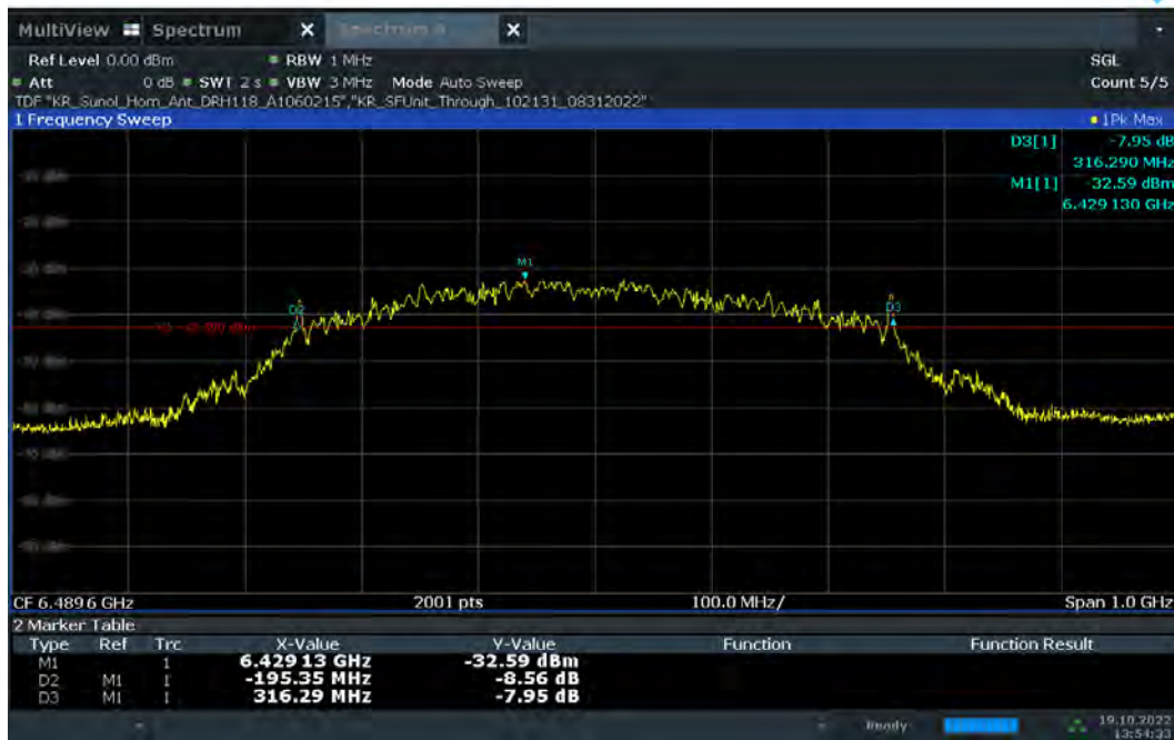
Plot 7-40. 10dBc Bandwidth – CH.5 - SP0 – Preamble 12
