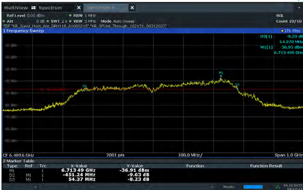
Plot 7-8. 10dBc Bandwidth – CH.5 – SP1 – Preamble 11
