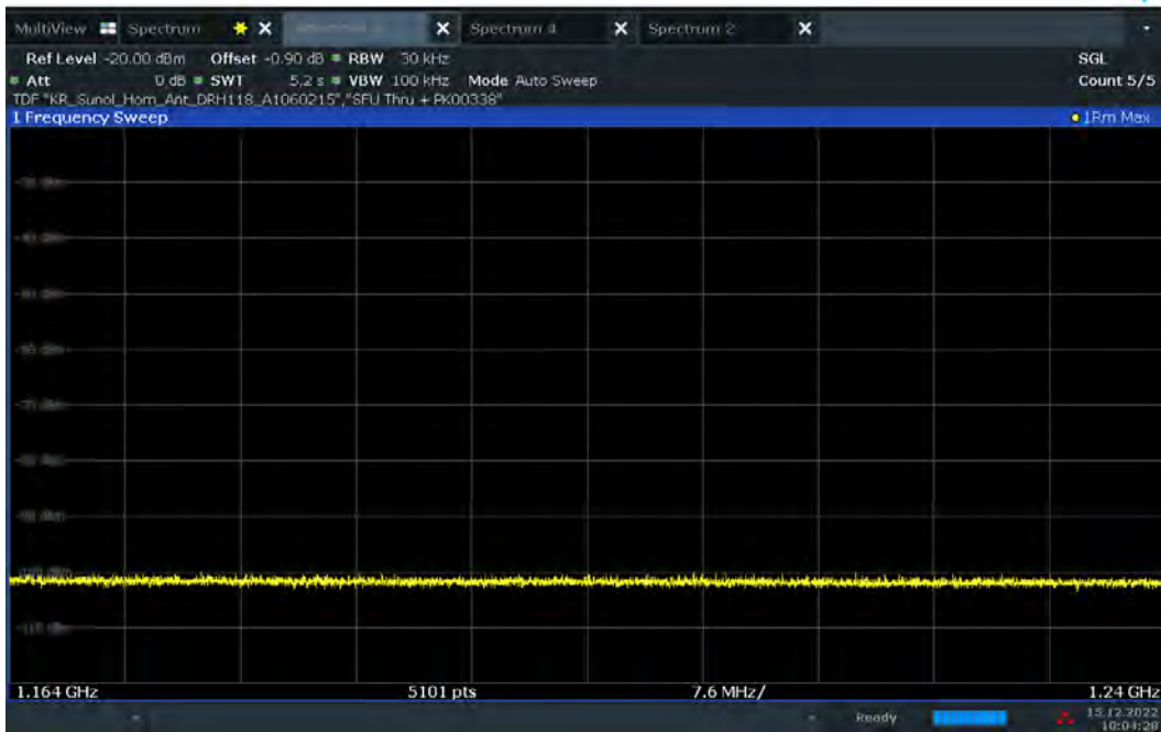
Plot 7-85. Radiated Spurious Pre-Scan 1164 - 1240 MHz - CH.5 - ANT 2 – GPS band
