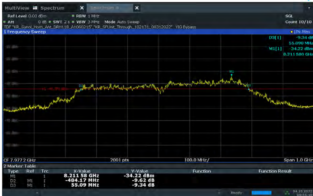
Plot 7-22. 10dBc Bandwidth – CH.9 - SP0 – Preamble 11
