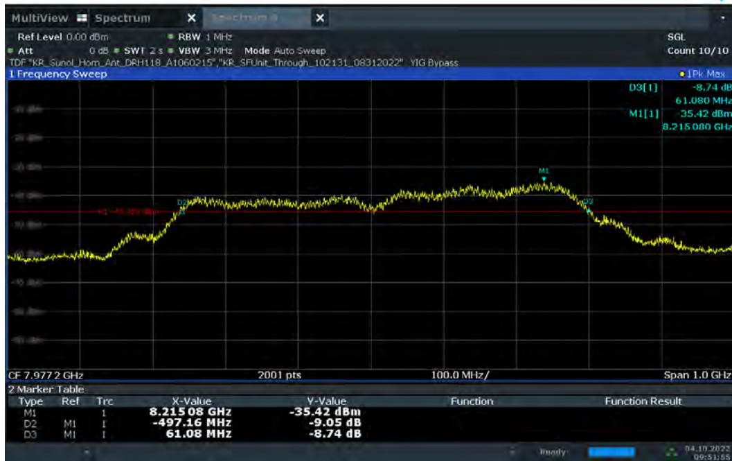
Plot 7-21. 10dBc Bandwidth – CH.9 – SP3 – Preamble 10
