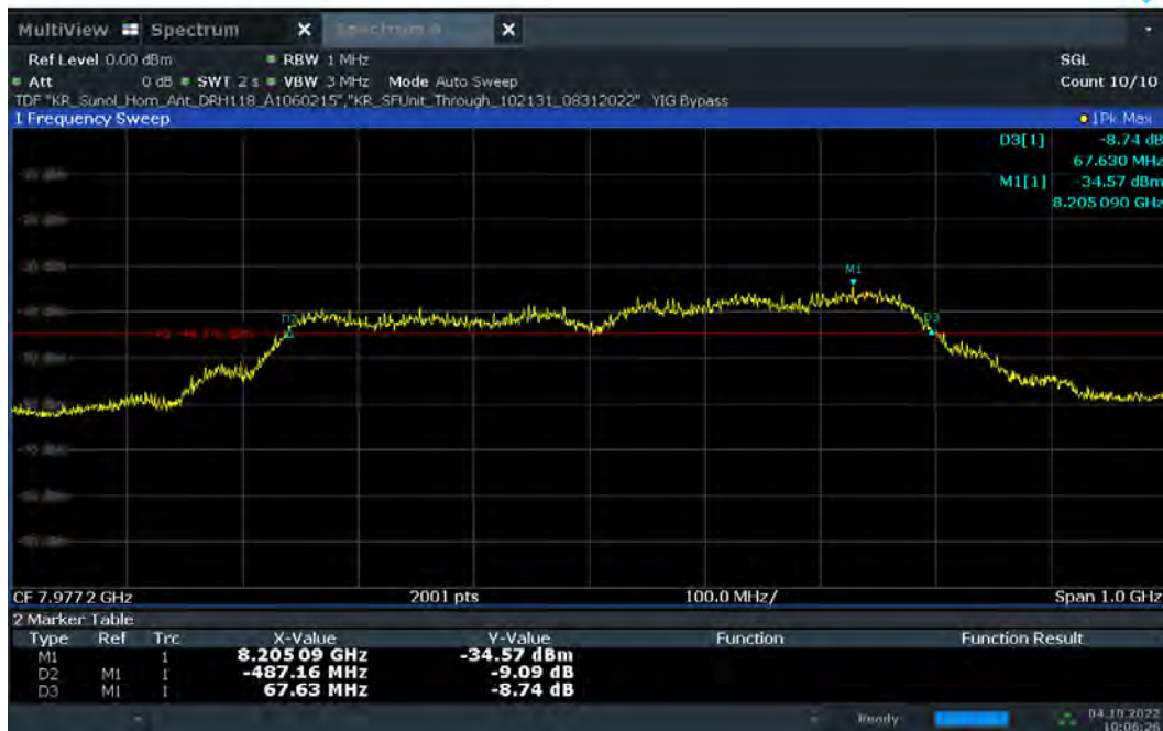
Plot 7-30. 10dBc Bandwidth – CH.9 – SP3 – Preamble 27
