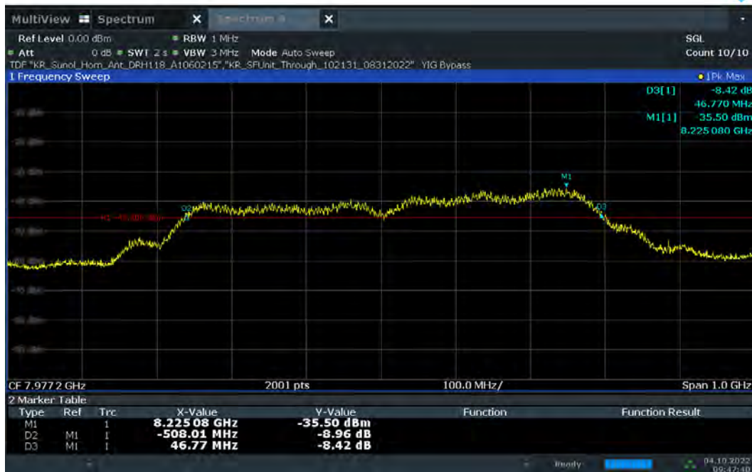
Plot 7-18. 10dBc Bandwidth – CH.9 – SP3 – Preamble 9
