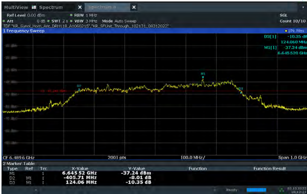
Plot 7-2. 10dBc Bandwidth – CH.5 – SP1 – Preamble 9
