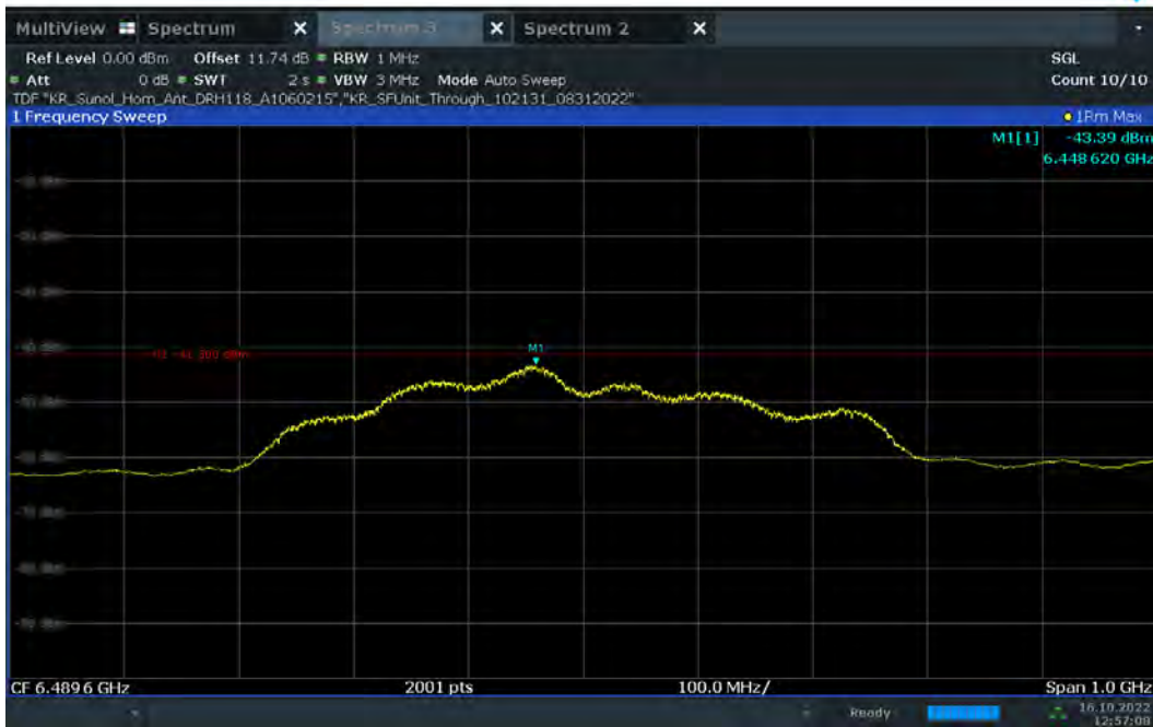
Plot 7-76. UWB Average Power Measurement - ANT 2 - CH.5 – HPRF
