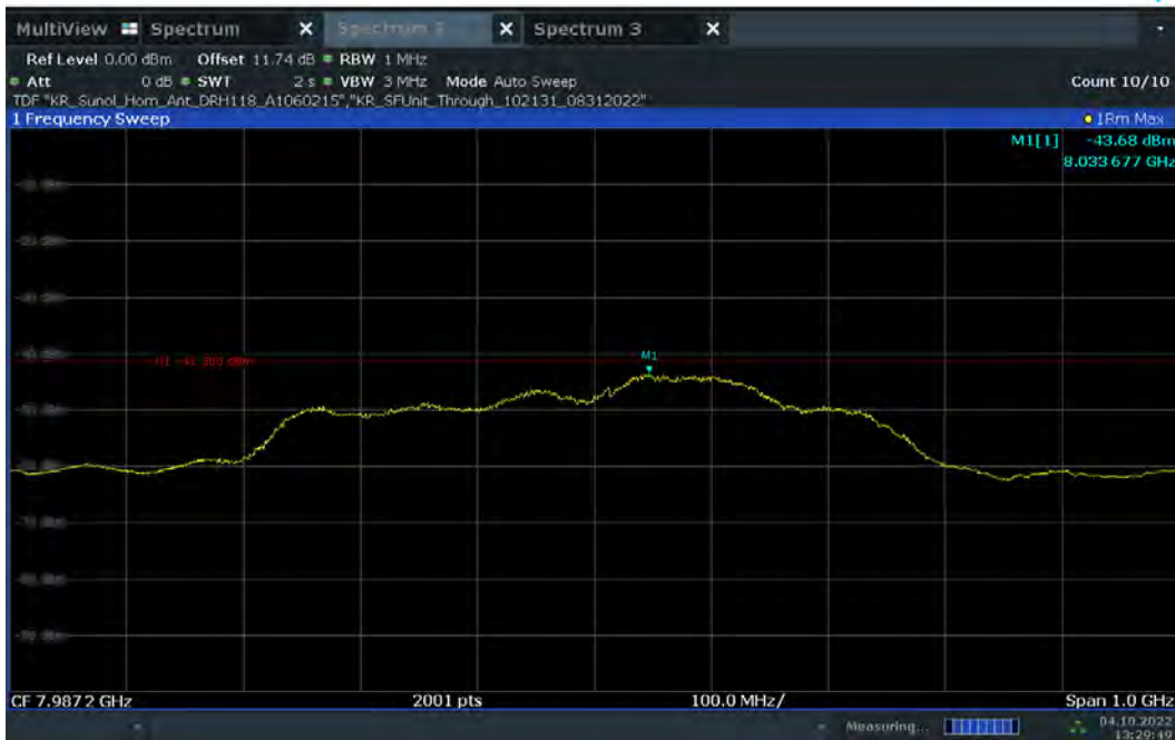
Plot 7-69. UWB Average Power Measurement - ANT 2 - CH.9 – BPRF
