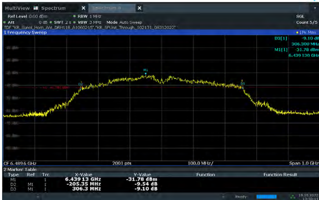
Plot 7-38. 10dBc Bandwidth – CH.5 – SP1 – Preamble 11
