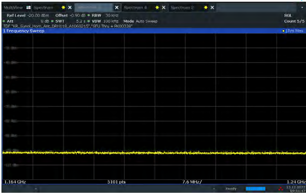
Plot 7-80. Radiated Spurious Pre-Scan 1164 - 1240 MHz - CH.5 - ANT 1 – GPS band
