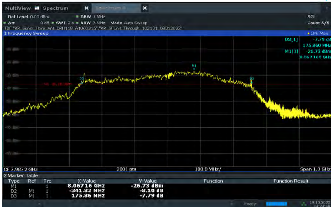
Plot 7-56. 10dBc Bandwidth – CH.9 – SP1 – Preamble 12
