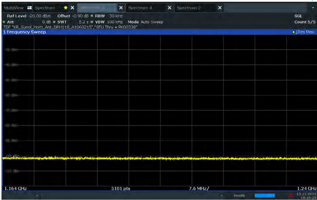
Plot 7-95. Radiated Spurious Pre-Scan 1164 - 1240 MHz - CH.9 - ANT 2 – GPS band
