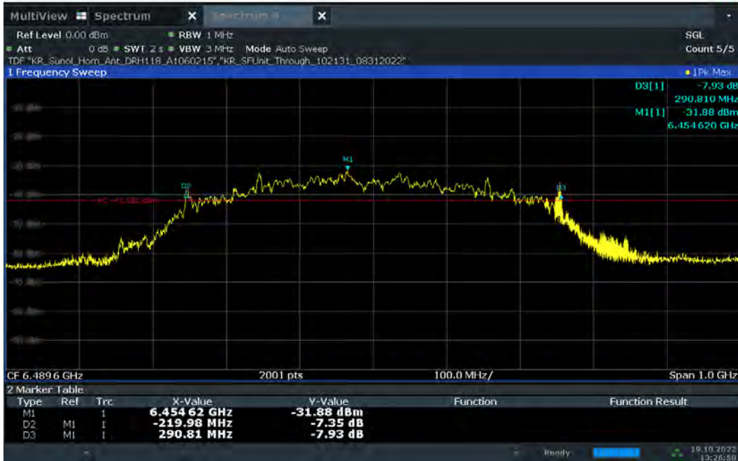
Plot 7-31. 10dBc Bandwidth – CH.5 - SP0 – Preamble 9
