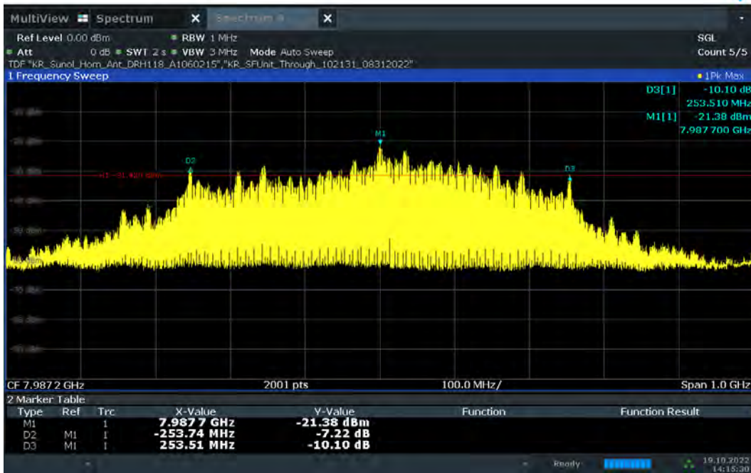
Plot 7-49. 10dBc Bandwidth – CH.9 - SP0 – Preamble 10
