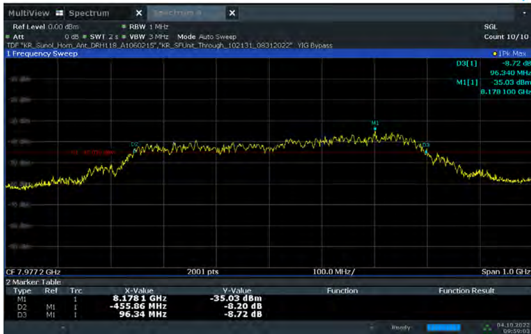
Plot 7-25. 10dBc Bandwidth – CH.9 - SP0 – Preamble 12
