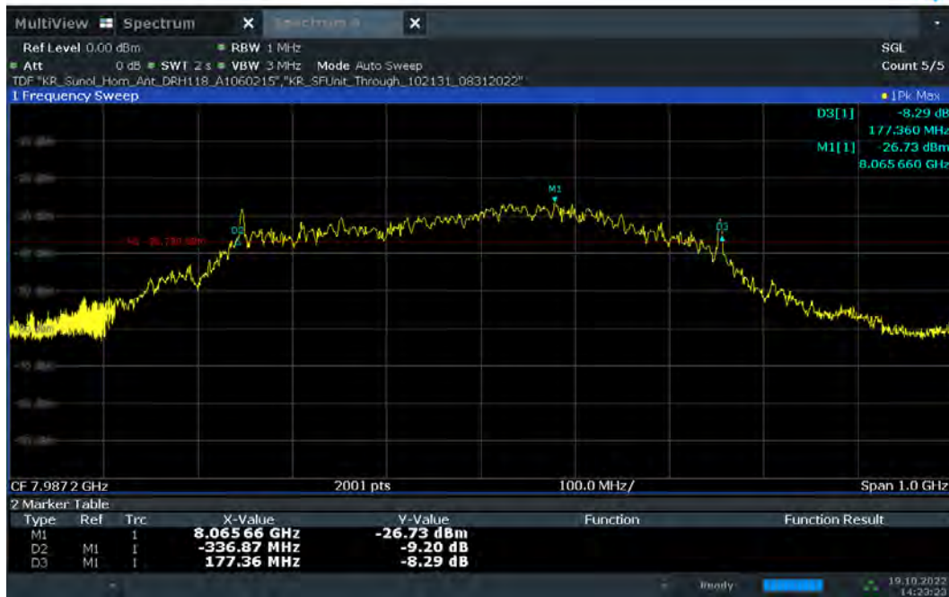
Plot 7-55. 10dBc Bandwidth – CH.9 - SP0 – Preamble 12
