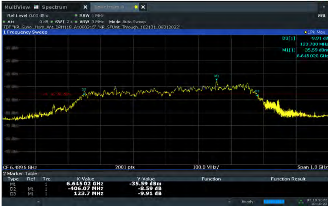
Plot 7-1. 10dBc Bandwidth – CH.5 - SP0 – Preamble 9
