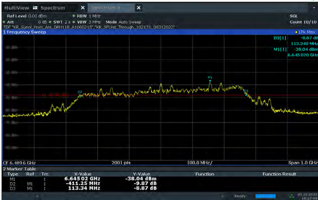
Plot 7-5. 10dBc Bandwidth – CH.5 – SP1 – Preamble 10
