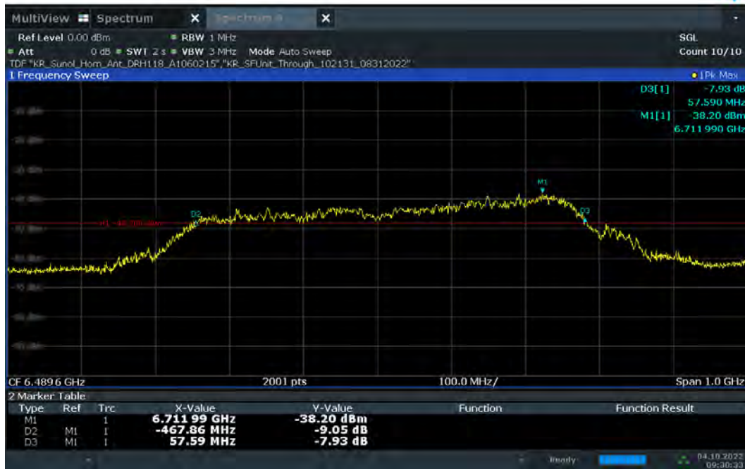
Plot 7-11. 10dBc Bandwidth – CH.5 – SP1 – Preamble 12
