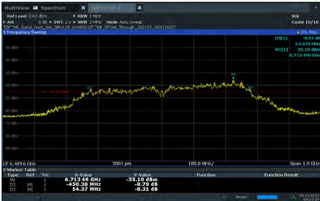
Plot 7-7. 10dBc Bandwidth – CH.5 - SP0 – Preamble 11
