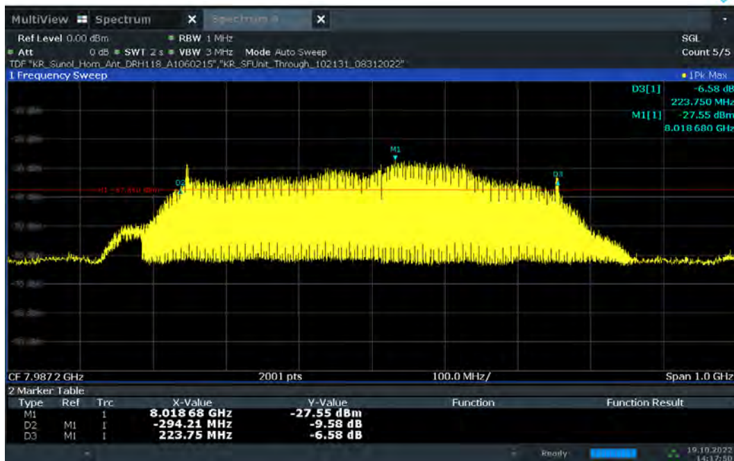
Plot 7-51. 10dBc Bandwidth – CH.9 – SP3 – Preamble 10
