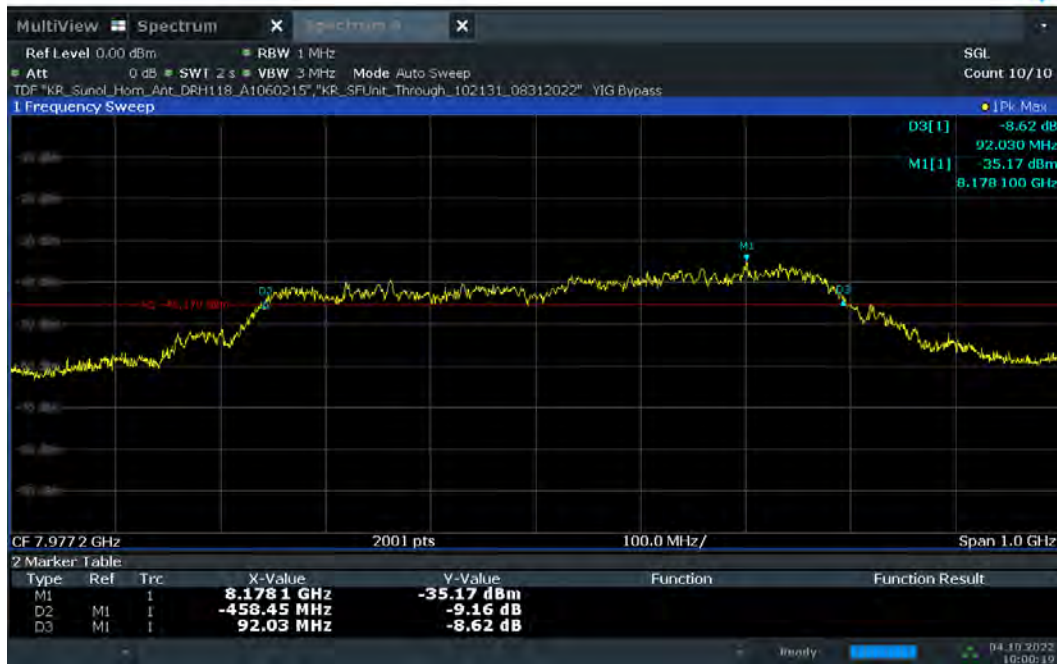
Plot 7-26. 10dBc Bandwidth – CH.9 – SP1 – Preamble 12
