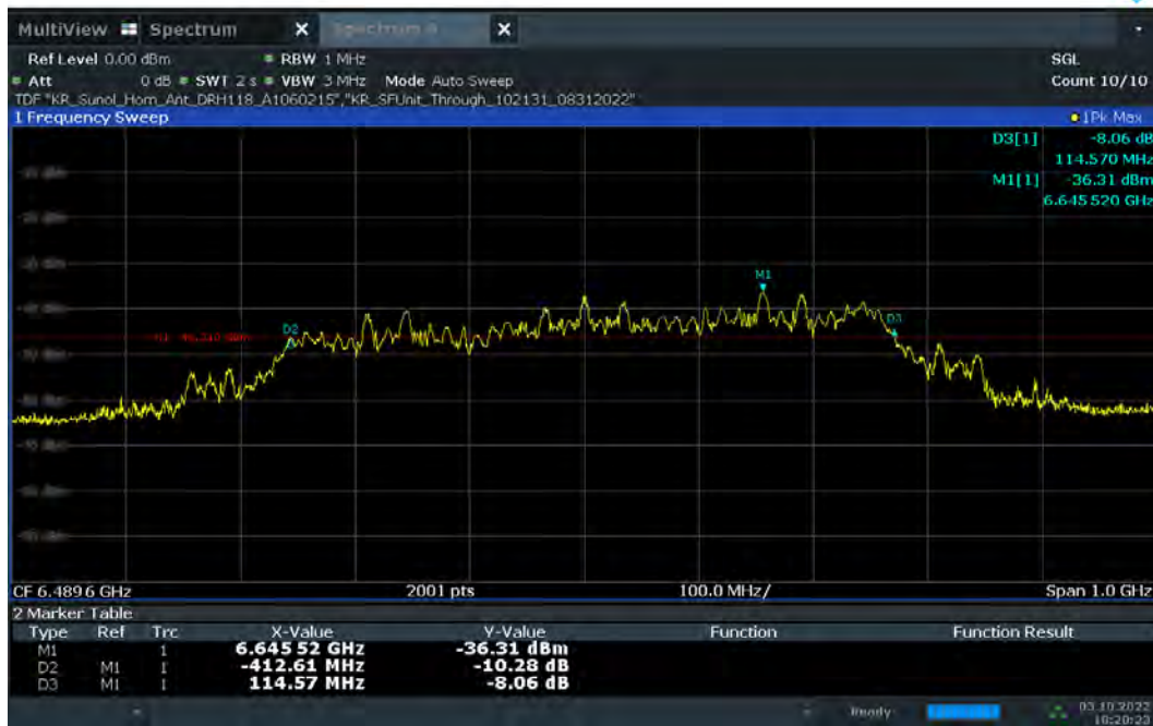
Plot 7-4. 10dBc Bandwidth – CH.5 - SP0 – Preamble 10
