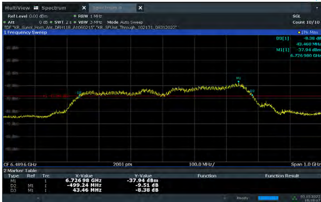
Plot 7-3. 10dBc Bandwidth – CH.5 – SP3 – Preamble 9
