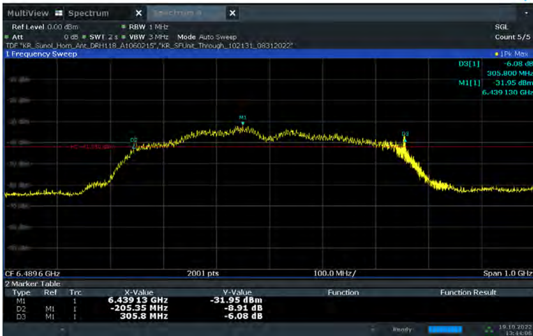
Plot 7-33. 10dBc Bandwidth – CH.5 – SP3 – Preamble 9
