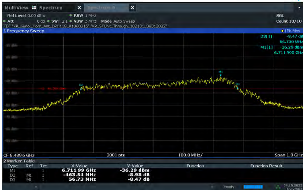
Plot 7-10. 10dBc Bandwidth – CH.5 - SP0 – Preamble 12
