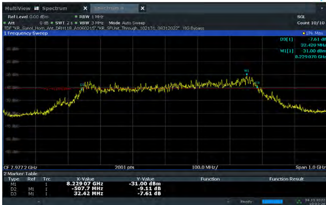
Plot 7-28. 10dBc Bandwidth – CH.9 - SP0 – Preamble 27
