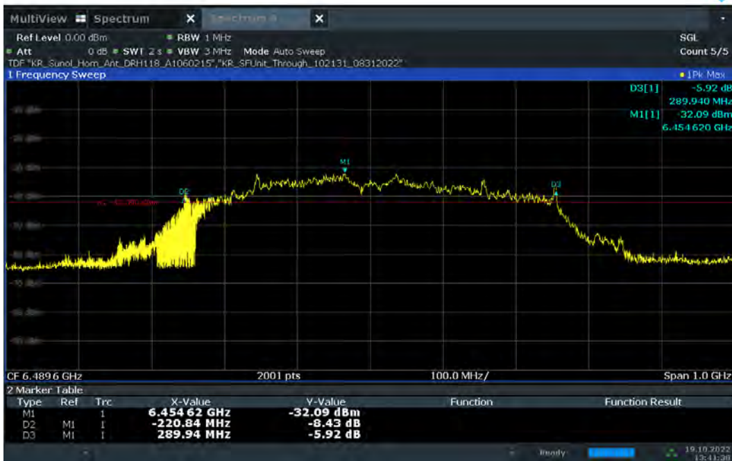
Plot 7-32. 10dBc Bandwidth – CH.5 – SP1 – Preamble 9
