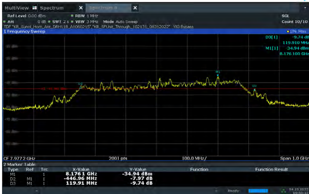
Plot 7-20. 10dBc Bandwidth – CH.9 – SP1 – Preamble 10
