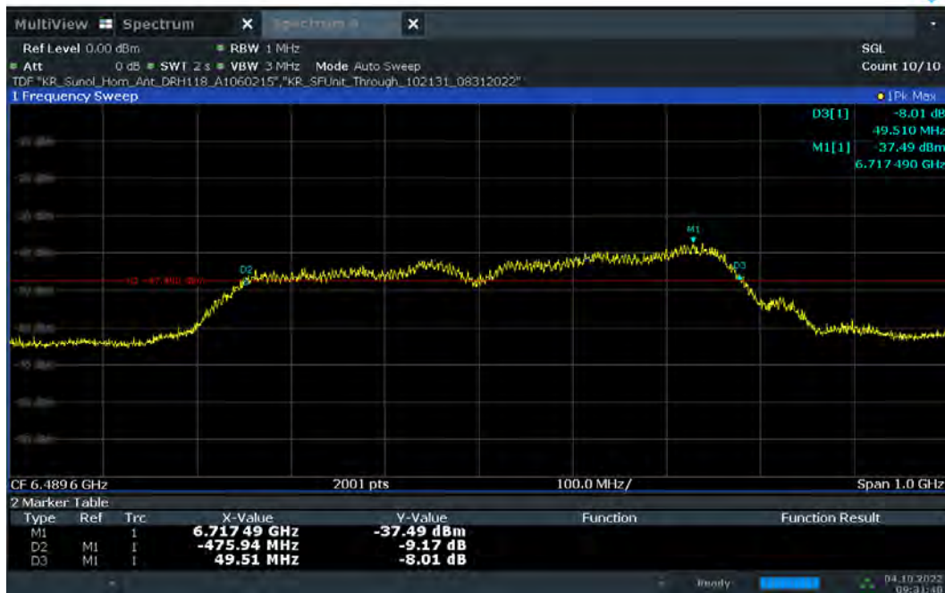
Plot 7-12. 10dBc Bandwidth – CH.5 – SP3 – Preamble 12
