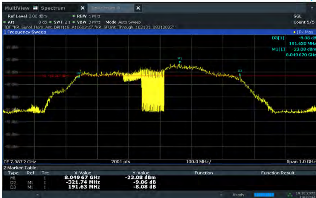
Plot 7-60. 10dBc Bandwidth – CH.9 – SP3 – Preamble 27
