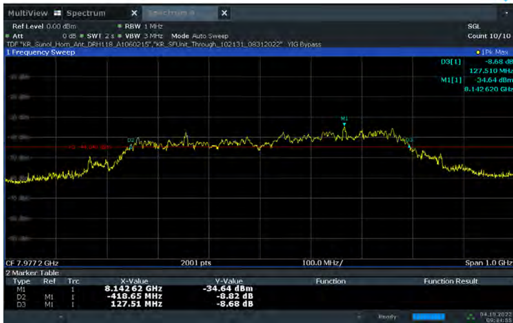
Plot 7-16. 10dBc Bandwidth – CH.9 - SP0 – Preamble 9
