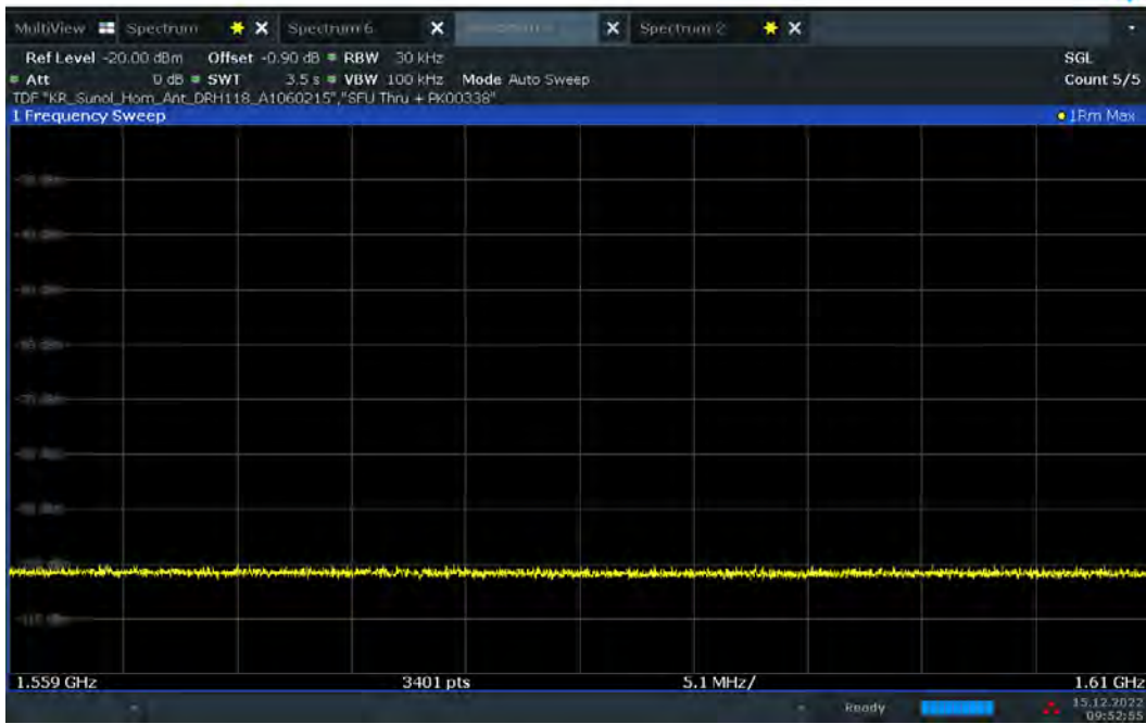
Plot 7-81. Radiated Spurious Pre-Scan 1559 - 1610 MHz - CH.5 - ANT 1 – GPS band
