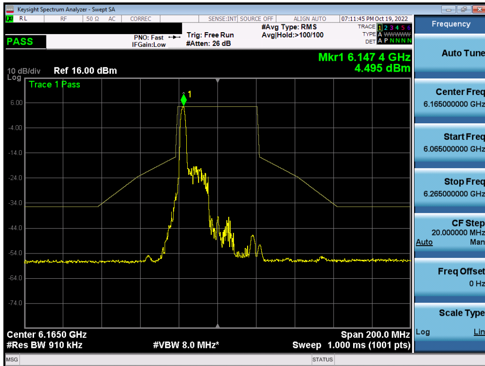
Plot 7-572. In-Band Emission Plot MIMO ANT2 (40MHz BW 802.11ax (26 Tones) (UNII Band 5) – Ch. 43) - SP
