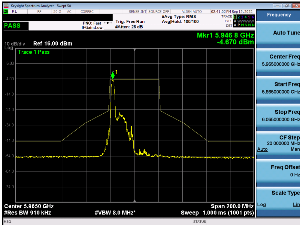
Plot 7-531. In-Band Emission Plot MIMO ANT2 (40MHz BW 802.11ax (26 Tones) (UNII Band 5) – Ch. 3) – LPI
