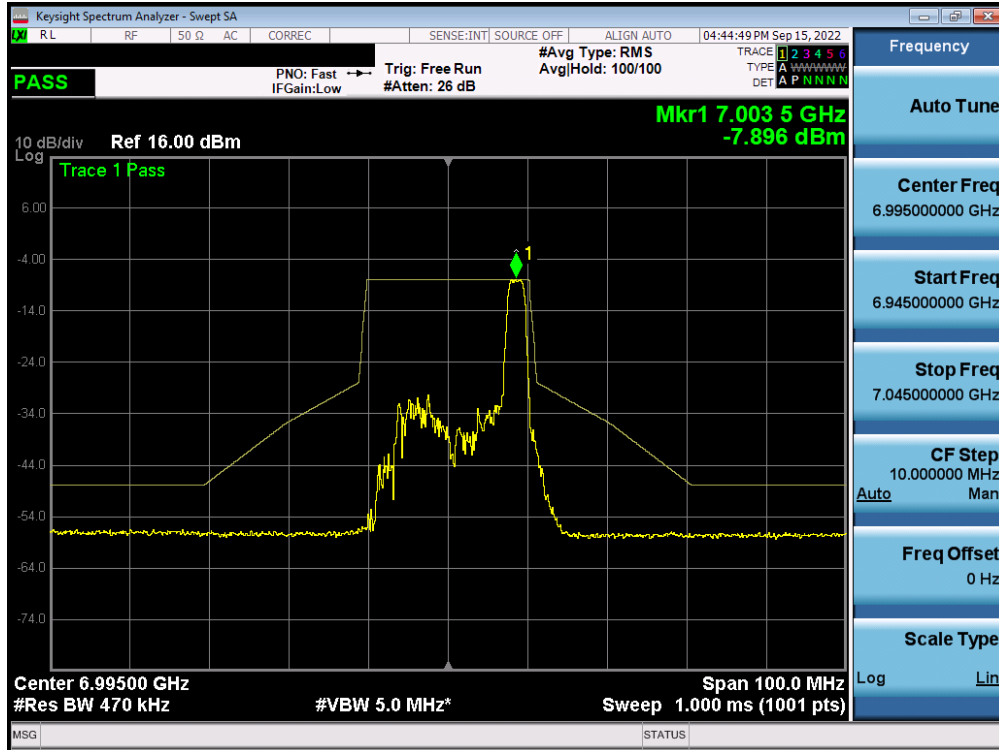
Plot 7-457. In-Band Emission Plot MIMO ANT1 (20MHz BW 802.11ax (26 Tones) (UNII Band 8) – Ch. 209) – LPI
