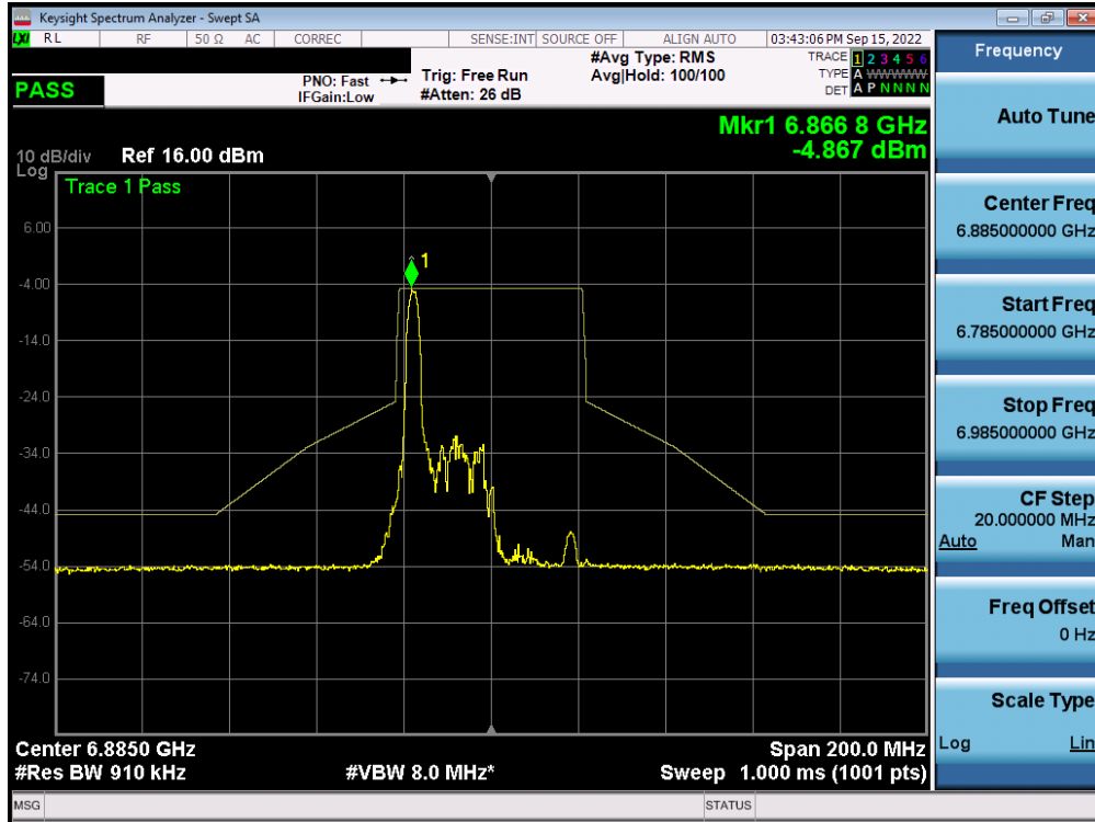
Plot 7-562. In-Band Emission Plot MIMO ANT2 (40MHz BW 802.11ax (26 Tones) (UNII Band 8) – Ch. 187) – LPI
