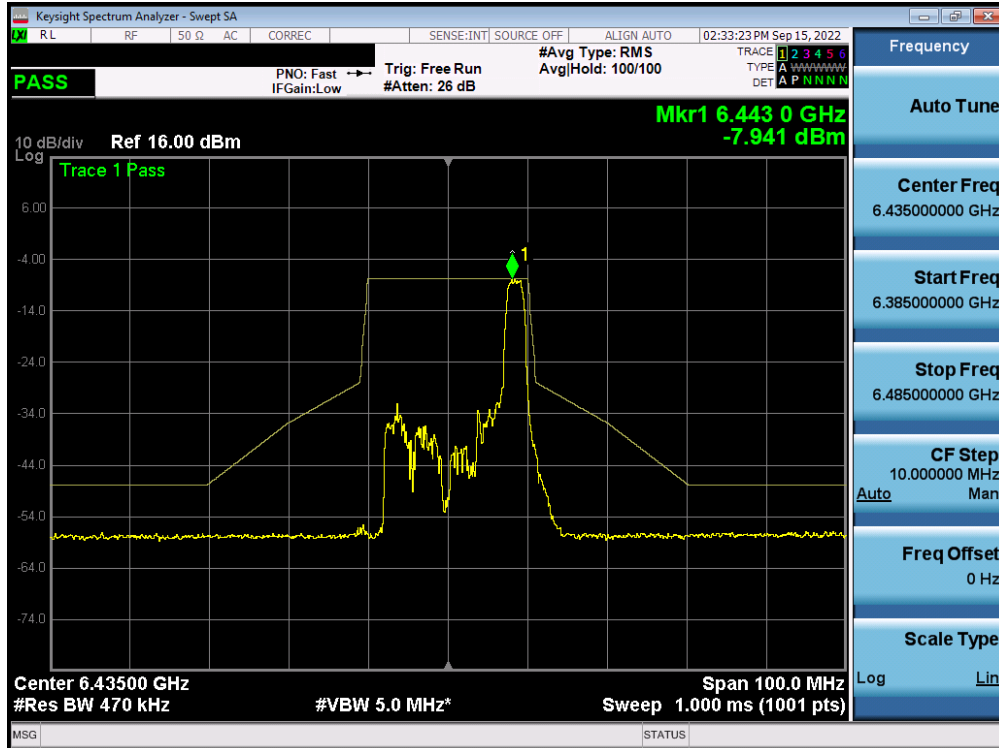
Plot 7-540. In-Band Emission Plot MIMO ANT2 (20MHz BW 802.11ax (26 Tones) (UNII Band 6) – Ch. 97) – LPI
