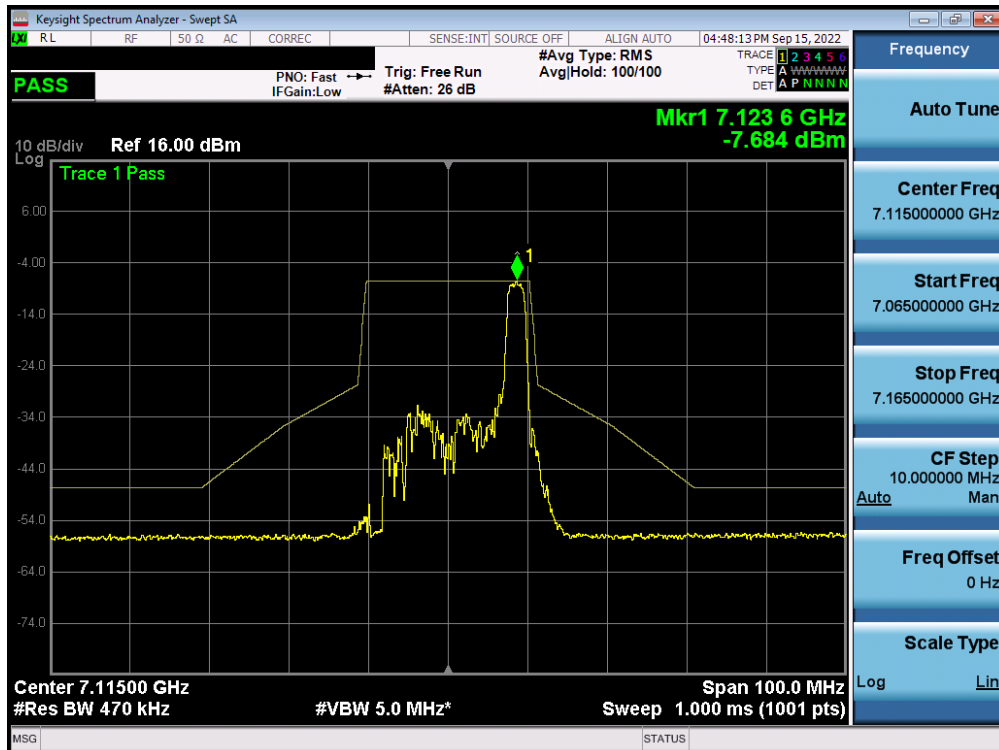
Plot 7-458. In-Band Emission Plot MIMO ANT1 (20MHz BW 802.11ax (26 Tones) (UNII Band 8) – Ch. 233) – LPI
