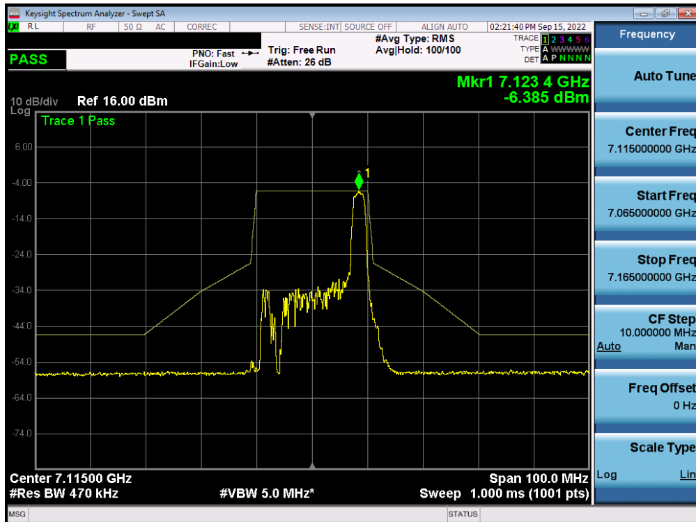
Plot 7-561. In-Band Emission Plot MIMO ANT2 (20MHz BW 802.11ax (26 Tones) (UNII Band 8) – Ch. 233) – LPI
