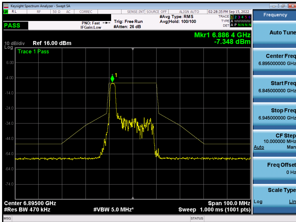
Plot 7-559. In-Band Emission Plot MIMO ANT2 (20MHz BW 802.11ax (26 Tones) (UNII Band 8) – Ch. 189) – LPI
