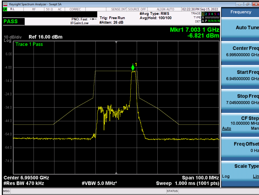
Plot 7-560. In-Band Emission Plot MIMO ANT2 (20MHz BW 802.11ax (26 Tones) (UNII Band 8) – Ch. 209) – LPI
