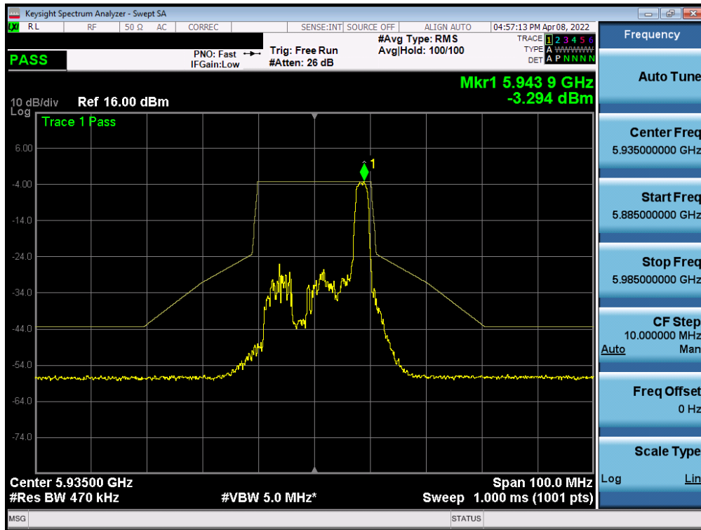
Plot 7-528. In-Band Emission Plot MIMO ANT2 (20MHz BW 802.11ax (26 Tones) UNII Band 5) – Ch. 2) – LPI
