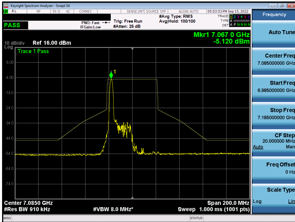
Plot 7-461. In-Band Emission Plot MIMO ANT1 (40MHz BW 802.11ax (26 Tones) (UNII Band 8) – Ch. 227) – LPI
