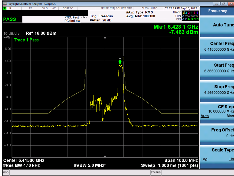
Plot 7-530. In-Band Emission Plot MIMO ANT2 (20MHz BW 802.11ax (26 Tones) UNII Band 5) – Ch. 93) – LPI
