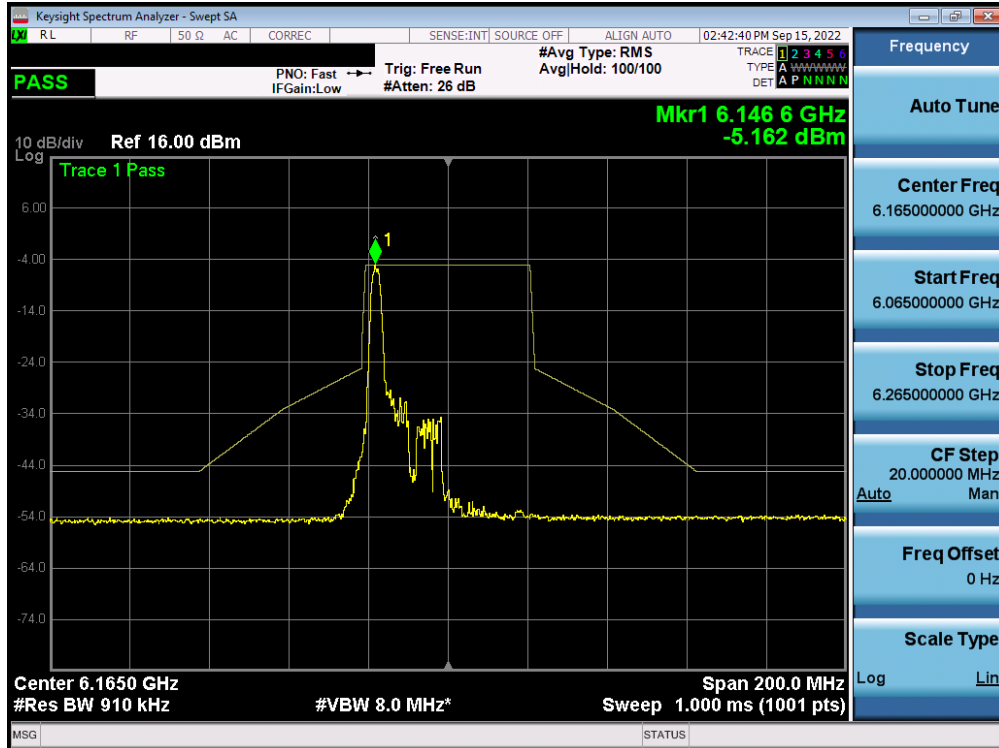
Plot 7-532. In-Band Emission Plot MIMO ANT2 (40MHz BW 802.11ax (26 Tones) (UNII Band 5) – Ch. 43) – LPI
