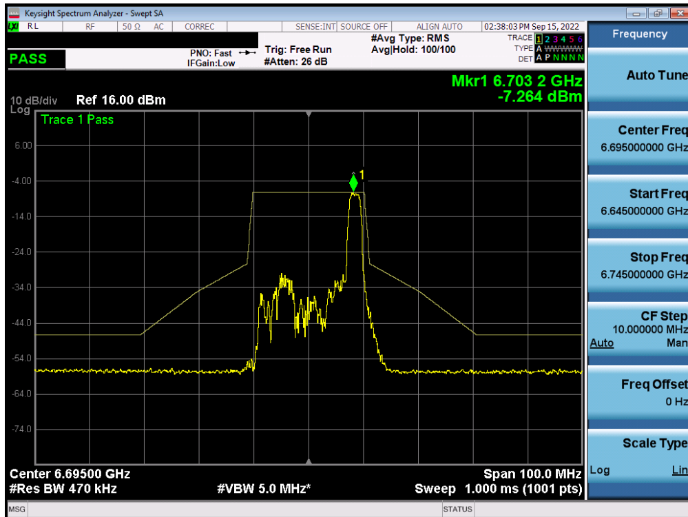
Plot 7-549. In-Band Emission Plot MIMO ANT2 (20MHz BW 802.11ax (26 Tones) (UNII Band 7) – Ch. 149) – LPI
