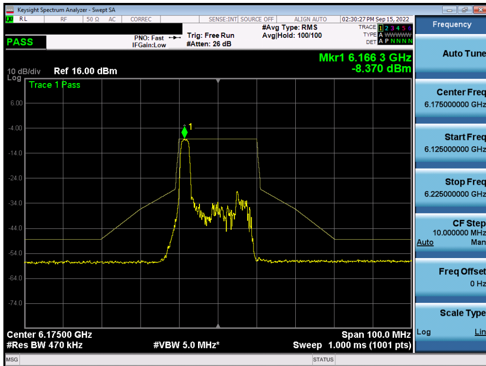
Plot 7-529. In-Band Emission Plot MIMO ANT2 (20MHz BW 802.11ax (26 Tones) (UNII Band 5) – Ch. 45) – LPI
