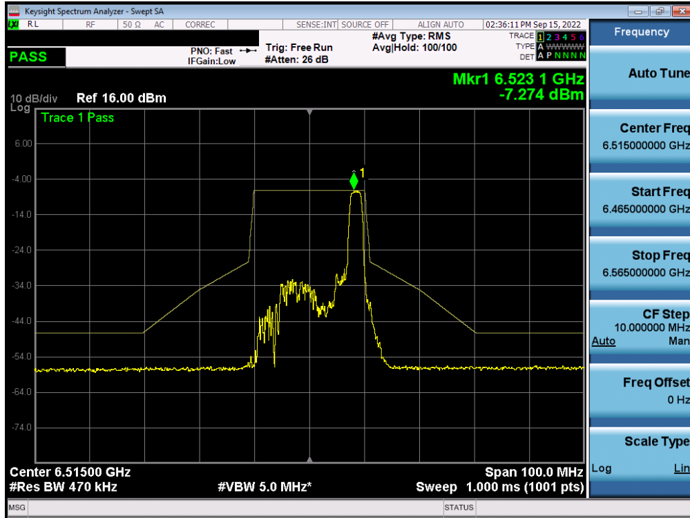
Plot 7-542. In-Band Emission Plot MIMO ANT2 (20MHz BW 802.11ax (26 Tones) (UNII Band 6) – Ch. 113) – LPI
