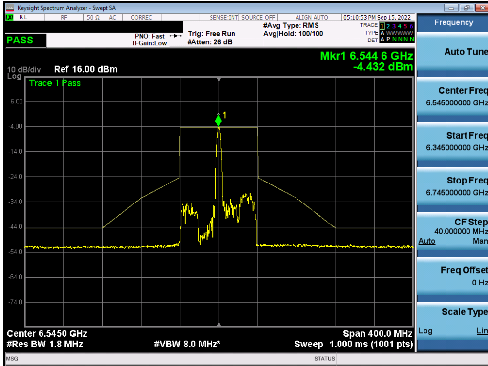
Plot 7-451. In-Band Emission Plot MIMO ANT1 (80MHz BW 802.11ax (26 Tones) (UNII Band 7) – Ch. 119) – LPI
