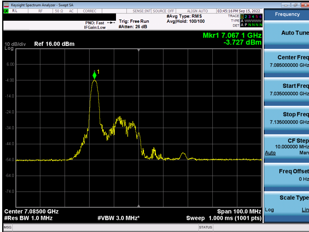
Plot 7-355. Power Spectral Density Plot MIMO ANT2 (40MHz BW 802.11ax (26 Tones) (UNII Band 8) – Ch. 227) – LPI
