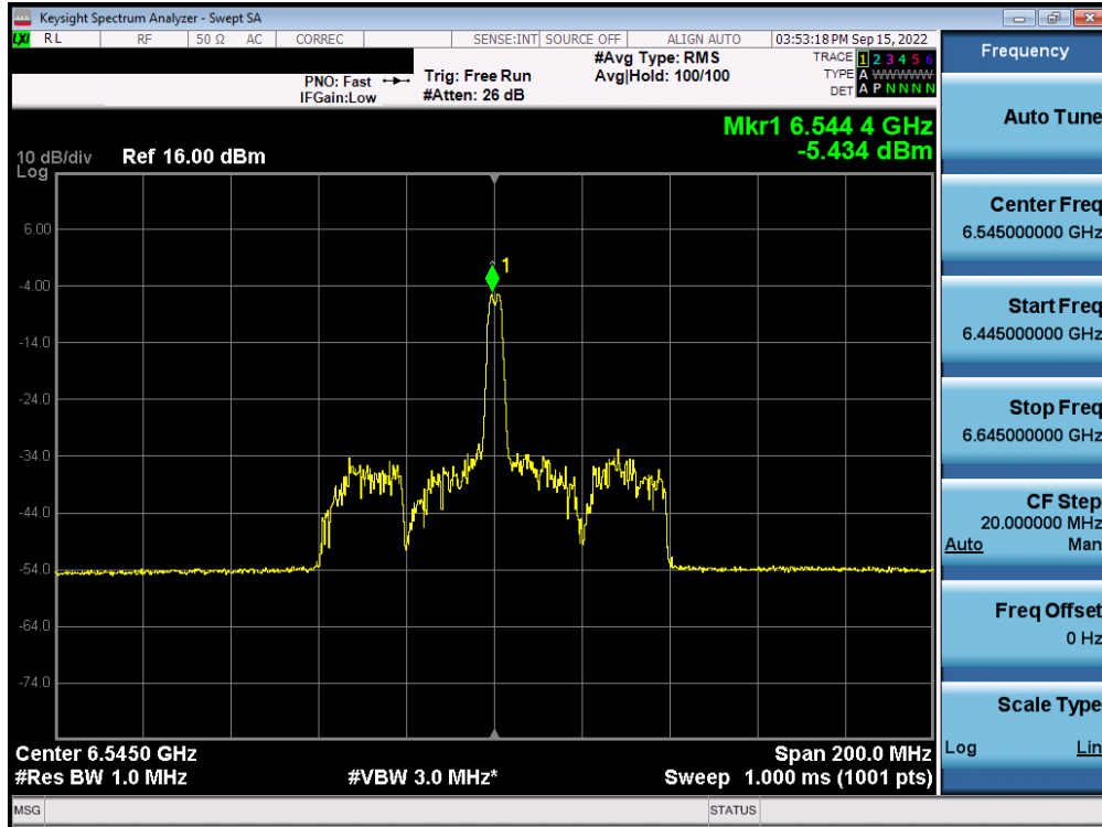
Plot 7-345. Power Spectral Density Plot MIMO ANT2 (80MHz BW 802.11ax (26 Tones) (UNII Band 7) – Ch. 119) – LPI
