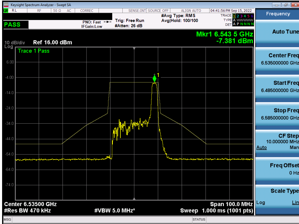
Plot 7-445. In-Band Emission Plot MIMO ANT1 (20MHz BW 802.11ax (26 Tones) (UNII Band 7) – Ch. 117) – LPI
