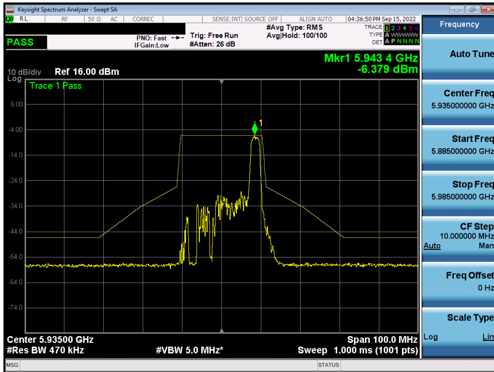
Plot 7-425. In-Band Emission Plot MIMO ANT1 (20MHz BW 802.11ax (26 Tones) UNII Band 5) – Ch. 2 – LPI
