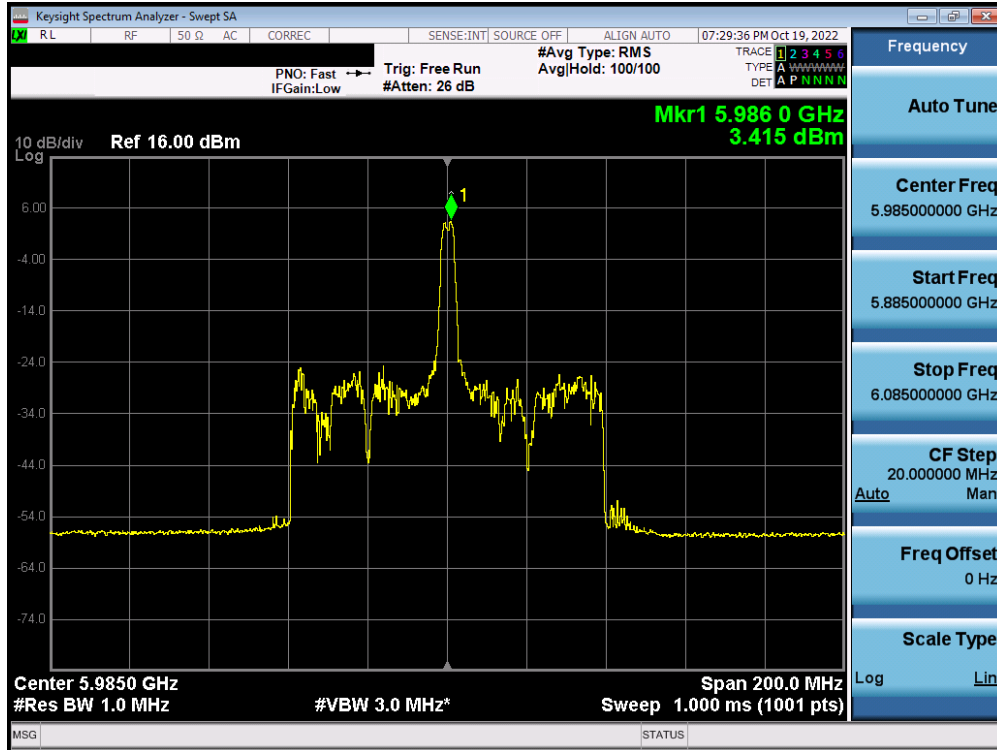
Plot 7-365. Power Spectral Density Plot MIMO ANT2 (80MHz BW 802.11ax (26 Tones) (UNII Band 5) – Ch. 7) – SP
