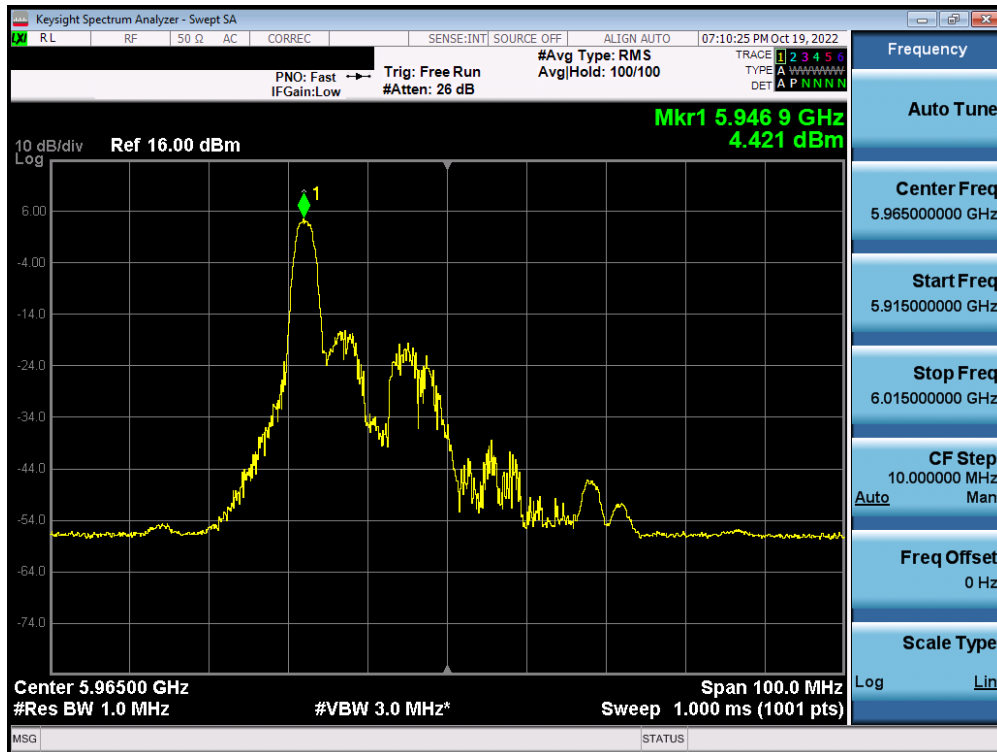
Plot 7-362. Power Spectral Density Plot MIMO ANT2 (40MHz BW 802.11ax (26 Tones) (UNII Band 5) – Ch. 3) – SP
