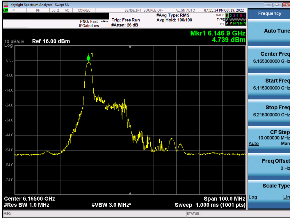
Plot 7-363. Power Spectral Density Plot MIMO ANT2 (40MHz BW 802.11ax (26 Tones) (UNII Band 5) – Ch. 43) – SP
