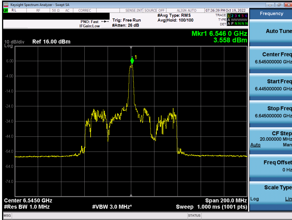
Plot 7-377. Power Spectral Density Plot MIMO ANT2 (80MHz BW 802.11ax (26 Tones) (UNII Band 7) – Ch. 119) – SP
