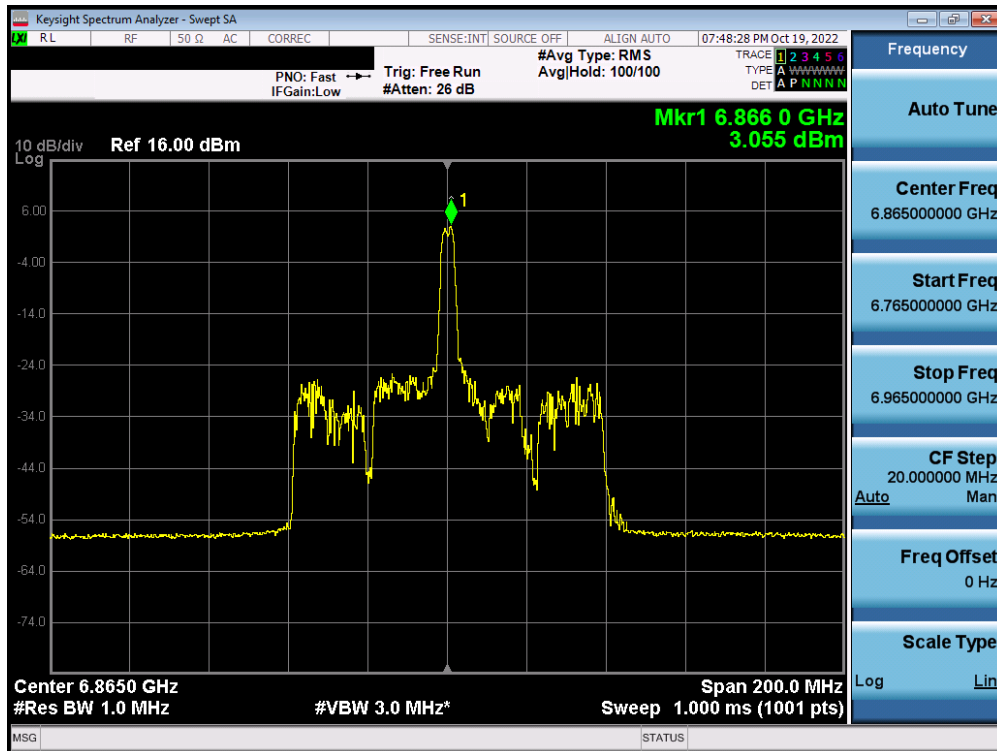
Plot 7-379. Power Spectral Density Plot MIMO ANT2 (80MHz BW 802.11ax (26 Tones) (UNII Band 7) – Ch. 183) – SP
