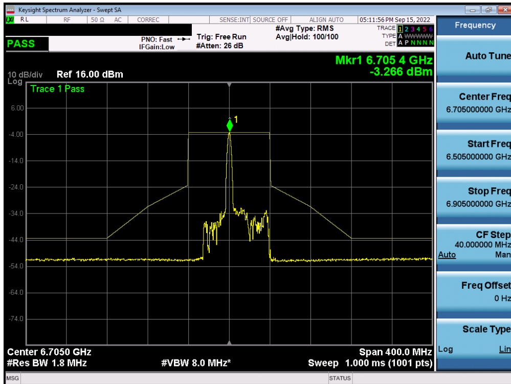
Plot 7-452. In-Band Emission Plot MIMO ANT1 (80MHz BW 802.11ax (26 Tones) (UNII Band 7) – Ch. 151) – LPI
