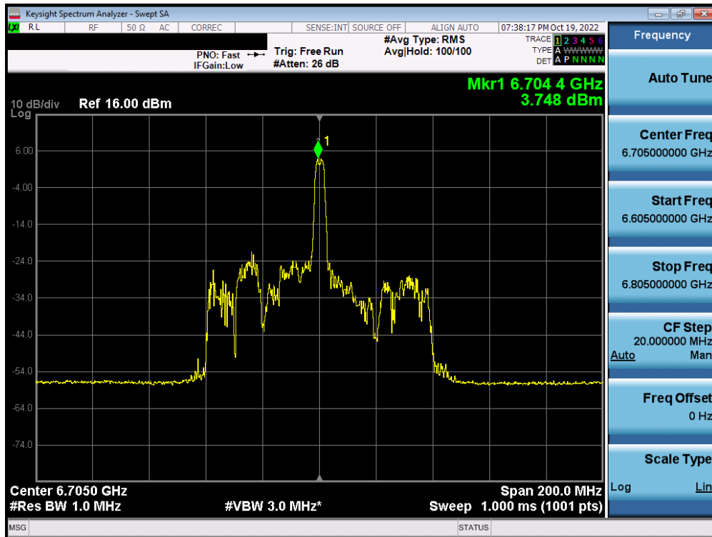
Plot 7-378. Power Spectral Density Plot MIMO ANT2 (80MHz BW 802.11ax (26 Tones) (UNII Band 7) – Ch. 151) – SP
