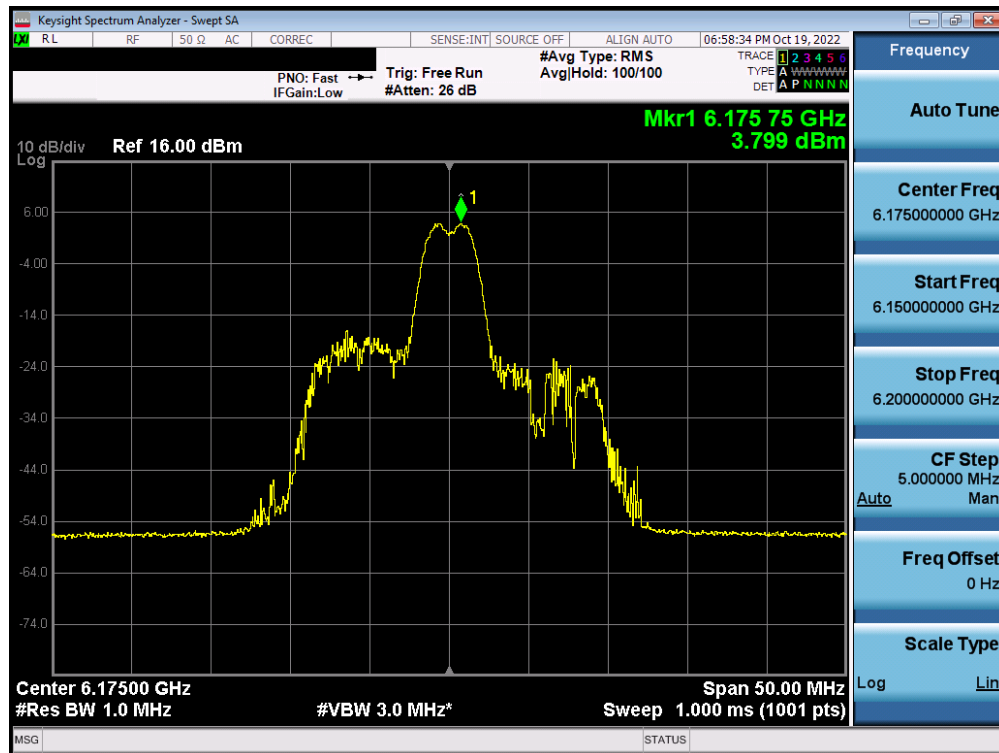
Plot 7-360. Power Spectral Density Plot MIMO ANT2 (20MHz BW 802.11ax (26 Tones) UNII Band 5) – Ch. 45) – SP
