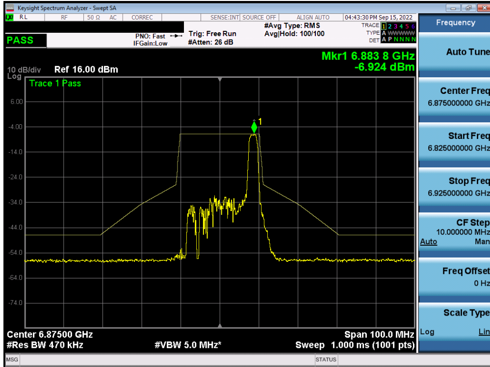
Plot 7-447. In-Band Emission Plot MIMO ANT1 (20MHz BW 802.11ax (26 Tones) (UNII Band 7) – Ch. 185) – LPI
