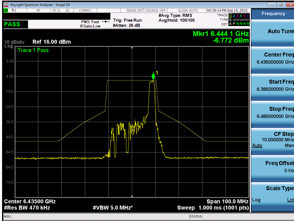
Plot 7-437. In-Band Emission Plot MIMO ANT1 (20MHz BW 802.11ax (26 Tones) (UNII Band 6) – Ch. 97) – LPI
