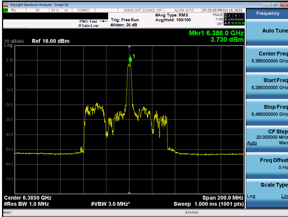
Plot 7-367. Power Spectral Density Plot MIMO ANT2 (80MHz BW 802.11ax (26 Tones) (UNII Band 5) – Ch. 87) – SP
