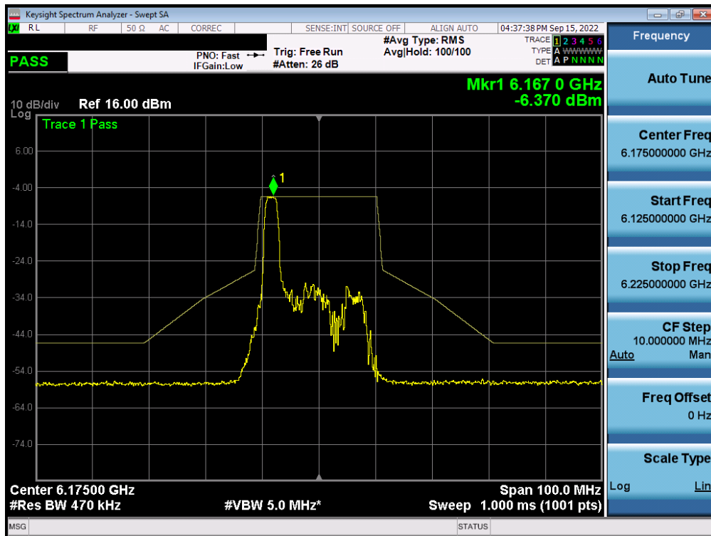
Plot 7-426. In-Band Emission Plot MIMO ANT1 (20MHz BW 802.11ax (26 Tones) (UNII Band 5) – Ch. 45) – LPI
