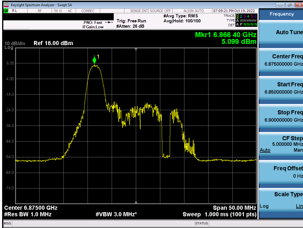
Plot 7-373. Power Spectral Density Plot MIMO ANT2 (20MHz BW 802.11ax (26 Tones) (UNII Band 7) – Ch. 185) – SP
