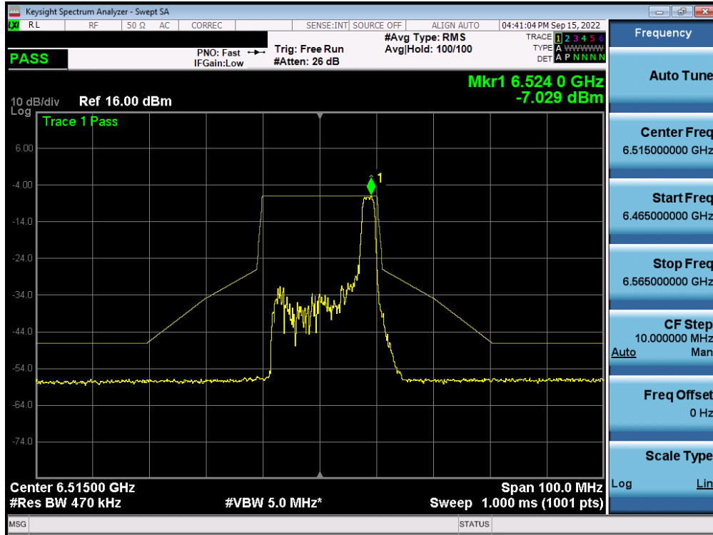
Plot 7-439. In-Band Emission Plot MIMO ANT1 (20MHz BW 802.11ax (26 Tones) (UNII Band 6) – Ch. 113) – LPI
