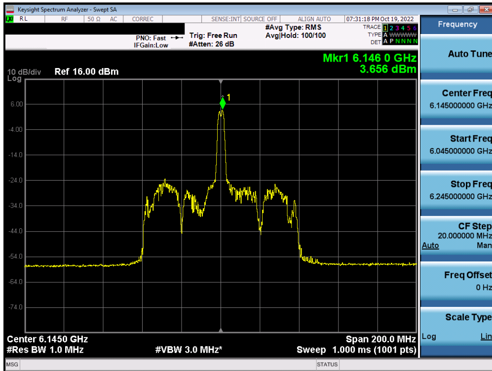
Plot 7-366. Power Spectral Density Plot MIMO ANT2 (80MHz BW 802.11ax (26 Tones) (UNII Band 5) – Ch. 39) – SP
