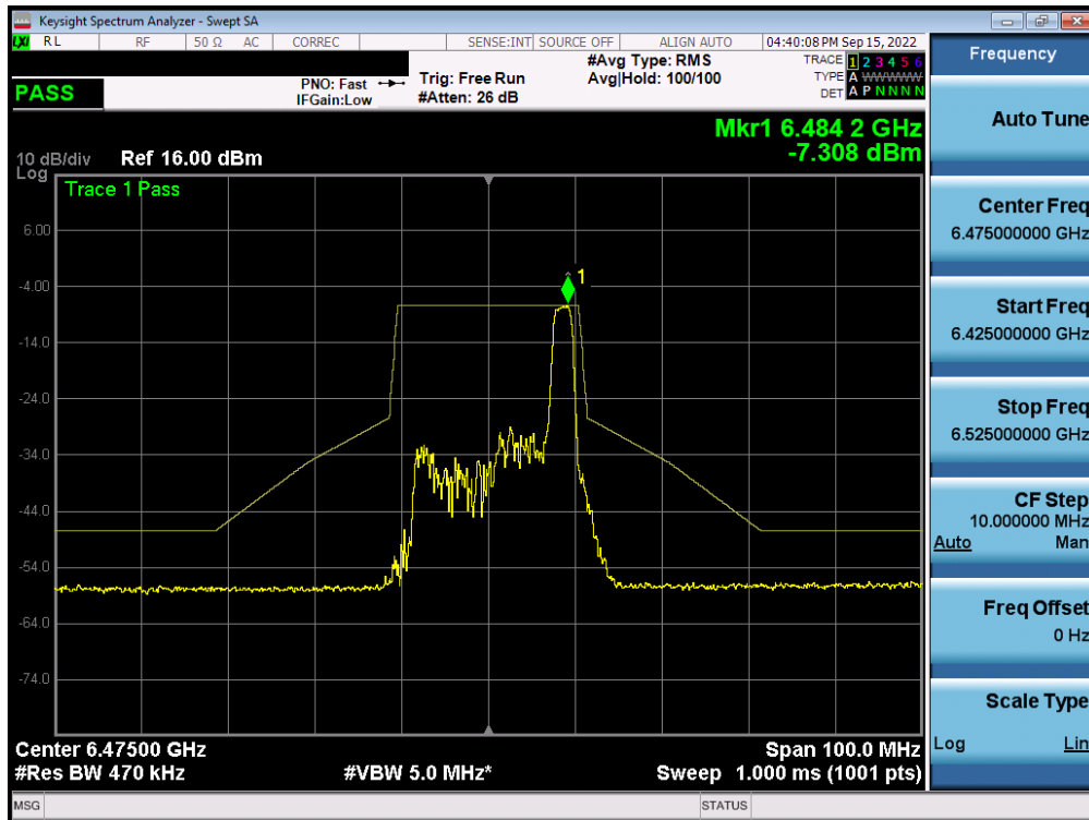
Plot 7-438. In-Band Emission Plot MIMO ANT1 (20MHz BW 802.11ax (26 Tones) (UNII Band 6) – Ch. 105) – LPI
