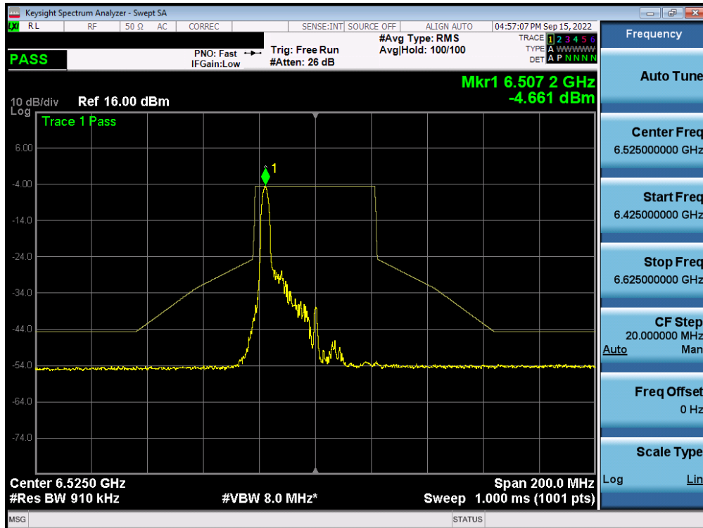
Plot 7-442. In-Band Emission Plot MIMO ANT1 (40MHz BW 802.11ax (26 Tones) (UNII Band 6) – Ch. 115) – LPI
