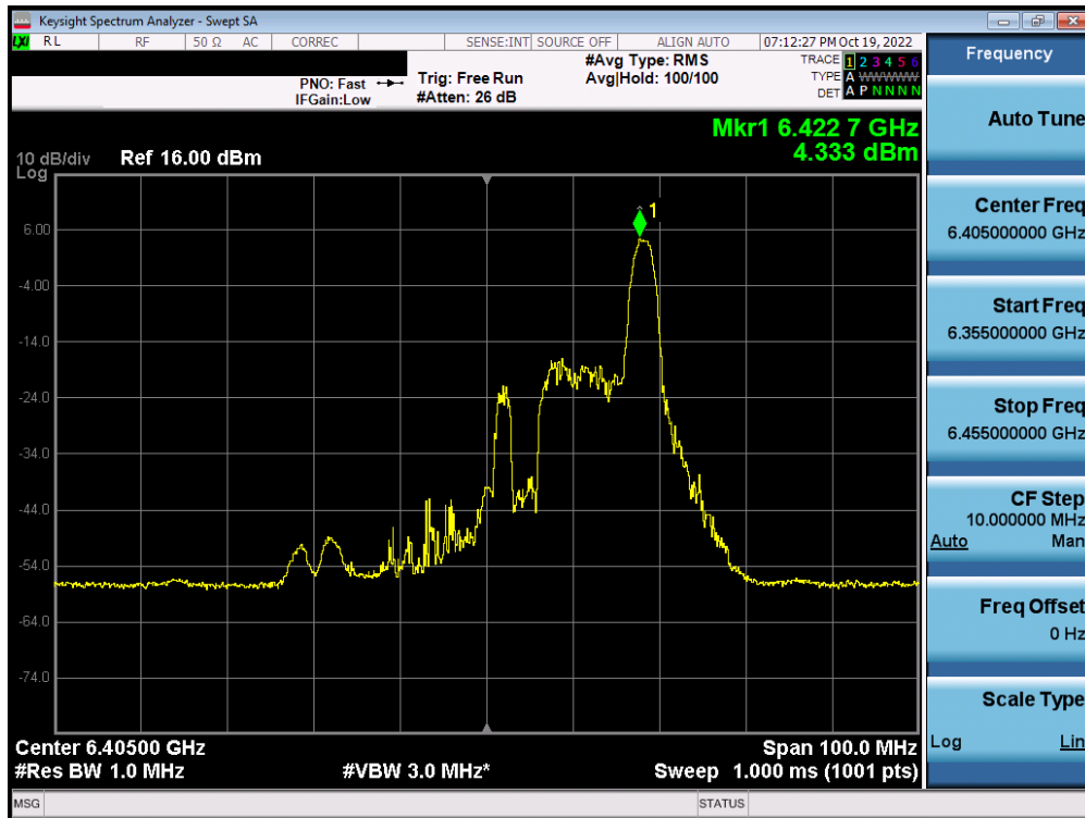
Plot 7-364. Power Spectral Density Plot MIMO ANT2 (40MHz BW 802.11ax (26 Tones) (UNII Band 5) – Ch. 91) – SP
