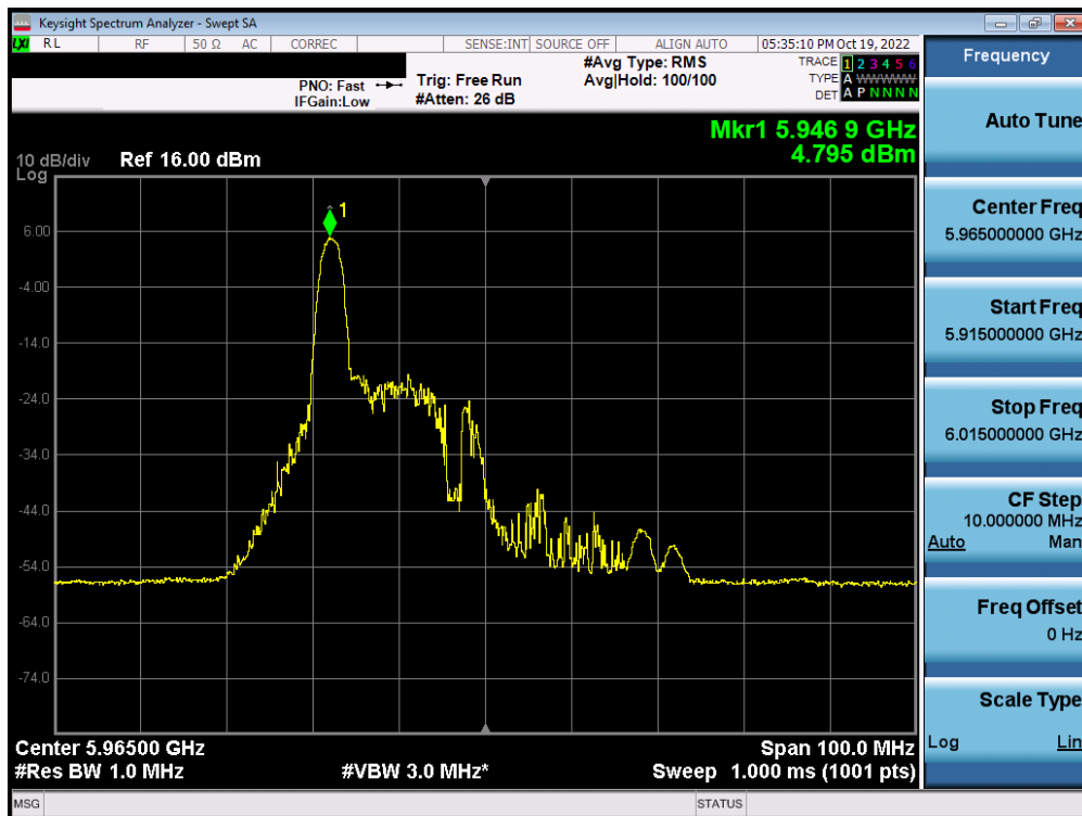
Plot 7-256. Power Spectral Density Plot MIMO ANT1 (40MHz BW 802.11ax (26 Tones) (UNII Band 5) – Ch. 3) – SP
