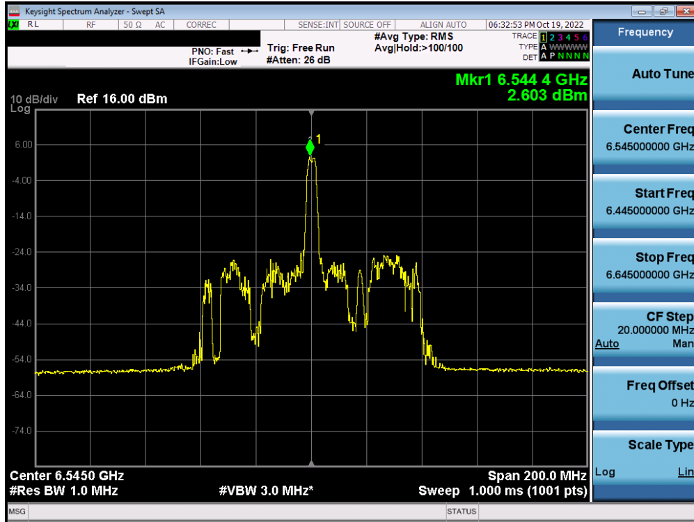
Plot 7-271. Power Spectral Density Plot MIMO ANT1 (80MHz BW 802.11ax (26 Tones) (UNII Band 7) – Ch. 119) – SP
