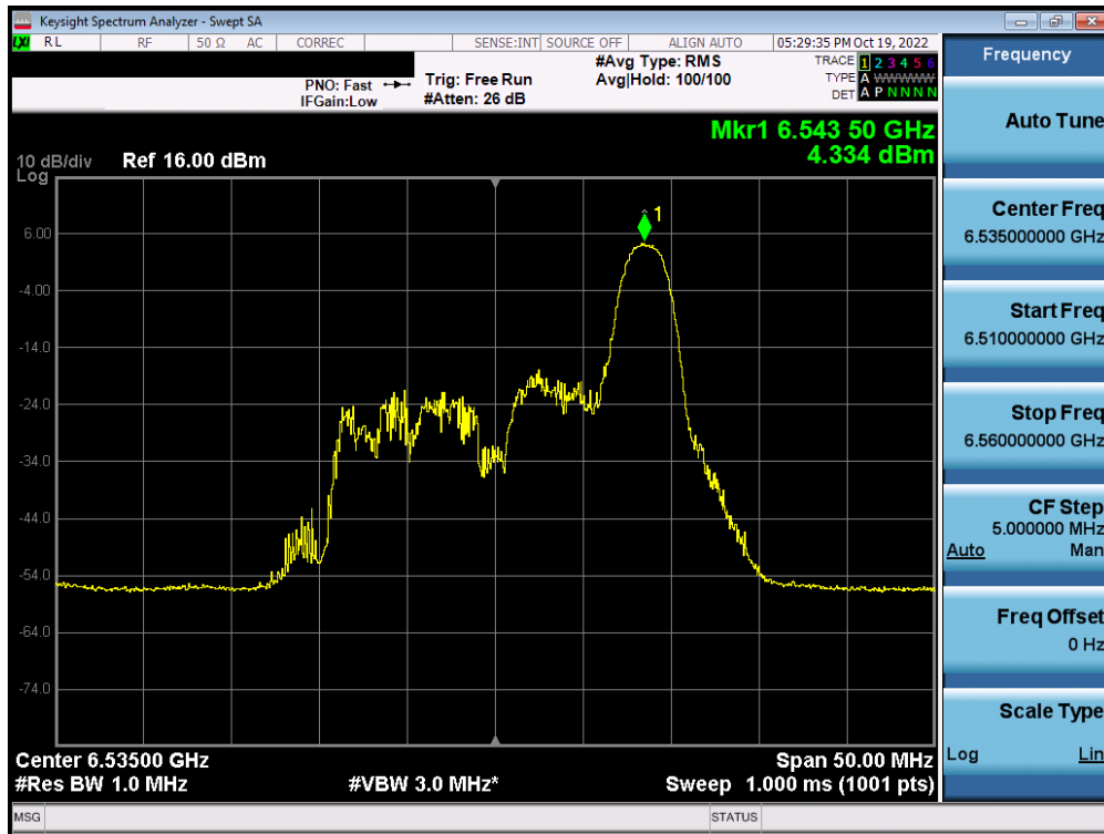
Plot 7-265. Power Spectral Density Plot MIMO ANT1 (20MHz BW 802.11ax (26 Tones) (UNII Band 7) – Ch. 117) – SP
