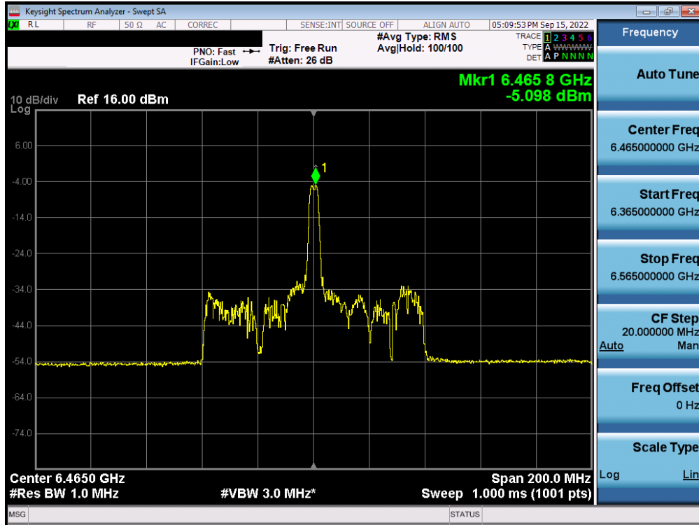
Plot 7-231. Power Spectral Density Plot MIMO ANT1 (80MHz BW 802.11ax (26 Tones) (UNII Band 6) – Ch. 103) – LPI
