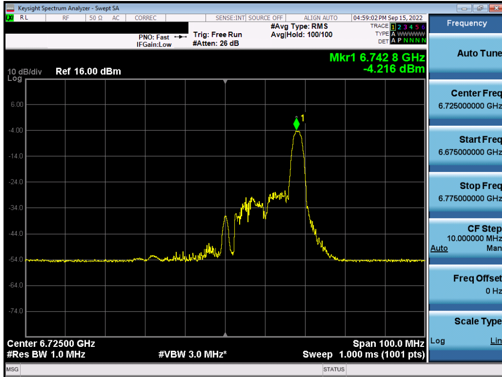
Plot 7-237. Power Spectral Density Plot MIMO ANT1 (40MHz BW 802.11ax (26 Tones) (UNII Band 7) – Ch. 155) – LPI
