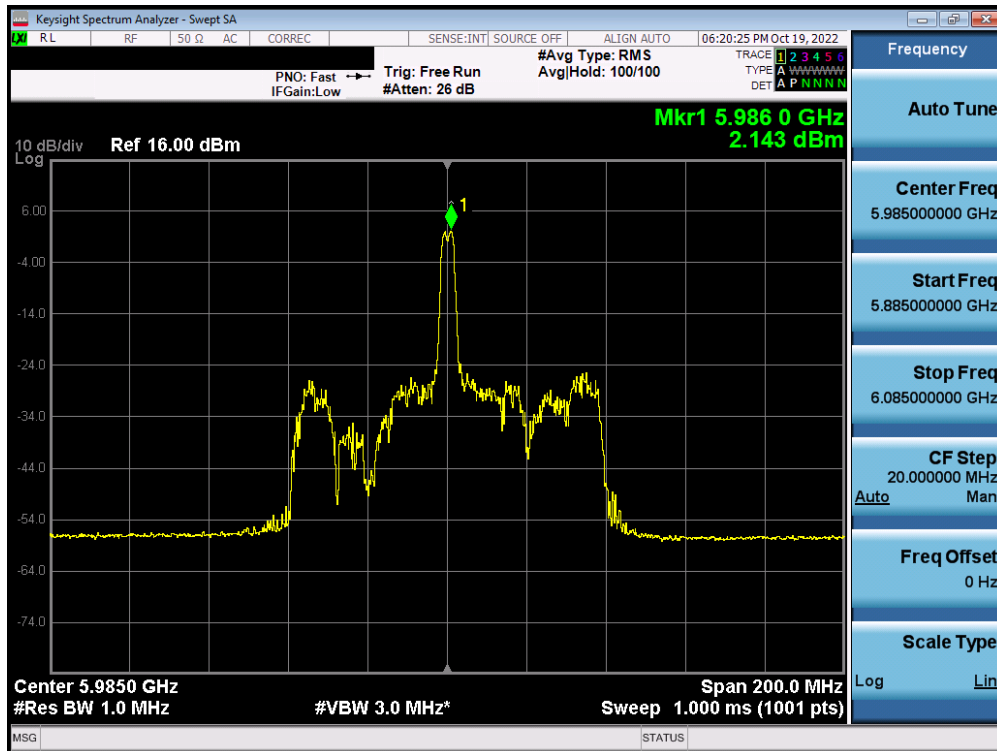
Plot 7-259. Power Spectral Density Plot MIMO ANT1 (80MHz BW 802.11ax (26 Tones) (UNII Band 5) – Ch. 7) – SP
