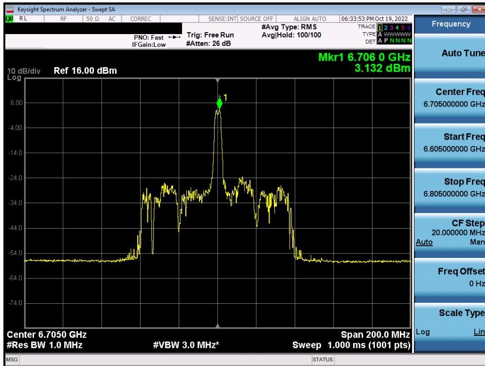
Plot 7-272. Power Spectral Density Plot MIMO ANT1 (80MHz BW 802.11ax (26 Tones) (UNII Band 7) – Ch. 151) – SP
