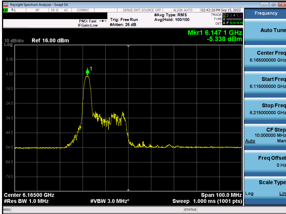
Plot 7-323. Power Spectral Density Plot MIMO ANT2 (40MHz BW 802.11ax (26 Tones) (UNII Band 5) – Ch. 43) – LPI
