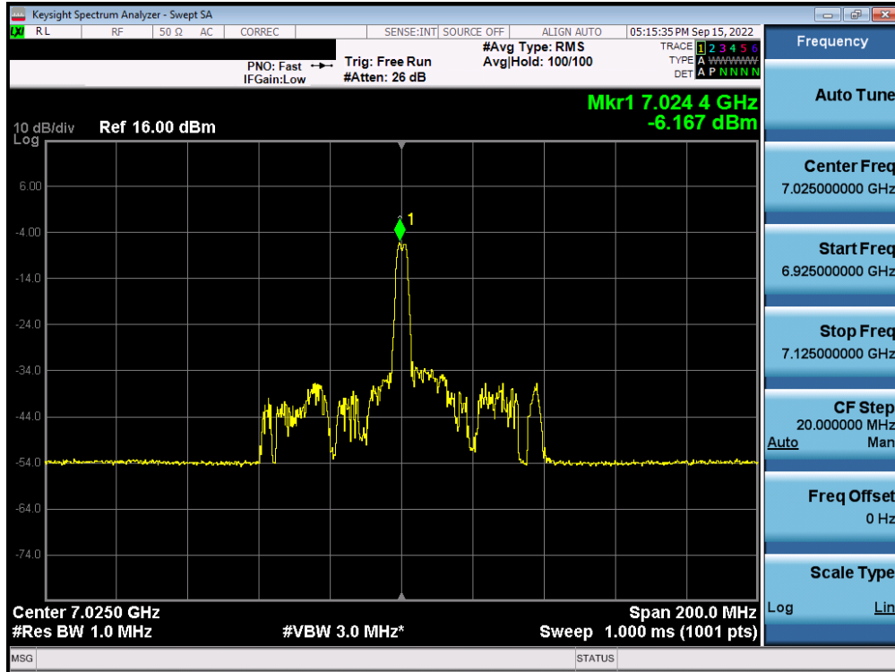
Plot 7-251. Power Spectral Density Plot MIMO ANT1 (80MHz BW 802.11ax (26 Tones) (UNII Band 8) – Ch. 215) – LPI
