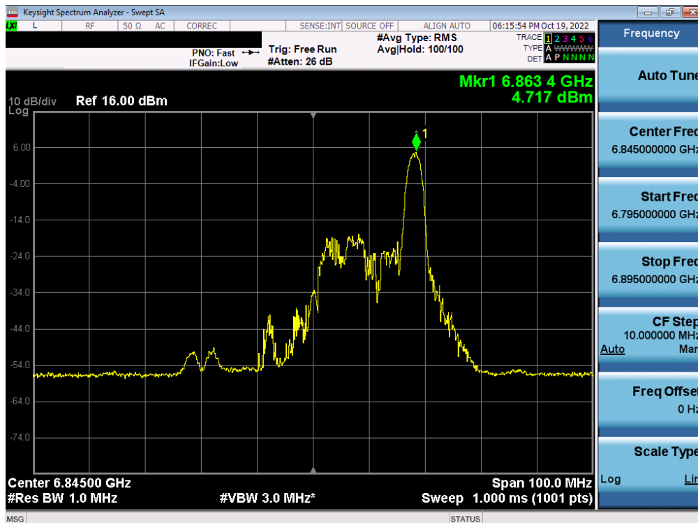
Plot 7-270. Power Spectral Density Plot MIMO ANT1 (40MHz BW 802.11ax (26 Tones) (UNII Band 7) – Ch. 179) – SP
