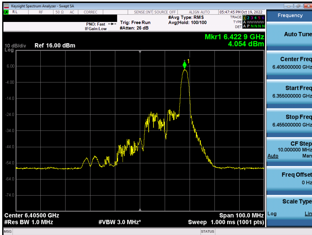
Plot 7-258. Power Spectral Density Plot MIMO ANT1 (40MHz BW 802.11ax (26 Tones) (UNII Band 5) – Ch. 91) – SP
