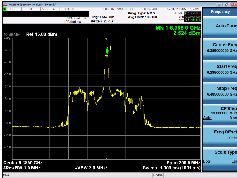
Plot 7-261. Power Spectral Density Plot MIMO ANT1 (80MHz BW 802.11ax (26 Tones) (UNII Band 5) – Ch. 87) – SP
