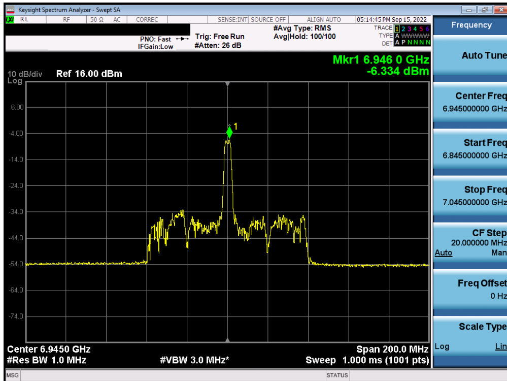
Plot 7-250. Power Spectral Density Plot MIMO ANT1 (80MHz BW 802.11ax (26 Tones) (UNII Band 8) – Ch. 199) – LPI
