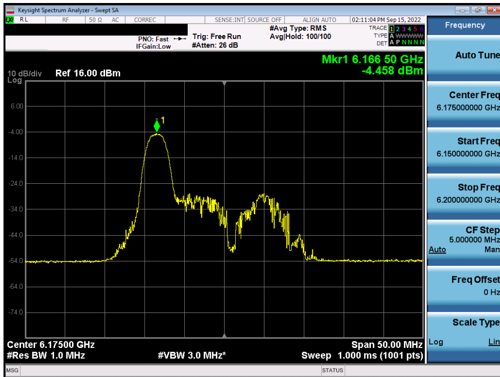
Plot 7-320. Power Spectral Density Plot MIMO ANT2 (20MHz BW 802.11ax (26 Tones) (UNII Band 5) – Ch. 45) – LPI
