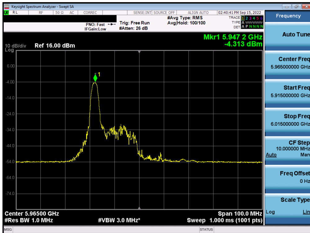
Plot 7-322. Power Spectral Density Plot MIMO ANT2 (40MHz BW 802.11ax (26 Tones) (UNII Band 5) – Ch. 3) – LPI
