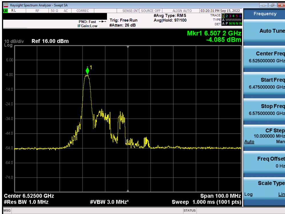
Plot 7-336. Power Spectral Density Plot MIMO ANT2 (40MHz BW 802.11ax (26 Tones) (UNII Band 6) – Ch. 115) – LPI
