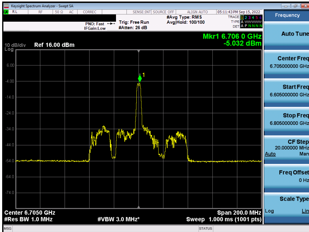
Plot 7-240. Power Spectral Density Plot MIMO ANT1 (80MHz BW 802.11ax (26 Tones) (UNII Band 7) – Ch. 151) – LPI
