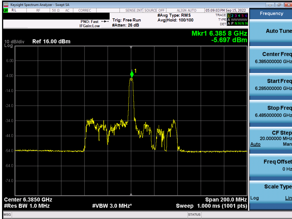
Plot 7-221. Power Spectral Density Plot MIMO ANT1 (80MHz BW 802.11ax (26 Tones) (UNII Band 5) – Ch. 87) – LPI
