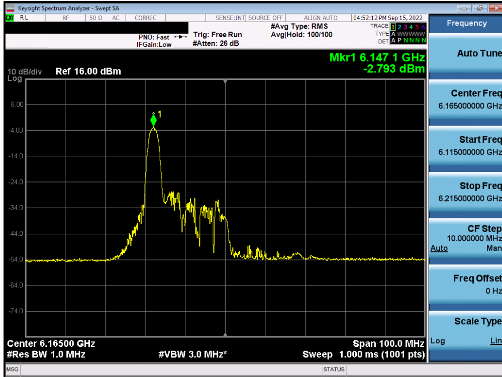
Plot 7-217. Power Spectral Density Plot MIMO ANT1 (40MHz BW 802.11ax (26 Tones) (UNII Band 5) – Ch. 43) – LPI
