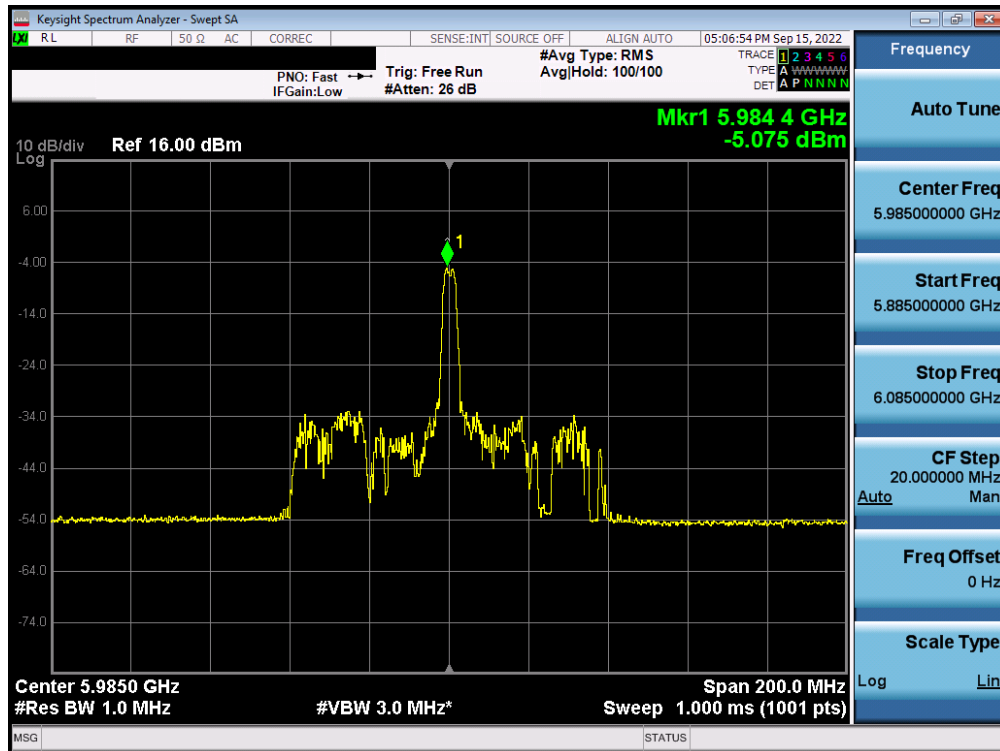
Plot 7-219. Power Spectral Density Plot MIMO ANT1 (80MHz BW 802.11ax (26 Tones) (UNII Band 5) – Ch. 7) – LPI
