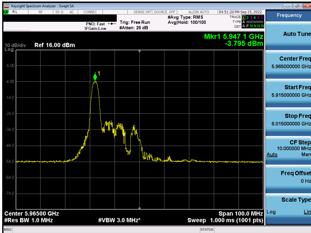
Plot 7-216. Power Spectral Density Plot MIMO ANT1 (40MHz BW 802.11ax (26 Tones) (UNII Band 5) – Ch. 3) – LPI
