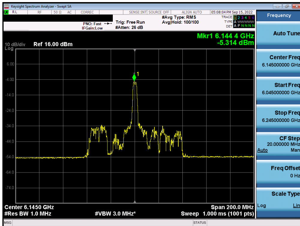
Plot 7-220. Power Spectral Density Plot MIMO ANT1 (80MHz BW 802.11ax (26 Tones) (UNII Band 5) – Ch. 39) – LPI
