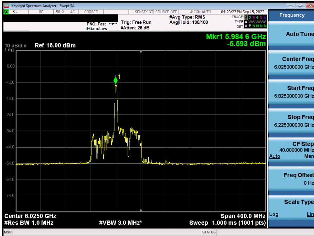
Plot 7-222. Power Spectral Density Plot MIMO ANT1 (160MHz BW 802.11ax (26 Tones) (UNII Band 5) – Ch. 15) – LPI
