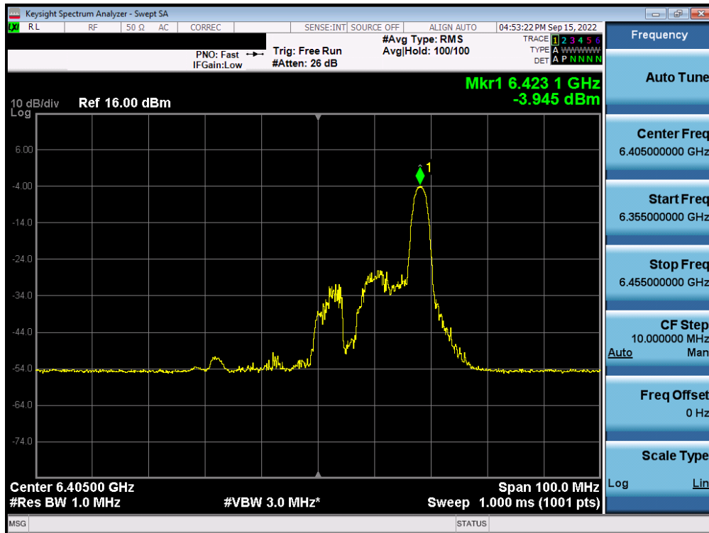
Plot 7-218. Power Spectral Density Plot MIMO ANT1 (40MHz BW 802.11ax (26 Tones) (UNII Band 5) – Ch. 91) – LPI
