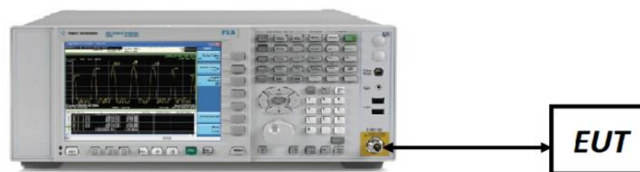
Figure 7-1. Test Instrument & Measurement Setup
