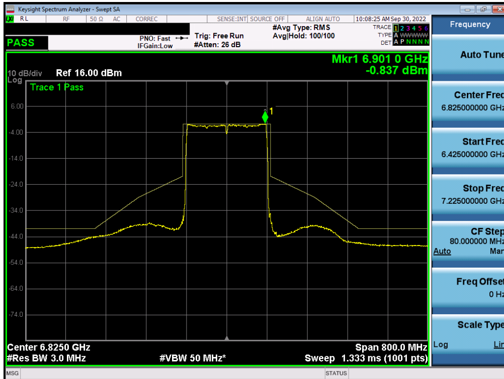
Plot 7-300. In-Band Emission Plot Measurement MIMO ANT2 (160MHz 802.11ax (UNII Band 7) – Ch. 175)
