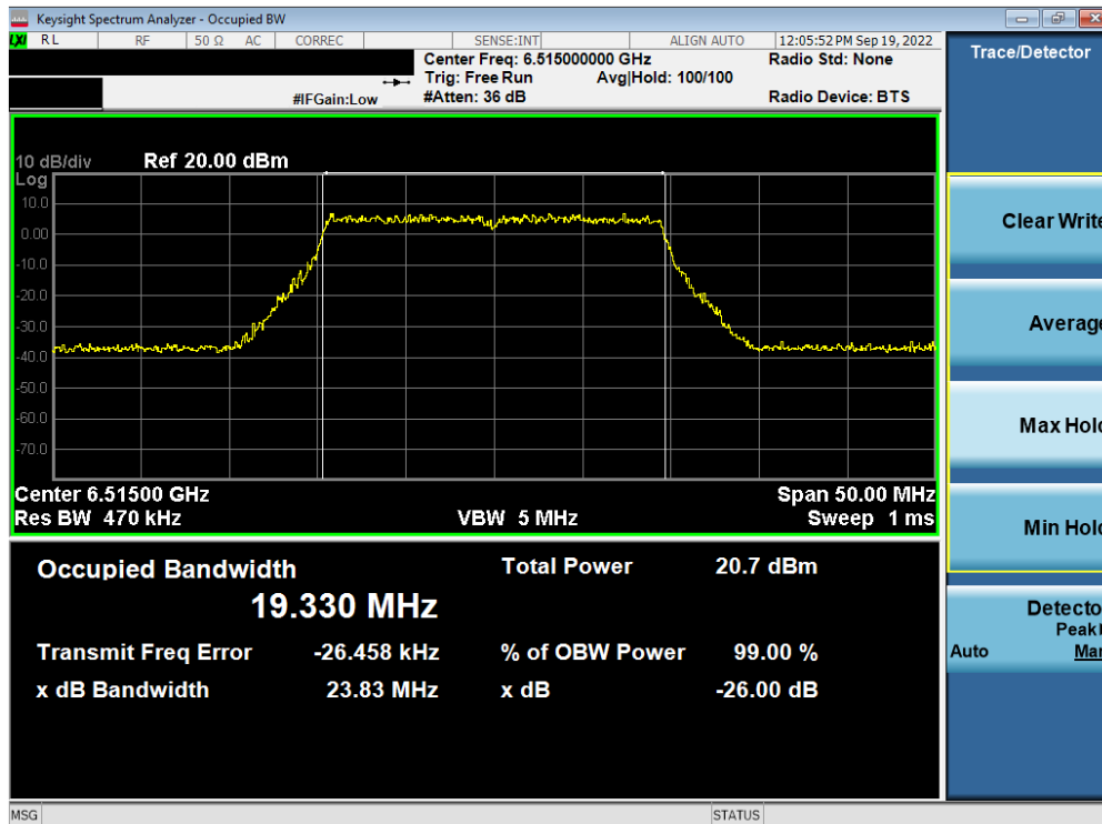
Plot 7-21. 26dB Bandwidth Plot MIMO ANT1 (20MHz 802.11ax (UNII Band 6) – Ch. 113)
