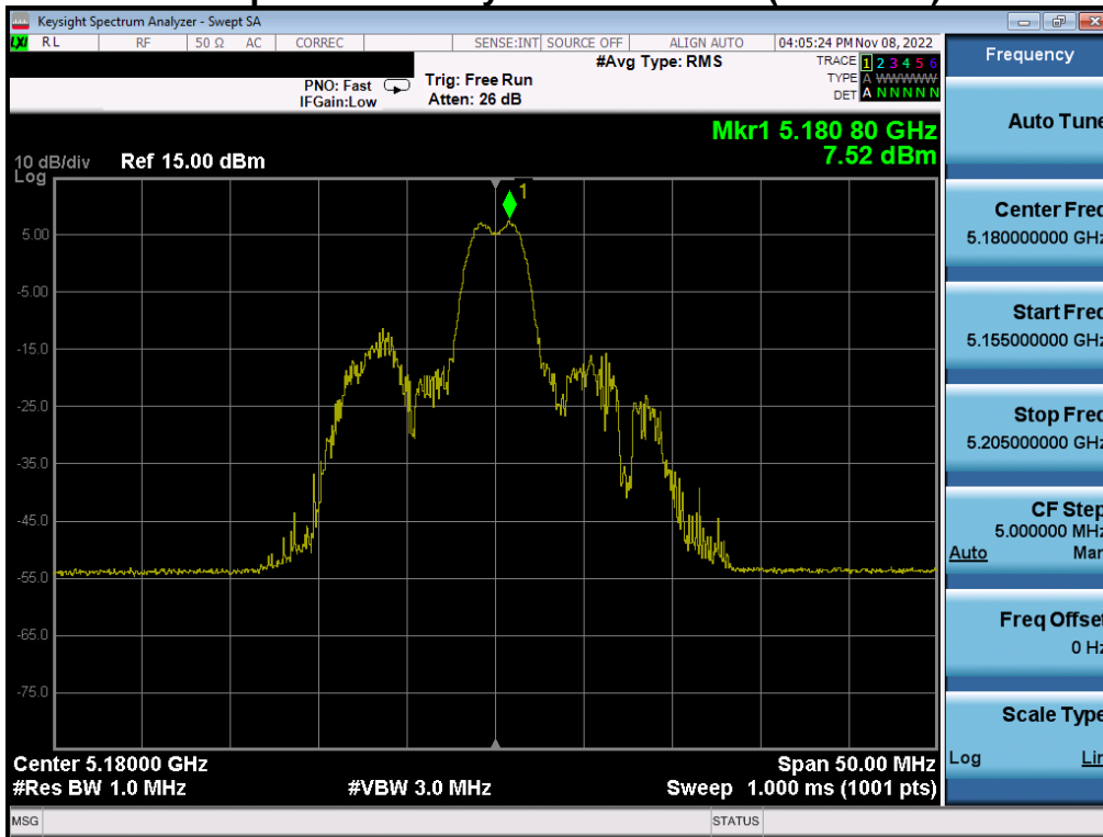
Plot 7-226. Power Spectral Density Plot MIMO ANT2 (20MHz BW 802.11ax – 26 Tones (UNII Band 1) – Ch. 36)
