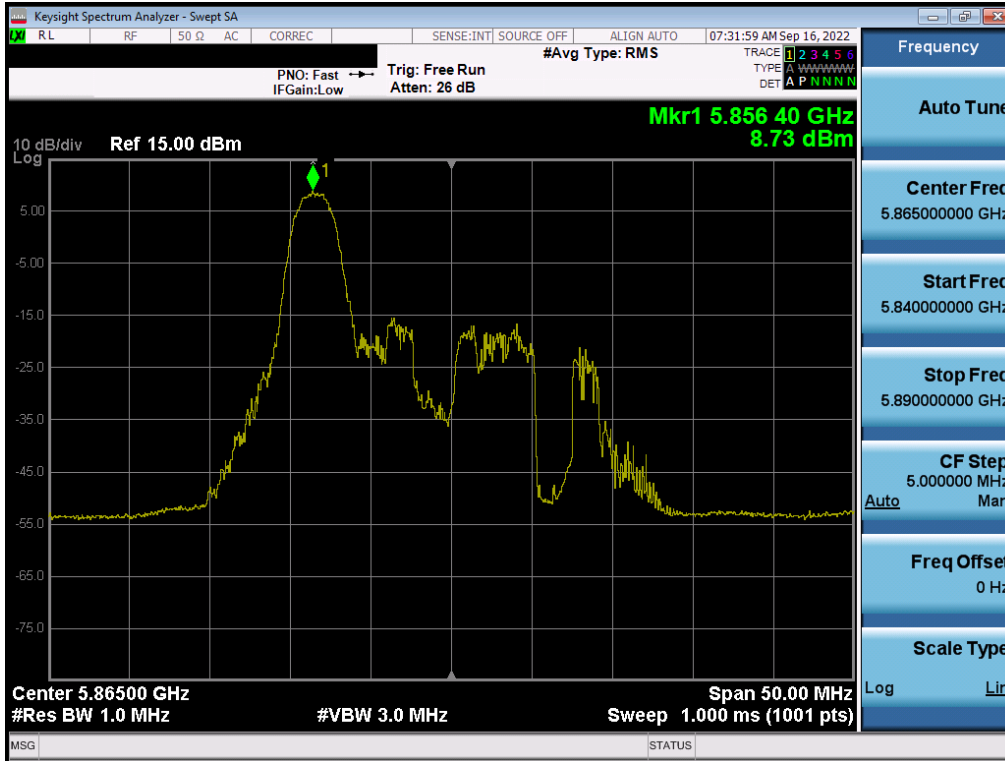
Plot 7-258. Power Spectral Density Plot MIMO ANT2 (20MHz BW 802.11ax – 26 Tones (UNII Band 4) – Ch. 173)
