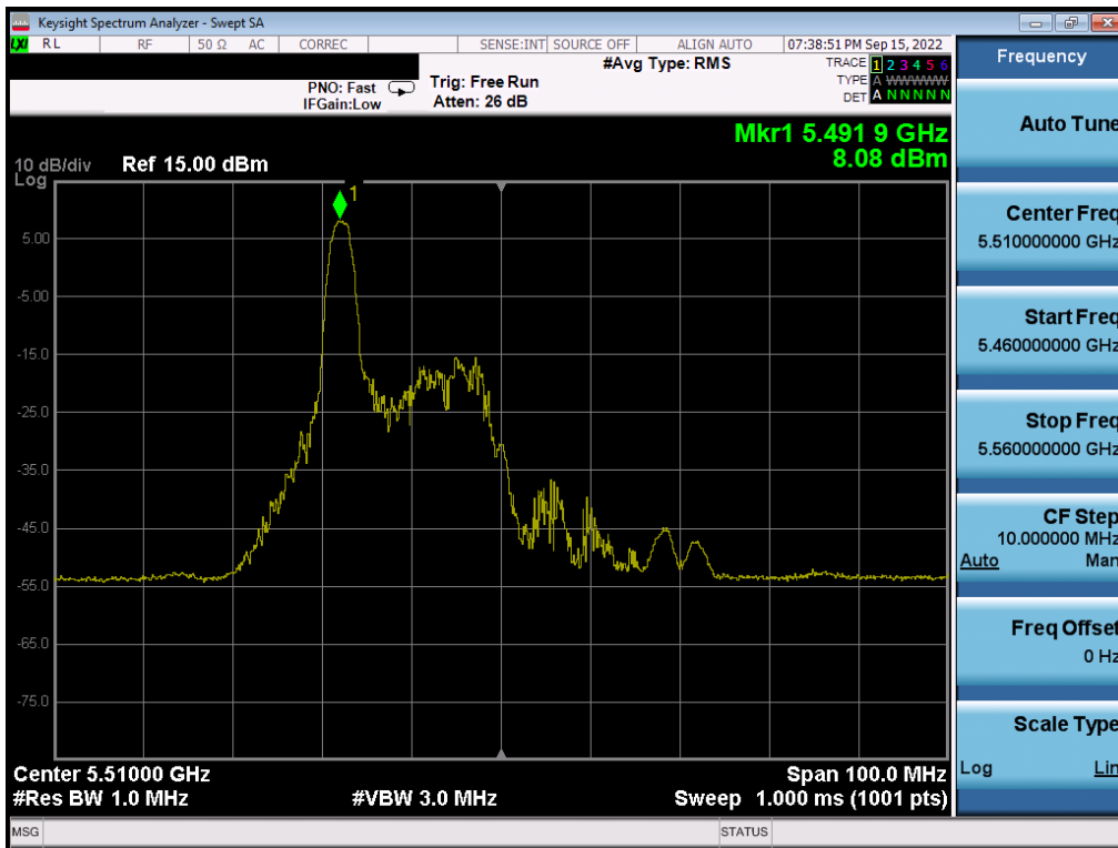
Plot 7-243. Power Spectral Density Plot MIMO ANT2 (40MHz BW 802.11ax – 26 Tones (UNII Band 2C) – Ch. 102)
