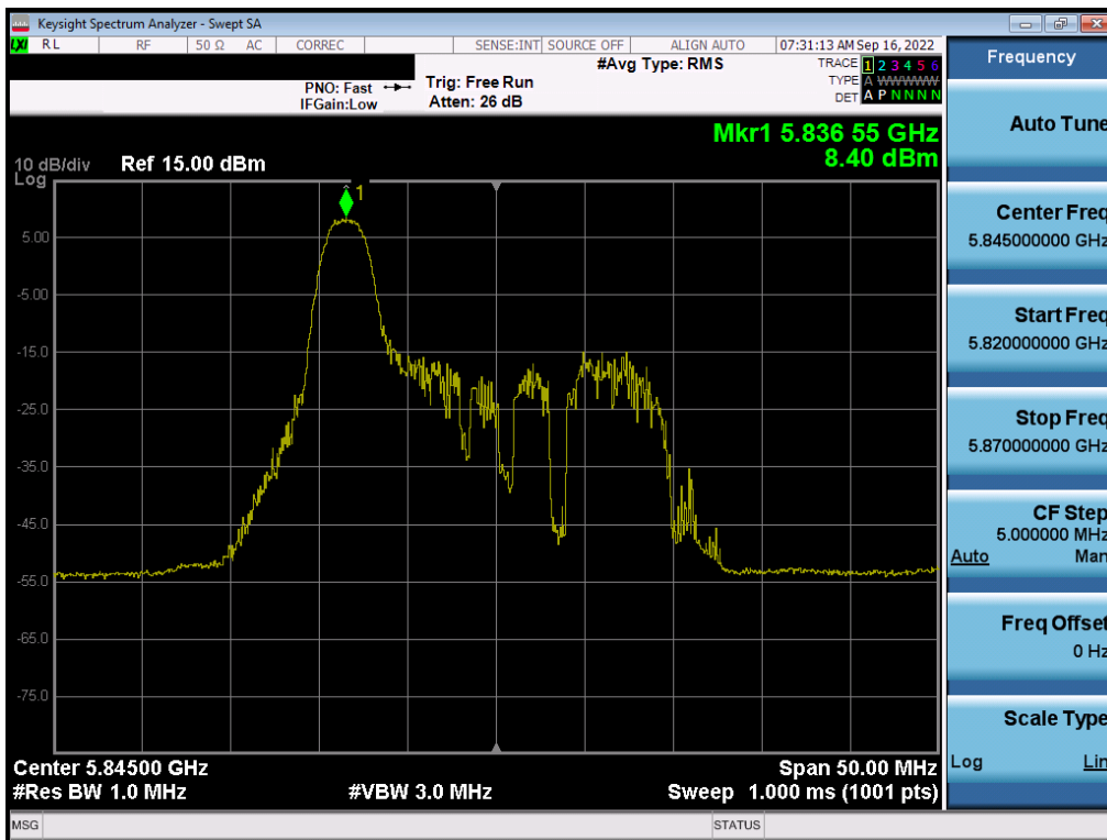
Plot 7-257. Power Spectral Density Plot MIMO ANT2 (20MHz BW 802.11ax – 26 Tones (UNII Band 3/4) – Ch. 169)
