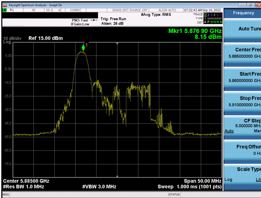
Plot 7-259. Power Spectral Density Plot MIMO ANT2 (20MHz BW 802.11ax – 26 Tones (UNII Band 4) – Ch. 177)
