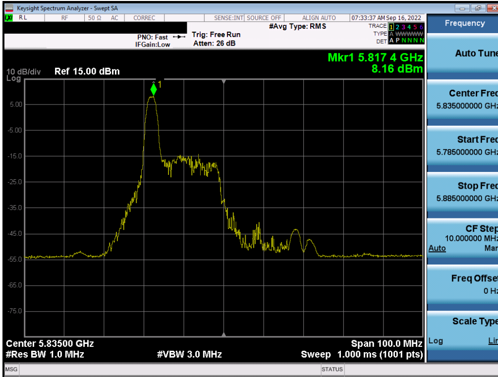
Plot 7-260. Power Spectral Density Plot MIMO ANT2 (40MHz BW 802.11ax – 26 Tones (UNII Band 3/4) – Ch. 167)
