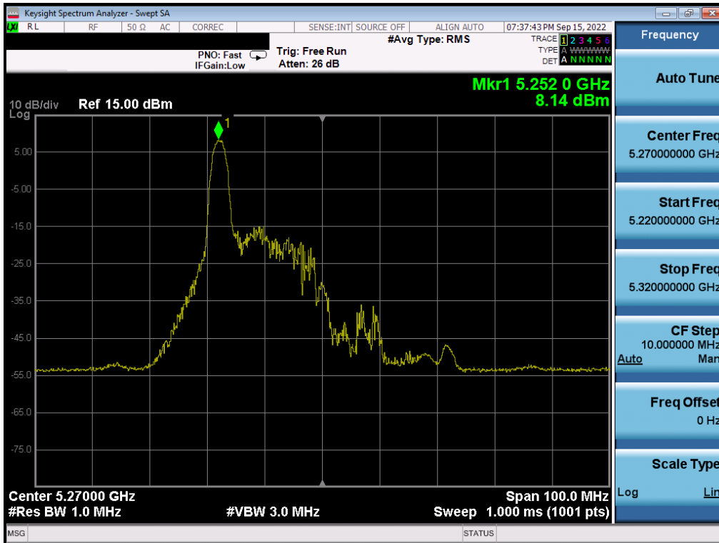
Plot 7-237. Power Spectral Density Plot MIMO ANT2 (40MHz BW 802.11ax – 26 Tones (UNII Band 2A) – Ch. 54)
