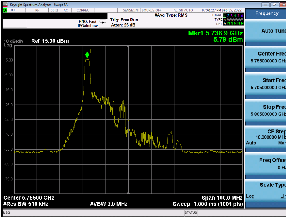
Plot 7-254. Power Spectral Density Plot MIMO ANT2 (40MHz BW 802.11ax – 26 Tones (UNII Band 3) – Ch. 151)
