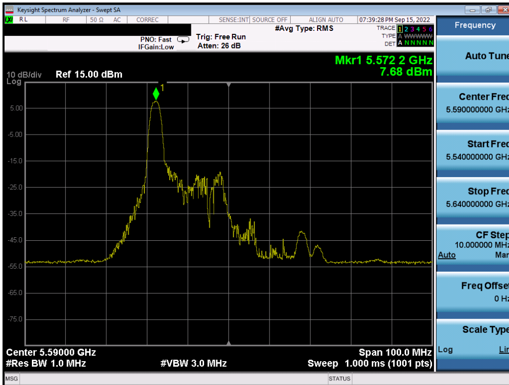
Plot 7-244. Power Spectral Density Plot MIMO ANT2 (40MHz BW 802.11ax – 26 Tones (UNII Band 2C) – Ch. 118)
