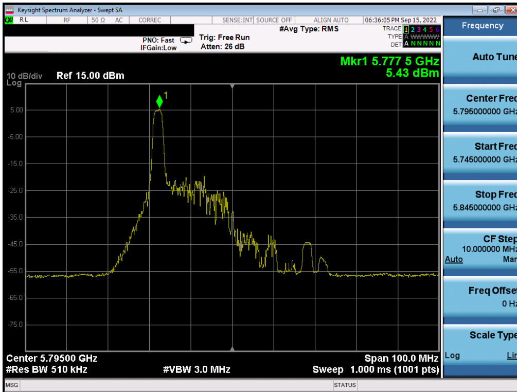
Plot 7-180. Power Spectral Density Plot MIMO ANT1 (40MHz BW 802.11ax – 26 Tones (UNII Band 3) – Ch. 159)
