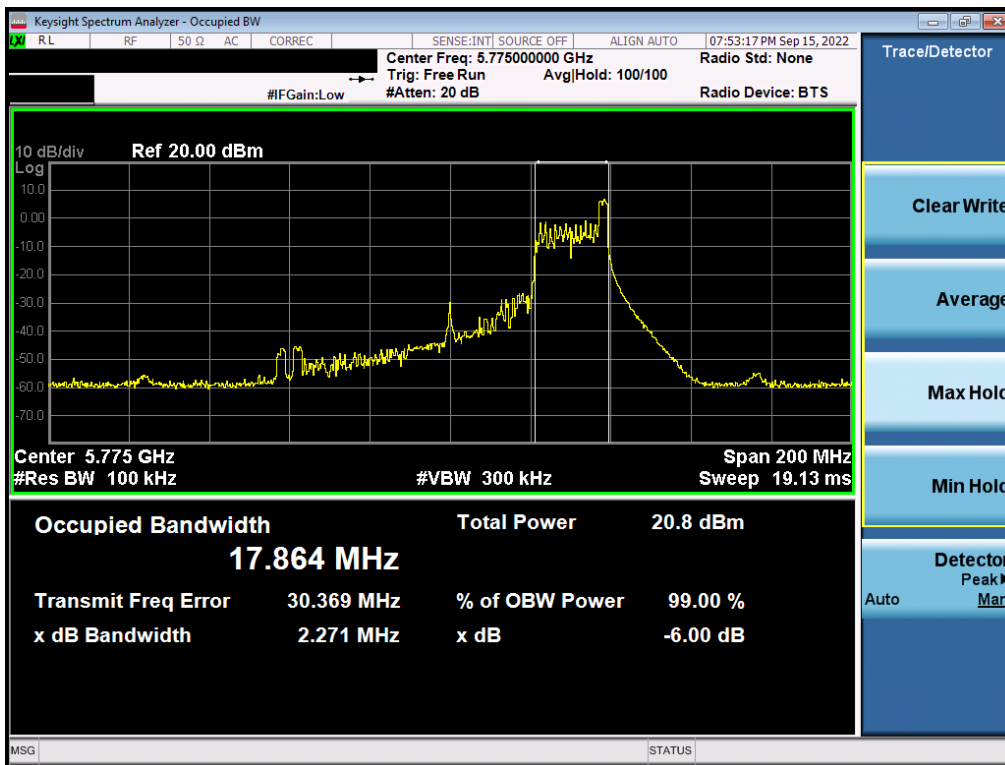
Plot 7-129. 6dB Bandwidth Plot MIMO ANT2 (80MHz BW 802.11ax – 26 Tones (UNII Band 3) – Ch. 155)
