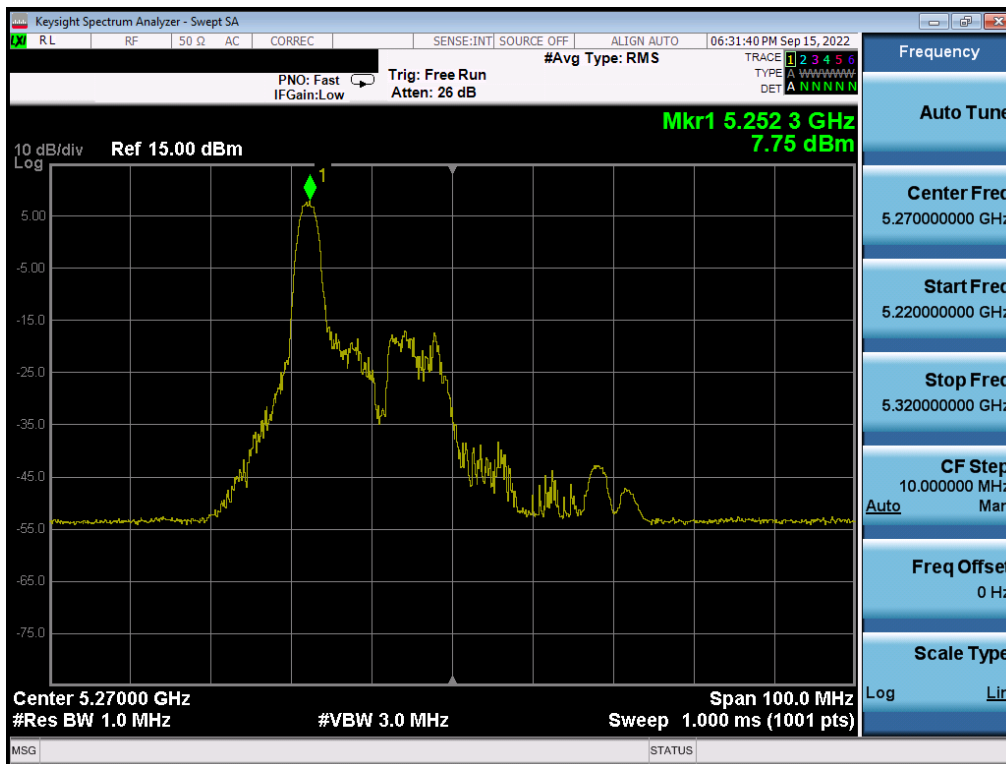
Plot 7-162. Power Spectral Density Plot MIMO ANT1 (40MHz BW 802.11ax – 26 Tones (UNII Band 2A) – Ch. 54)
