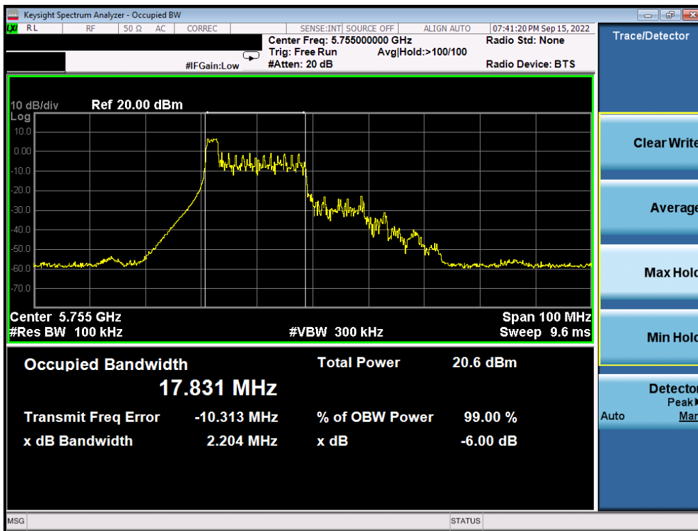
Plot 7-127. 6dB Bandwidth Plot MIMO ANT2 (40MHz BW 802.11ax – 26 Tones (UNII Band 3) – Ch. 151)
