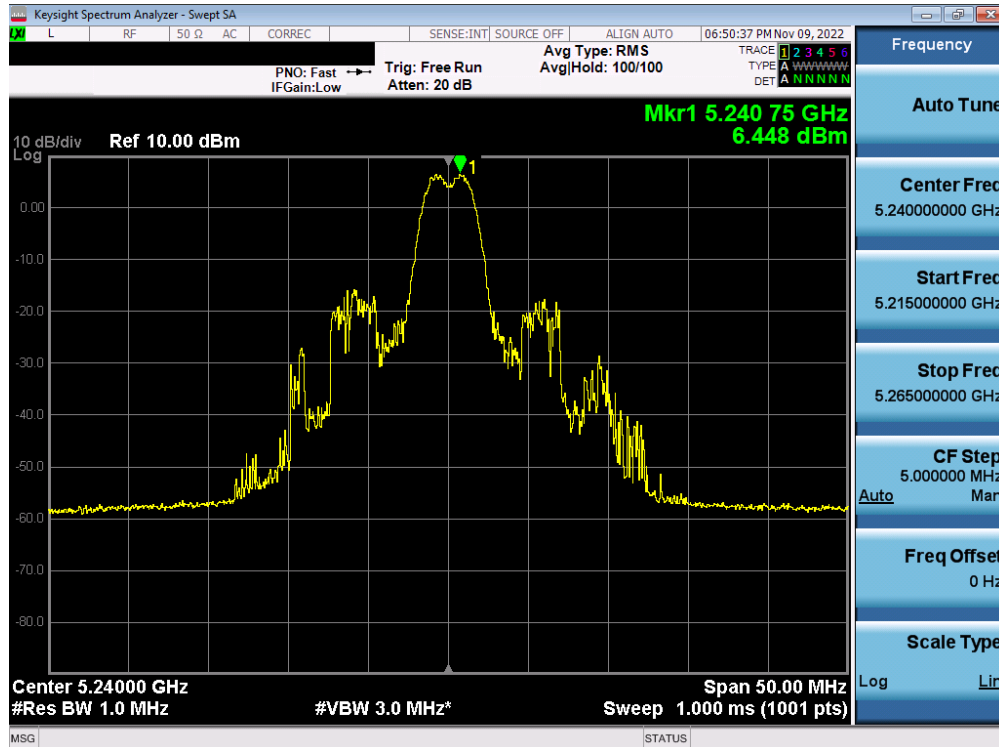
Plot 7-153. Power Spectral Density Plot MIMO ANT1 (20MHz BW 802.11ax – 26 Tones (UNII Band 1) – Ch. 48)
