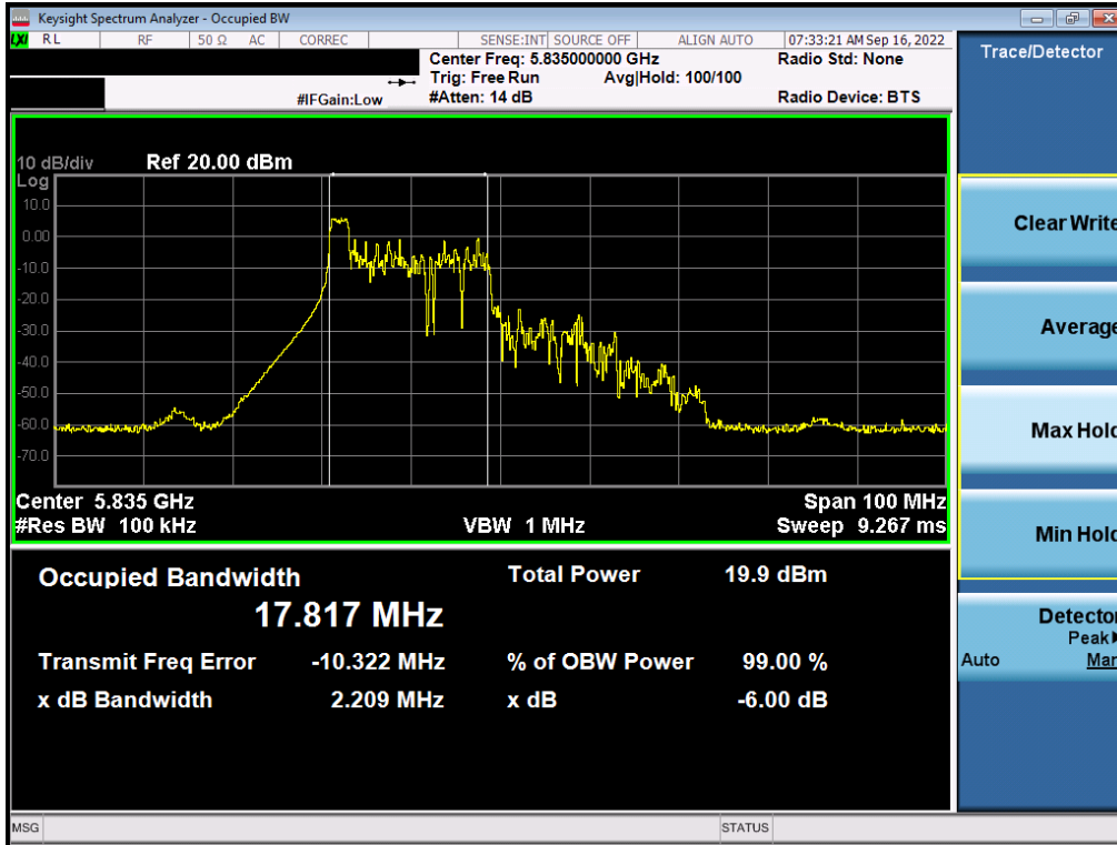
Plot 7-133. 6dB Bandwidth Plot MIMO ANT2 (40MHz BW 802.11ax – 26 Tones (UNII Band 3/4) – Ch. 167)
