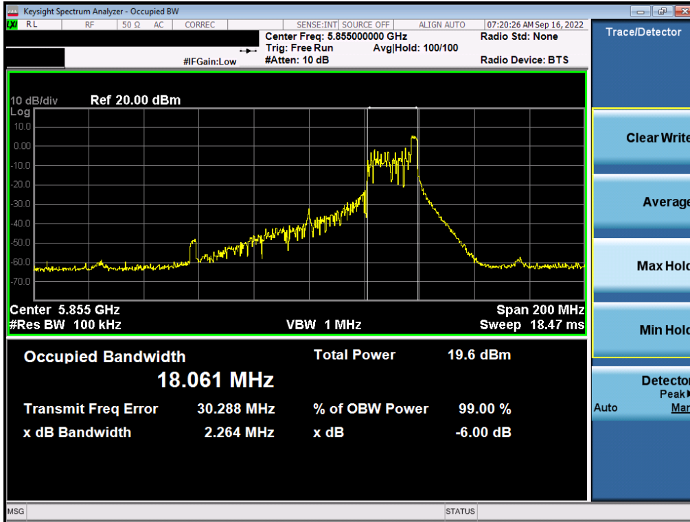
Plot 7-108. 6dB Bandwidth Plot MIMO ANT1 (80MHz BW 802.11ax – 26 Tones (UNII Band 3/4) – Ch. 171)
