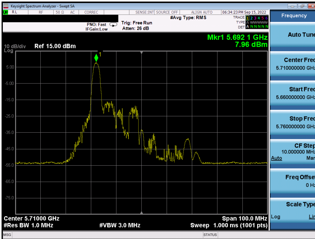
Plot 7-170. Power Spectral Density Plot MIMO ANT1 (40MHz BW 802.11ax – 26 Tones (UNII Band 2C) – Ch. 142)
