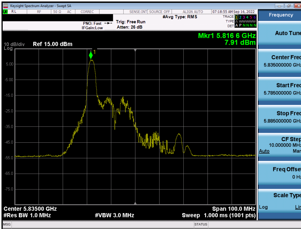
Plot 7-185. Power Spectral Density Plot MIMO ANT1 (40MHz BW 802.11ax – 26 Tones (UNII Band 3/4) – Ch. 167)
