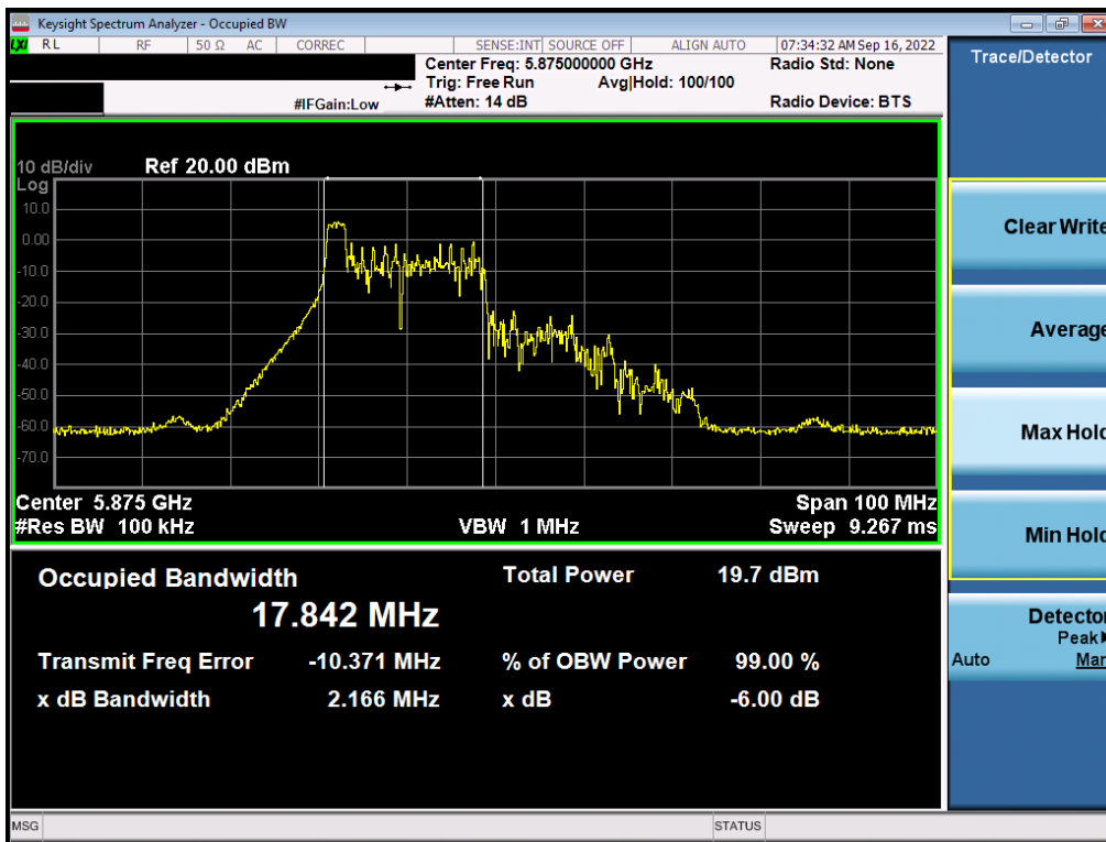
Plot 7-134. 6dB Bandwidth Plot MIMO ANT2 (40MHz BW 802.11ax – 26 Tones (UNII Band 4) – Ch. 175)
