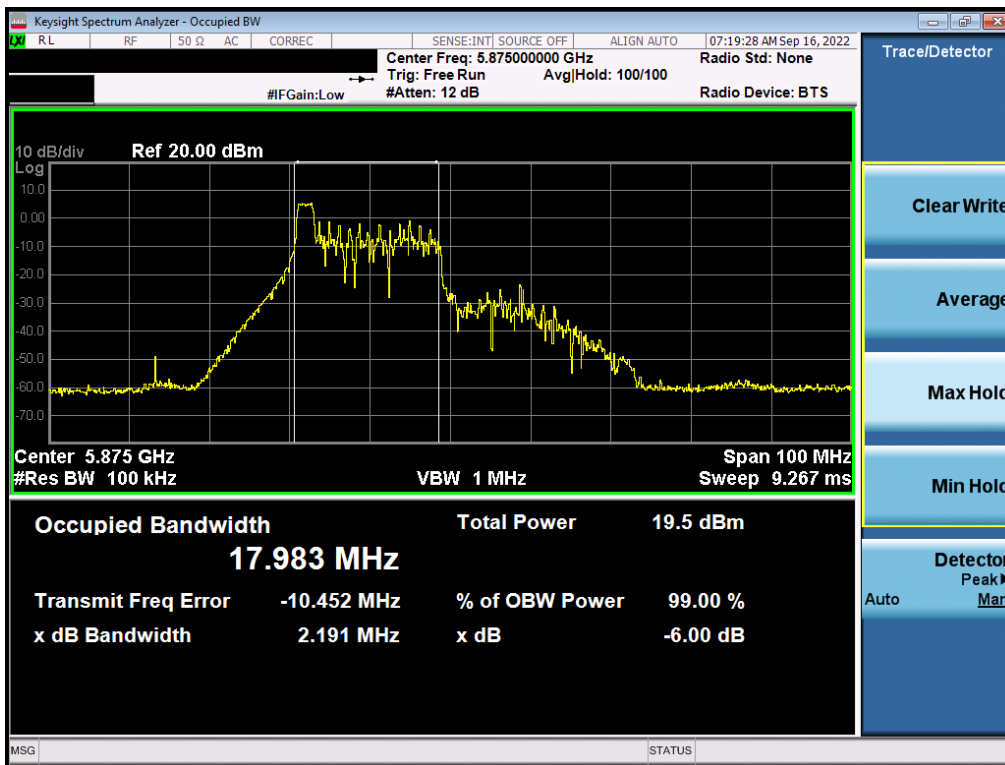
Plot 7-107. 6dB Bandwidth Plot MIMO ANT1 (40MHz BW 802.11ax – 26 Tones (UNII Band 4) – Ch. 175)
