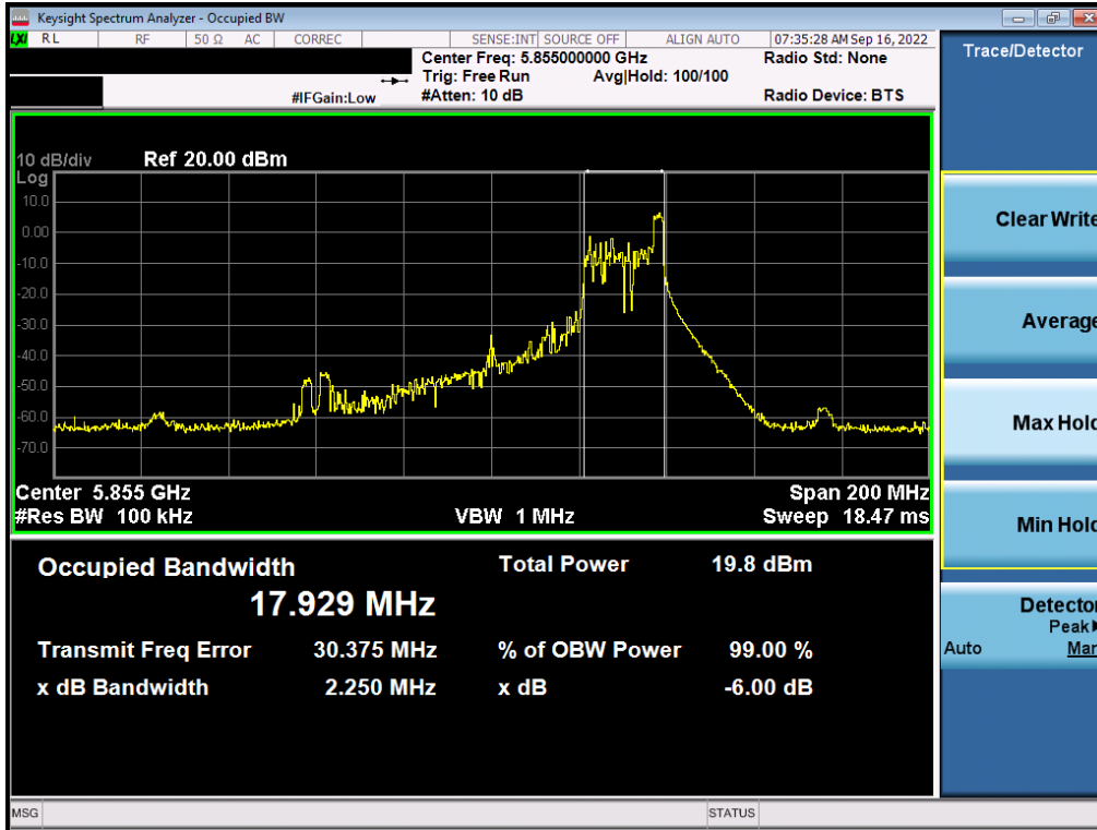
Plot 7-135. 6dB Bandwidth Plot MIMO ANT2 (80MHz BW 802.11ax – 26 Tones (UNII Band 3/4) – Ch. 171)
