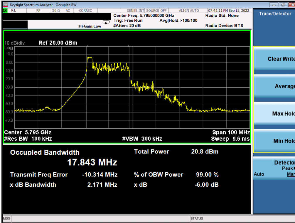
Plot 7-128. 6dB Bandwidth Plot MIMO ANT2 (40MHz BW 802.11ax – 26 Tones (UNII Band 3) – Ch. 159)
