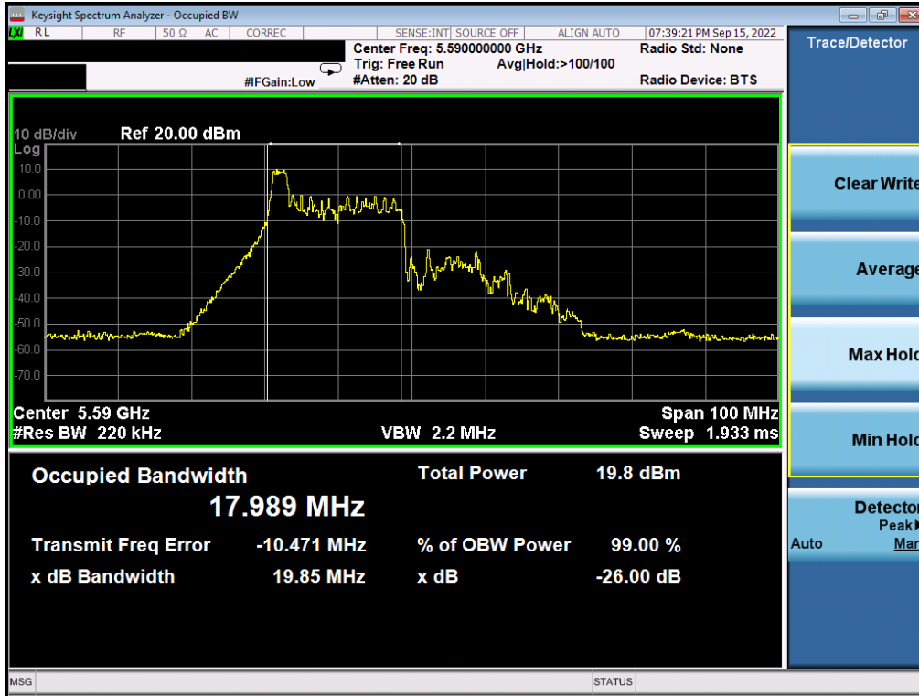
Plot 7-67. 26dB Bandwidth Plot MIMO ANT2 (40MHz BW 802.11ax – 26 Tones (UNII Band 2C) – Ch. 118)
