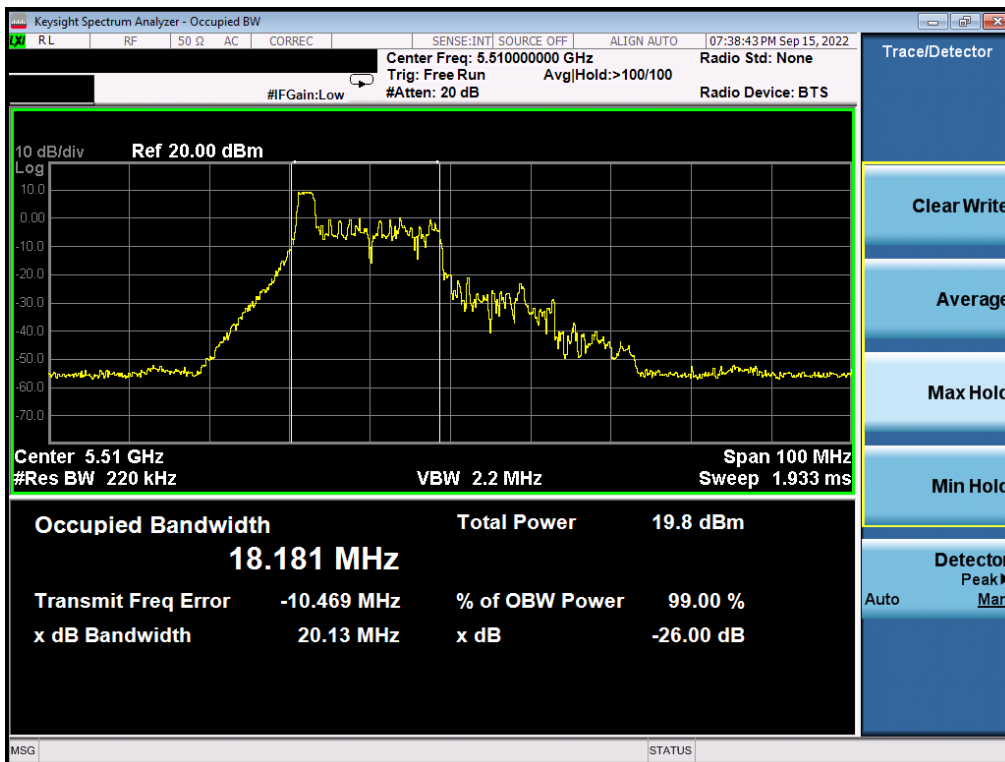
Plot 7-66. 26dB Bandwidth Plot MIMO ANT2 (40MHz BW 802.11ax – 26 Tones (UNII Band 2C) – Ch. 102)
