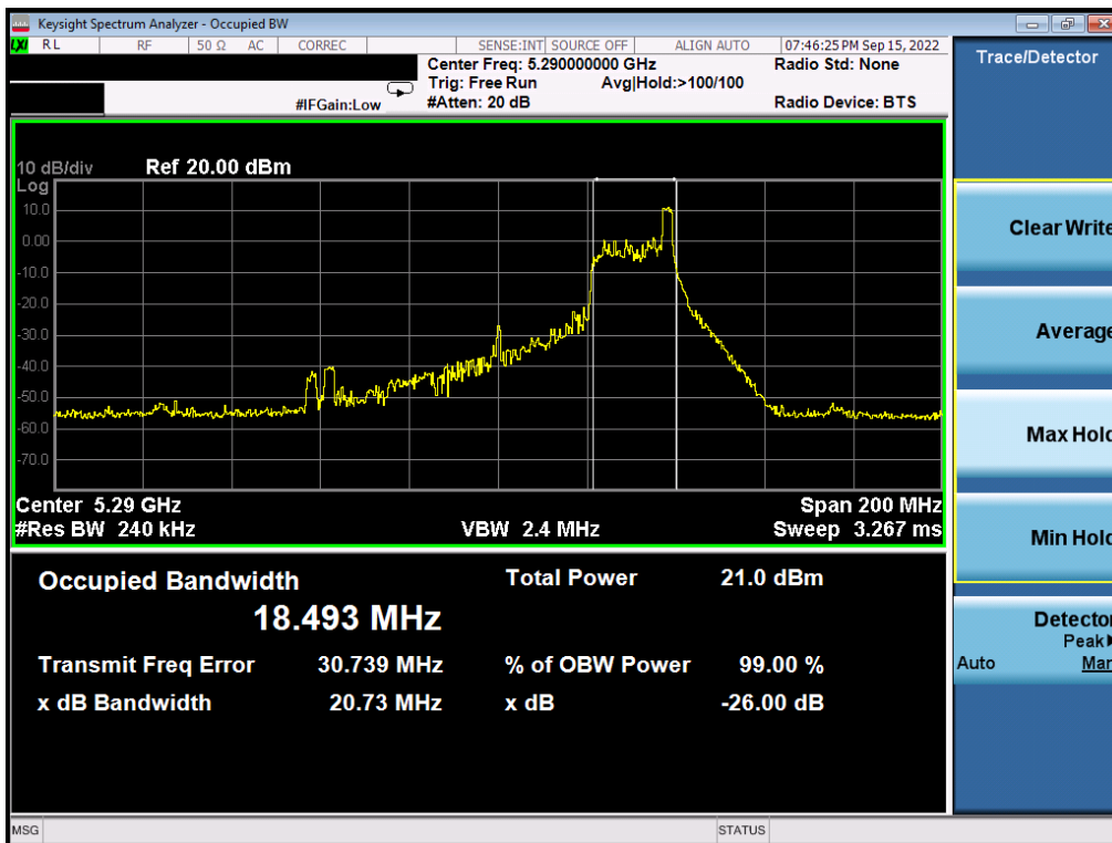
Plot 7-62. 26dB Bandwidth Plot MIMO ANT2 (80MHz BW 802.11ax – 26 Tones (UNII Band 2A) – Ch. 58)
