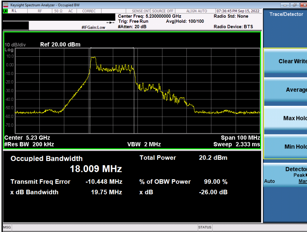
Plot 7-53. 26dB Bandwidth Plot MIMO ANT2 (40MHz BW 802.11ax – 26 Tones (UNII Band 1) – Ch. 46)
