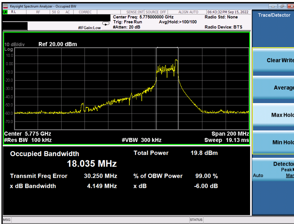
Plot 7-102. 6dB Bandwidth Plot SISO ANT1 (80MHz BW 802.11ax – 26 Tones (UNII Band 3) – Ch. 155)
