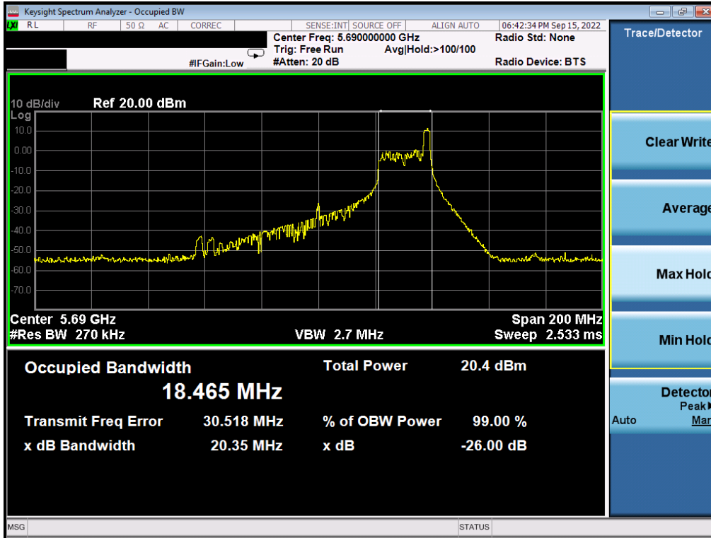
Plot 7-23. 26dB Bandwidth Plot MIMO ANT1 (80MHz BW 802.11ax – 26 Tones (UNII Band 2C) – Ch. 138)
