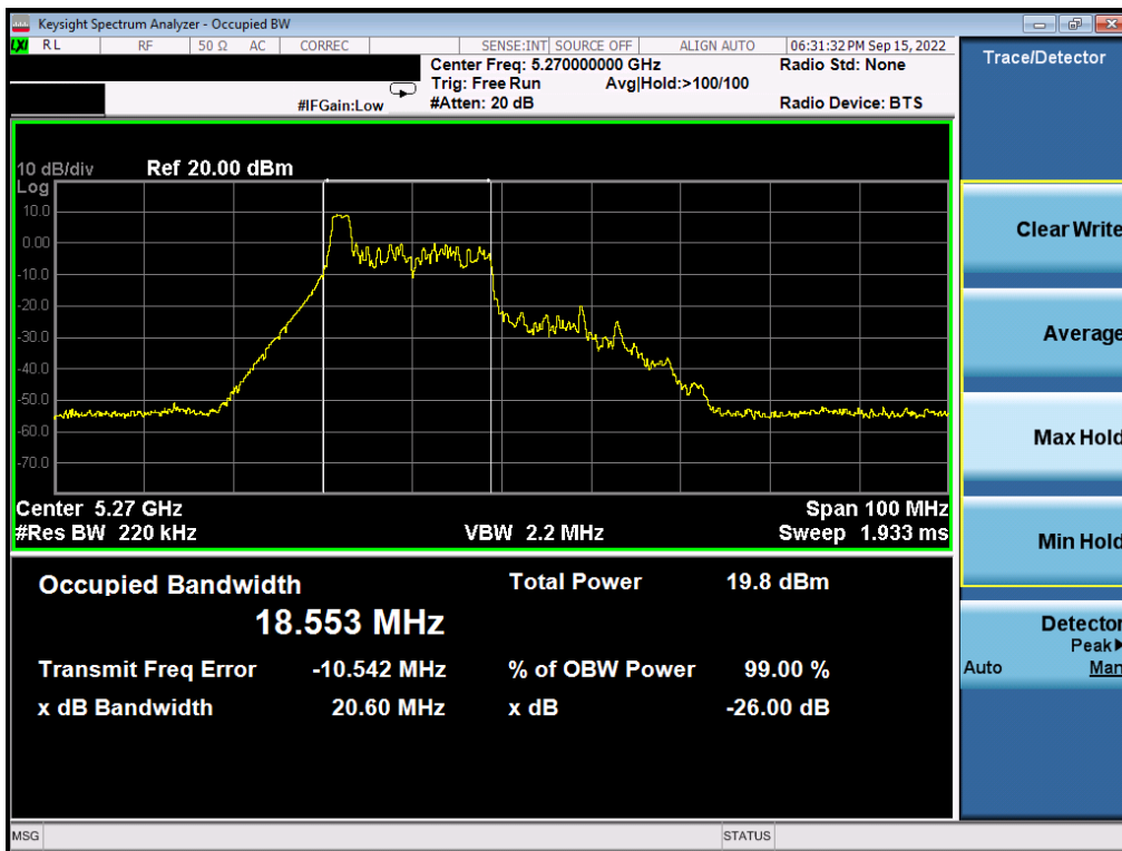
Plot 7-12. 26dB Bandwidth Plot MIMO ANT1 (40MHz BW 802.11ax – 26 Tones (UNII Band 2A) – Ch. 54)
