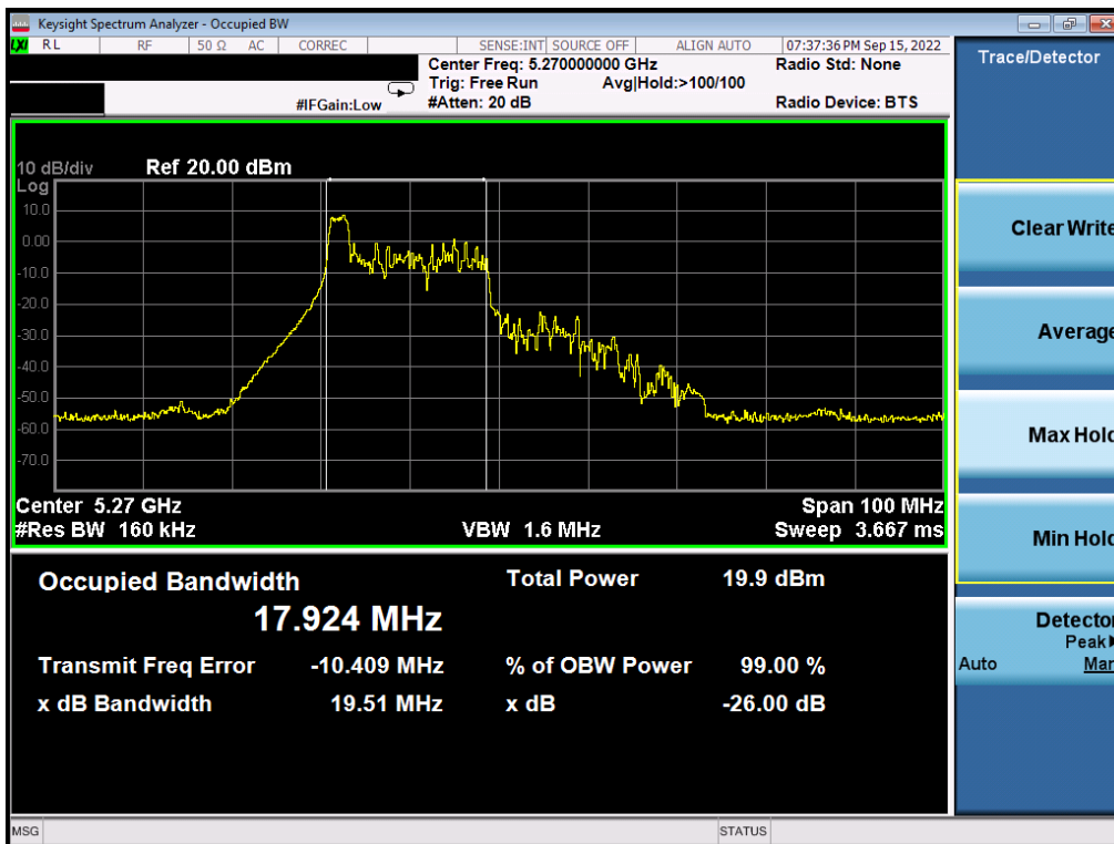
Plot 7-60. 26dB Bandwidth Plot MIMO ANT2 (40MHz BW 802.11ax – 26 Tones (UNII Band 2A) – Ch. 54)
