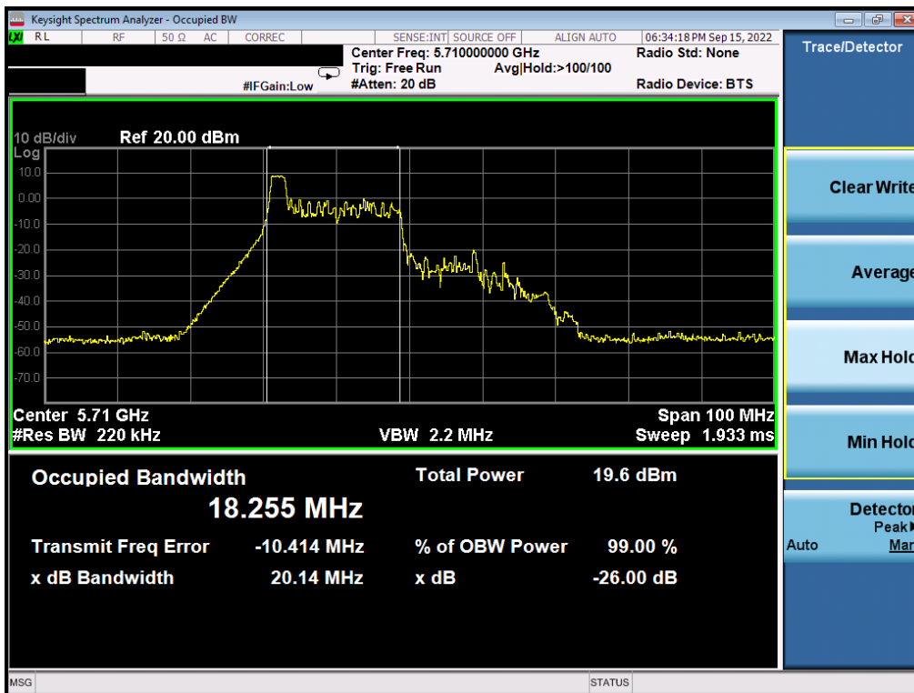
Plot 7-20. 26dB Bandwidth Plot MIMO ANT1 (40MHz BW 802.11ax – 26 Tones (UNII Band 2C) – Ch. 142)
