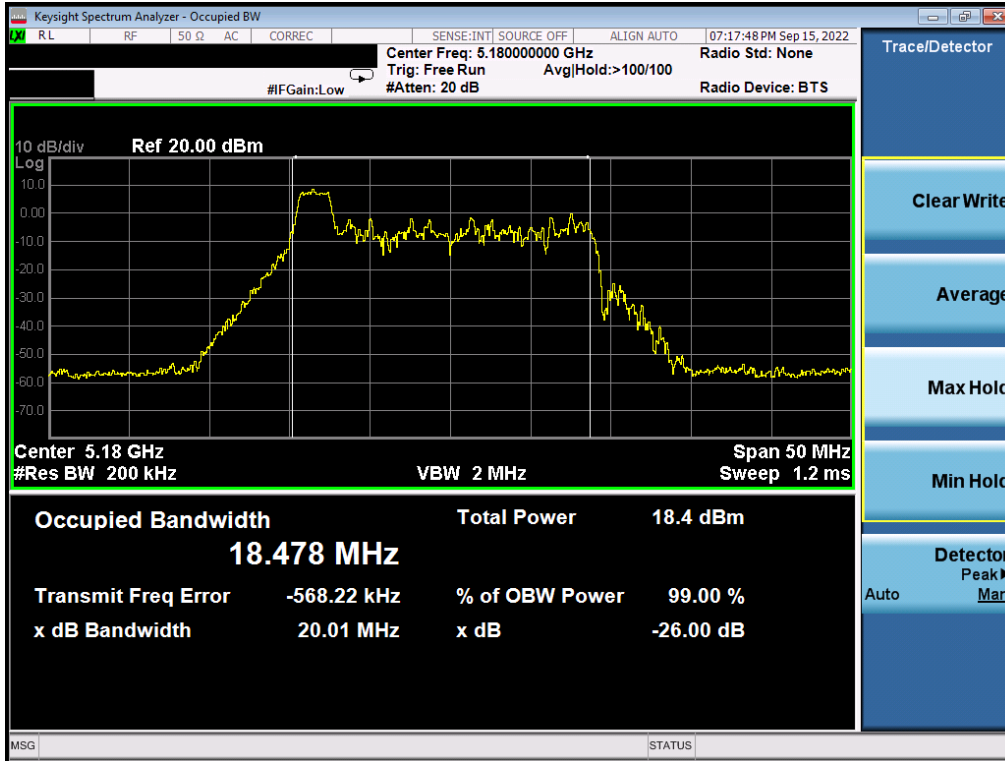
Plot 7-49. 26dB Bandwidth Plot MIMO ANT2 (20MHz BW 802.11ax – 26 Tones (UNII Band 1) – Ch. 36)
