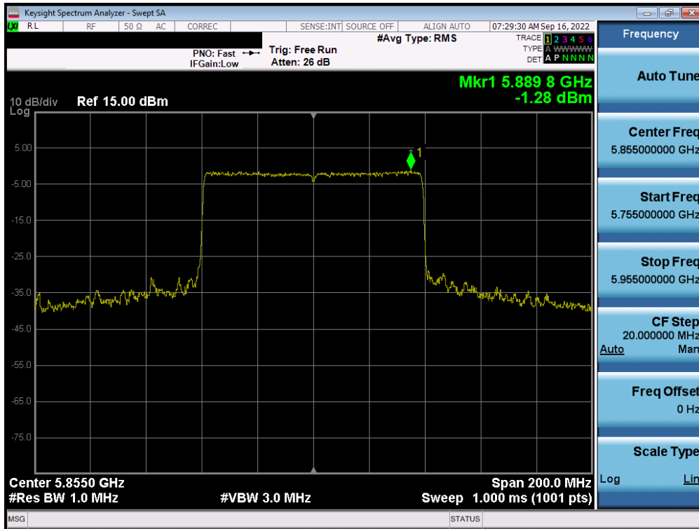
Plot 7-259. Power Spectral Density Plot MIMO ANT1 (80MHz BW 802.11ax (UNII Band 3/4) – Ch. 171)
