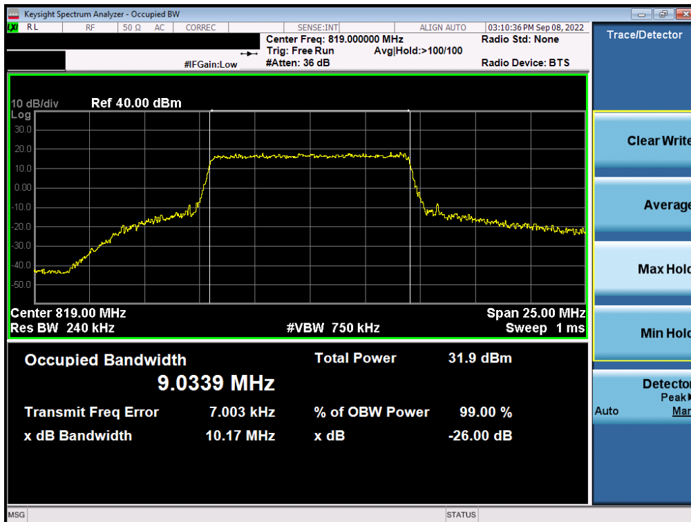
Plot 7-4. Occupied Bandwidth Plot (LTE Band 26 - 10MHz 16-QAM - Full RB)
