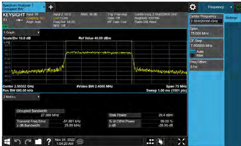
Plot 7-32. Occupied Bandwidth Plot (NR Band n41(PC3) - 30MHz 16-QAM - Full RB)
