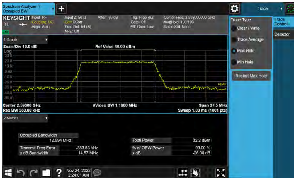
Plot 7-36. Occupied Bandwidth Plot (NR Band n41(PC3) - 15MHz \pi/2 BPSK - Full RB)
