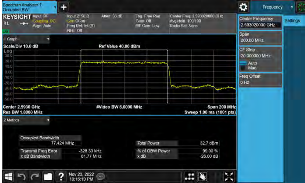
Plot 7-15. Occupied Bandwidth Plot (NR Band n41(PC3) - 80MHz \pi/2 BPSK - Full RB)
