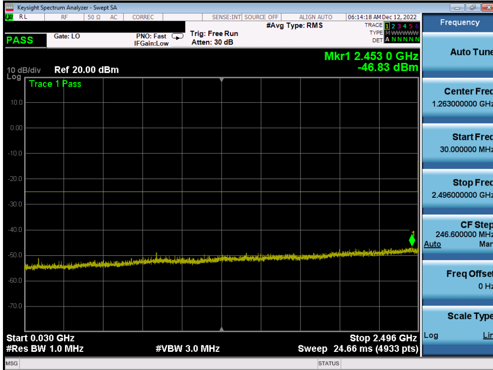
Plot 7-48. Conducted Spurious Plot (LTE Band 41(PC3) - 20MHz QPSK - RB Size 1, RB Offset 0 - High Channel - Ant1)
