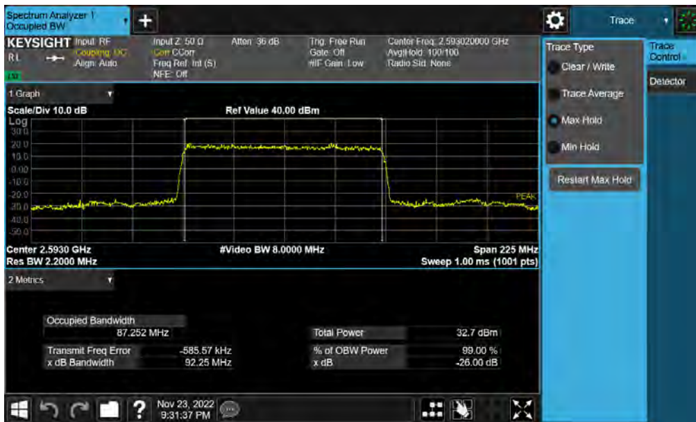
Plot 7-12. Occupied Bandwidth Plot (NR Band n41(PC3) - 90MHz \pi/2 BPSK - Full RB)
