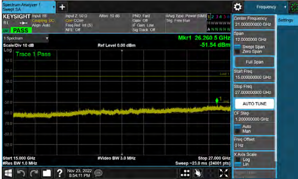
Plot 7-53. Conducted Spurious Plot (NR Band n41(PC3) - 100MHz QPSK - RB Size 1, RB Offset 0 - Low Channel Ant1)
