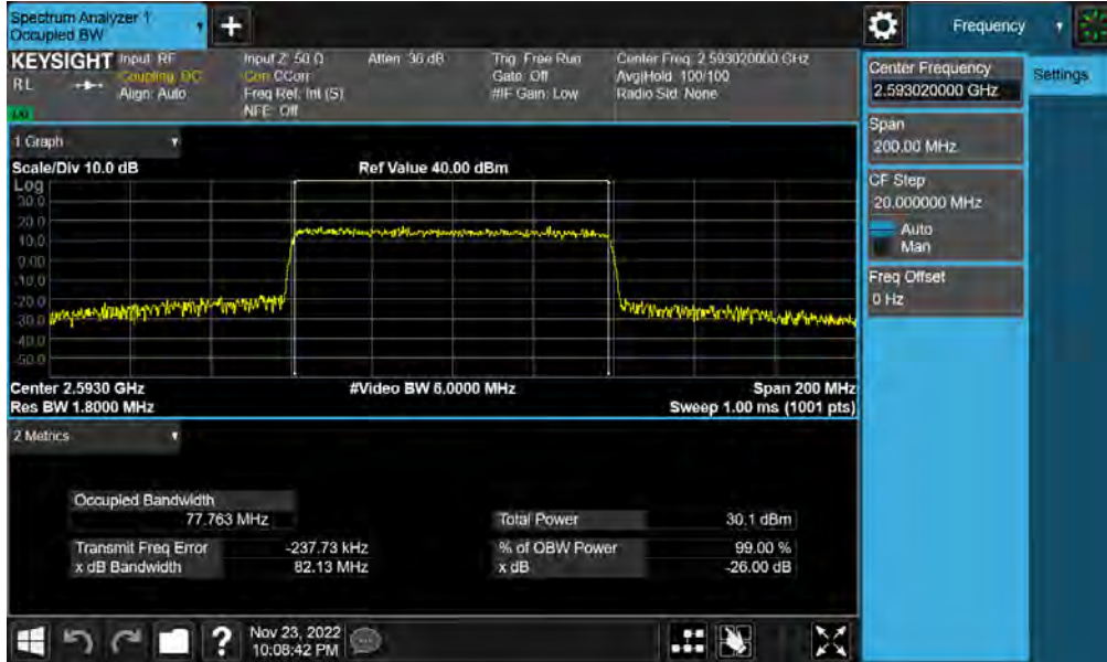
Plot 7-17. Occupied Bandwidth Plot (NR Band n41(PC3) - 80MHz 16-QAM - Full RB)
