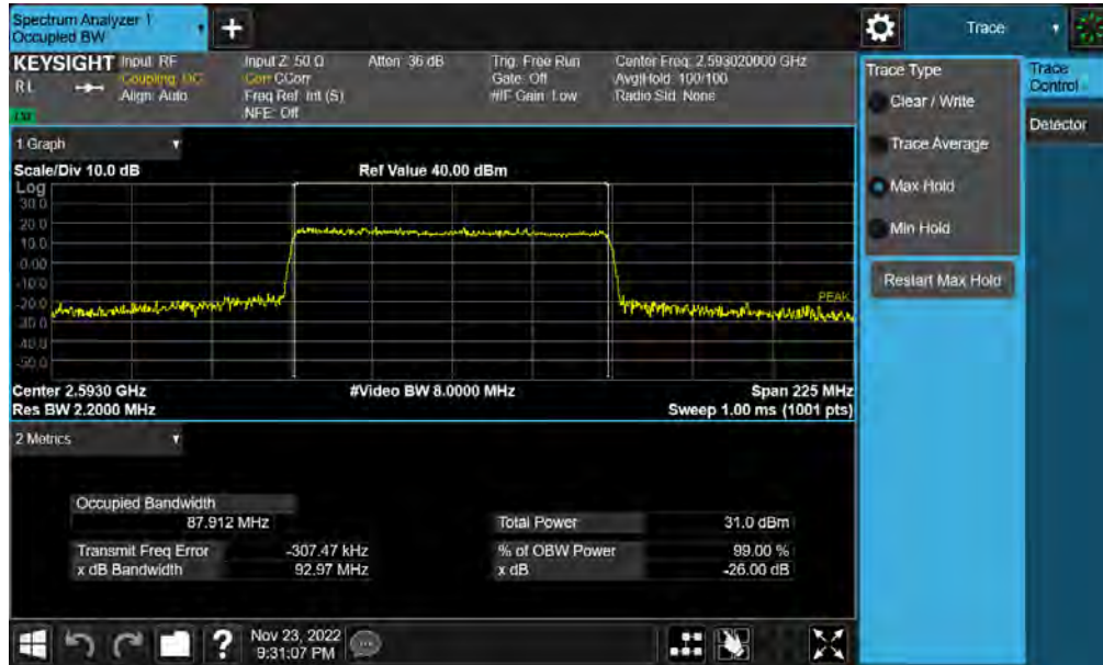
Plot 7-13. Occupied Bandwidth Plot (NR Band n41(PC3) - 90MHz QPSK - Full RB)
