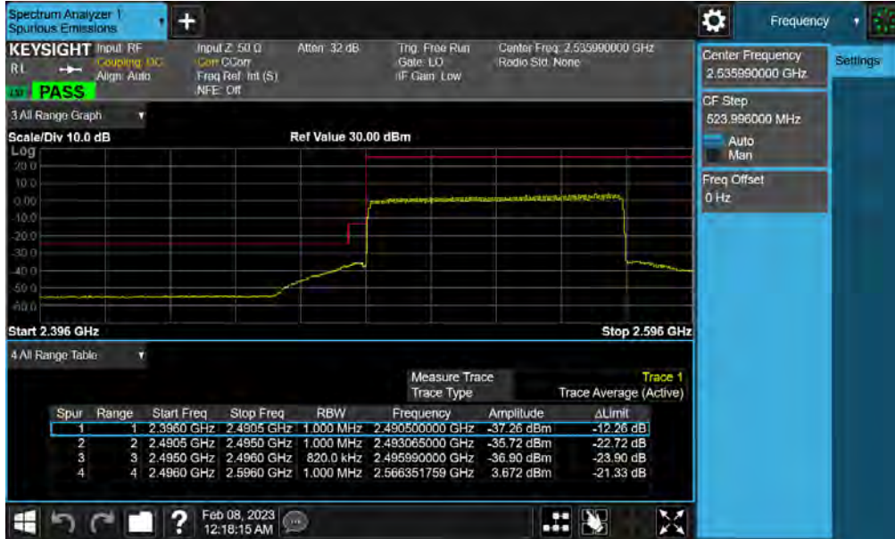
Plot 7-84. Lower ACP Plot (NR Band n41(PC3) - 80MHz CP-OFDM-QPSK – Full RB)
