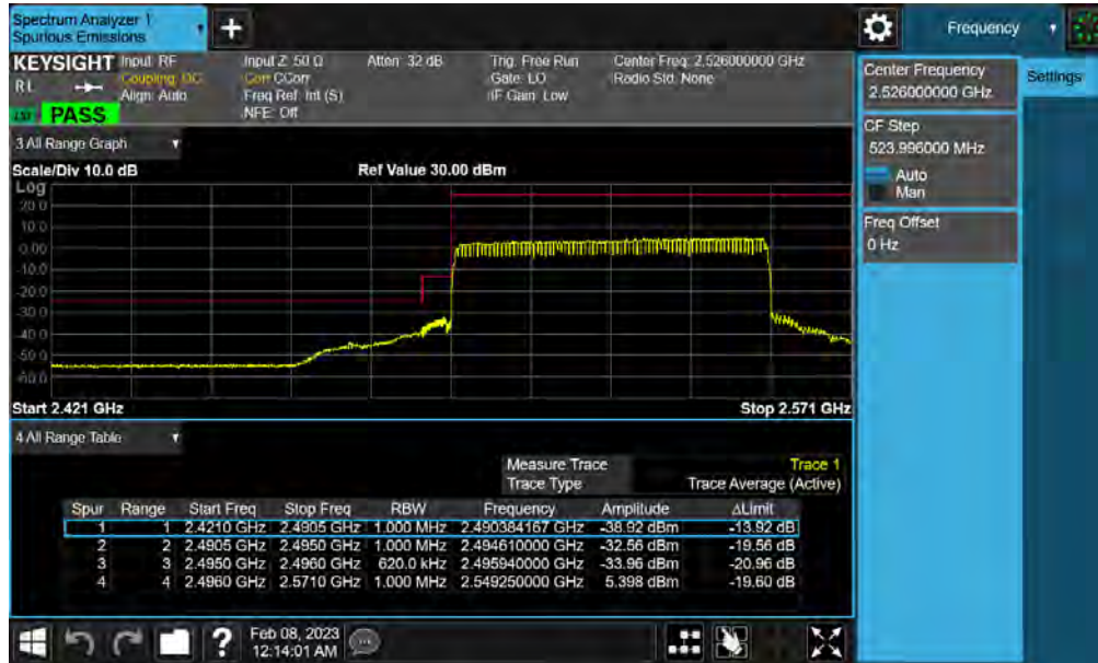
Plot 7-88. Lower ACP Plot (NR Band n41(PC3) - 60MHz CP-OFDM-QPSK – Full RB)
