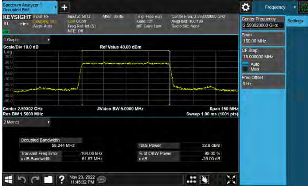
Plot 7-21. Occupied Bandwidth Plot (NR Band n41(PC3) - 60MHz \pi/2 BPSK - Full RB)
