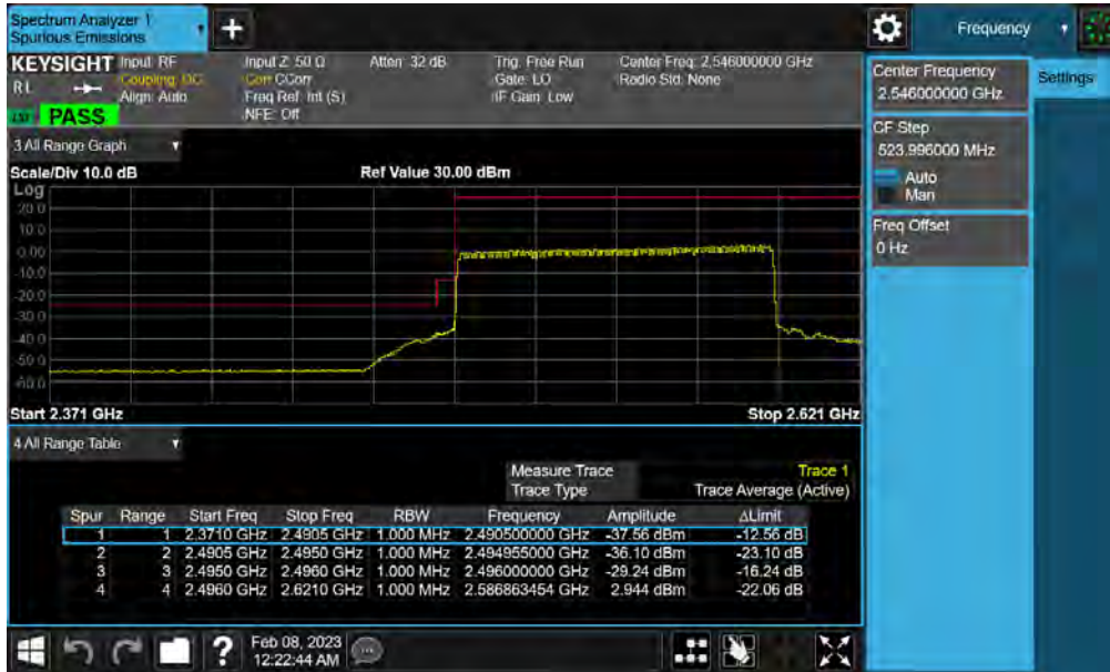
Plot 7-80. Lower ACP Plot (NR Band n41(PC3) - 100MHz CP-OFDM-QPSK – Full RB)
