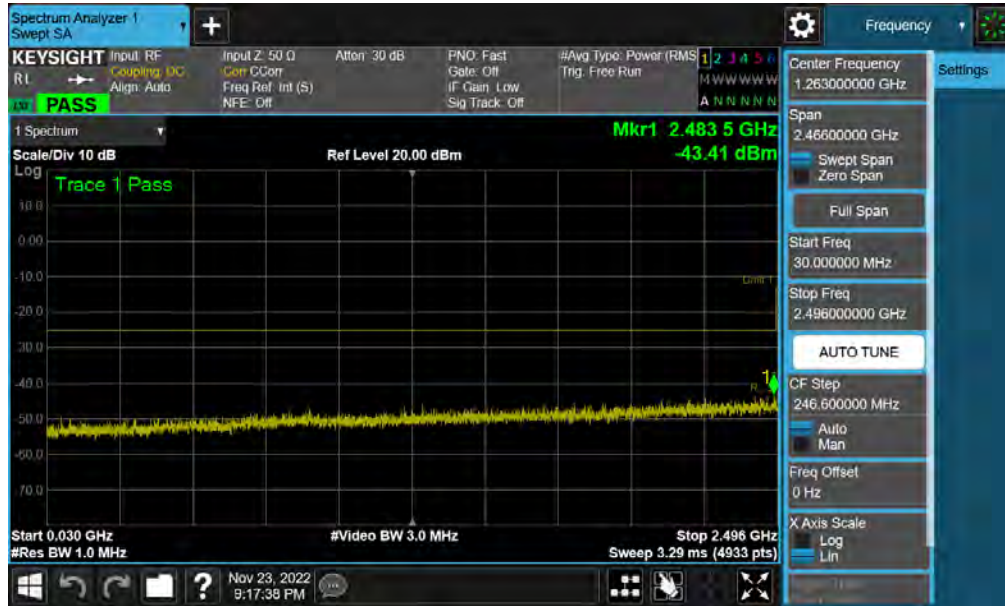
Plot 7-57. Conducted Spurious Plot (NR Band n41(PC3) - 100MHz QPSK - RB Size 1, RB Offset 0 - High Channel Ant1)
