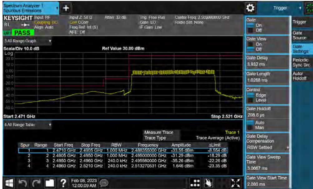
Plot 7-94. Lower ACP Plot (NR Band n41(PC3) - 20MHz CP-OFDM-QPSK – Full RB)
