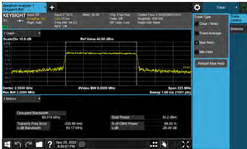
Plot 7-14. Occupied Bandwidth Plot (NR Band n41(PC3) - 90MHz 16-QAM - Full RB)
