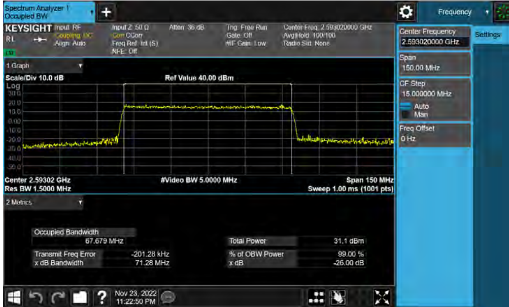
Plot 7-19. Occupied Bandwidth Plot (NR Band n41(PC3) - 70MHz QPSK - Full RB)
