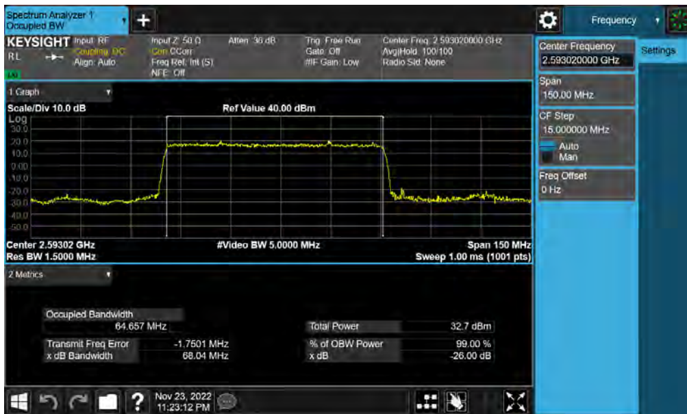
Plot 7-18. Occupied Bandwidth Plot (NR Band n41(PC3) - 70MHz \pi/2 BPSK - Full RB)
