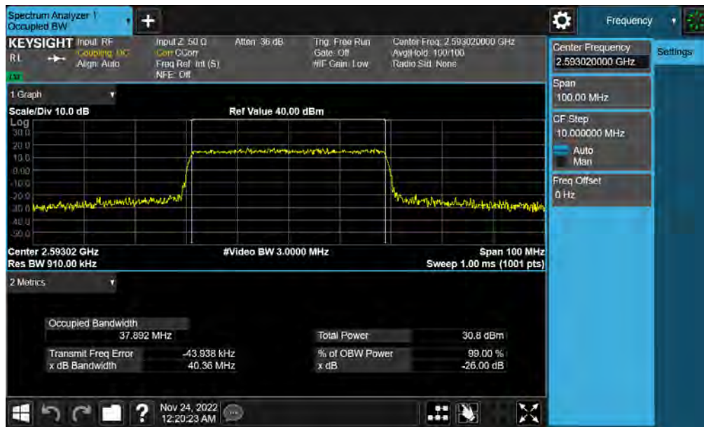
Plot 7-28. Occupied Bandwidth Plot (NR Band n41(PC3) - 40MHz QPSK - Full RB)
