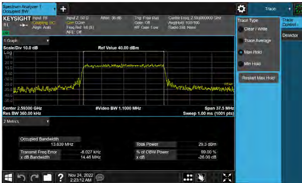
Plot 7-38. Occupied Bandwidth Plot (NR Band n41(PC3) - 15MHz 16-QAM - Full RB)
