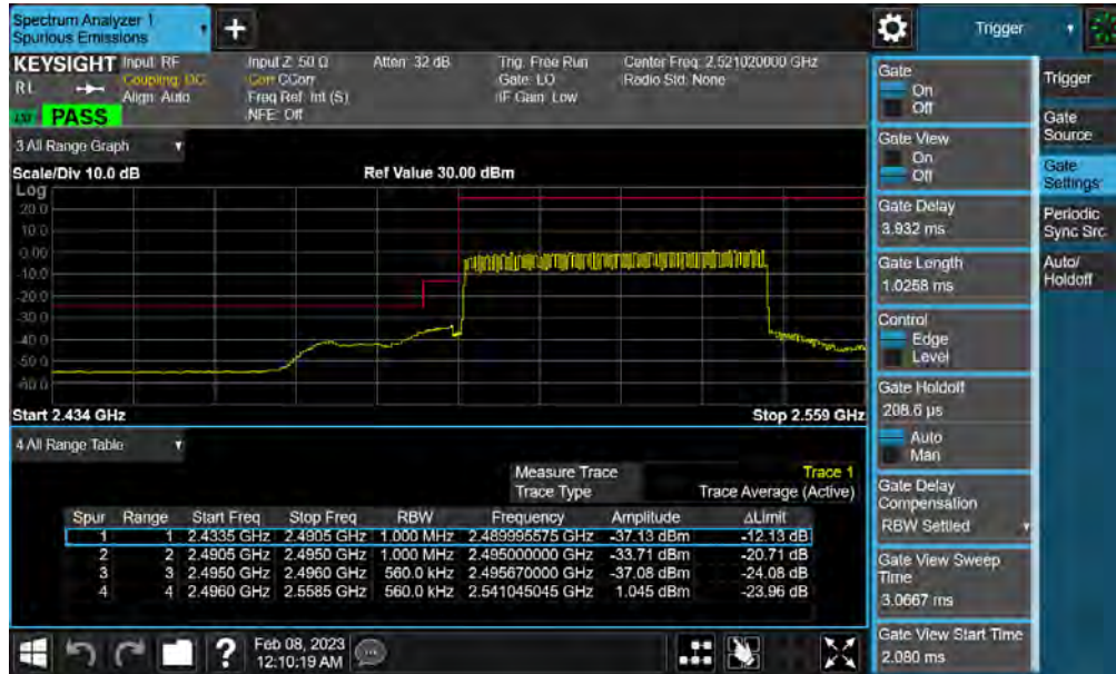
Plot 7-90. Lower ACP Plot (NR Band n41(PC3) - 50MHz CP-OFDM-QPSK – Full RB)
