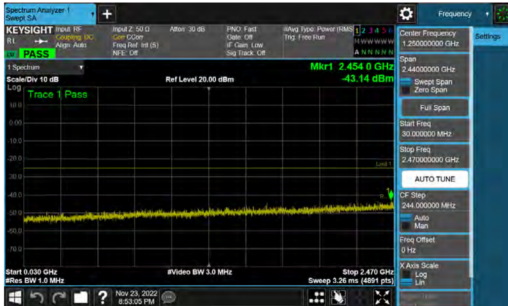
Plot 7-51. Conducted Spurious Plot (NR Band n41(PC3) - 100MHz QPSK - RB Size 1, RB Offset 0 - Low Channel Ant1)
