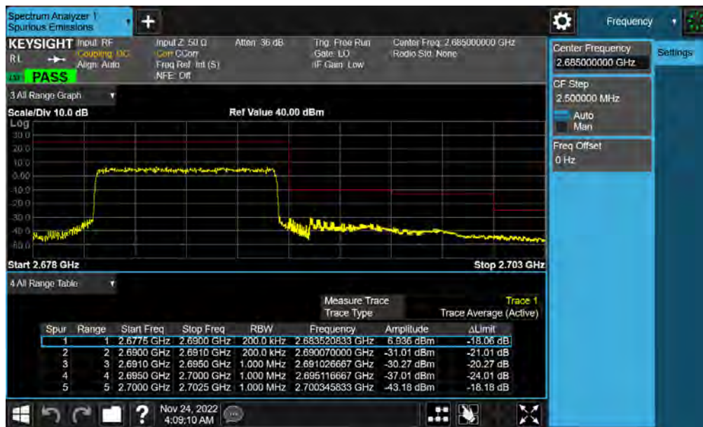
Plot 7-99. Upper ACP Plot (NR Band n41(PCI3) - 10MHz CP-OFDM-QPSK – Full RB)
