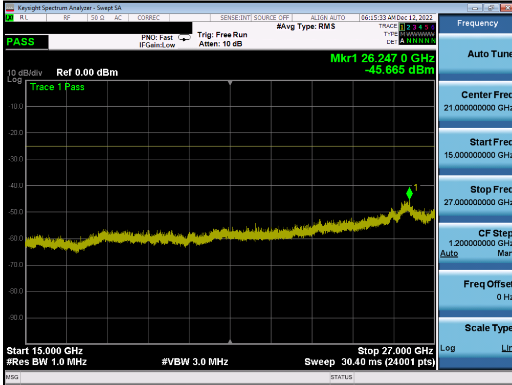
Plot 7-50. Conducted Spurious Plot (LTE Band 41(PC3) - 20MHz QPSK - RB Size 1, RB Offset 0 - High Channel - Ant1)
