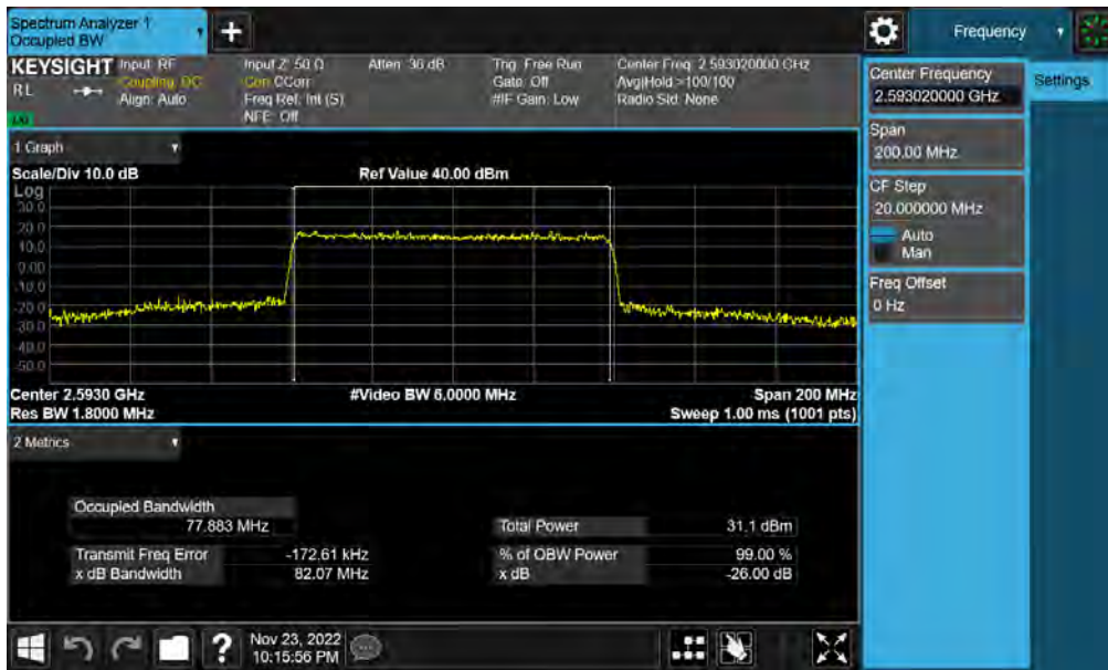
Plot 7-16. Occupied Bandwidth Plot (NR Band n41(PC3) - 80MHz QPSK - Full RB)
