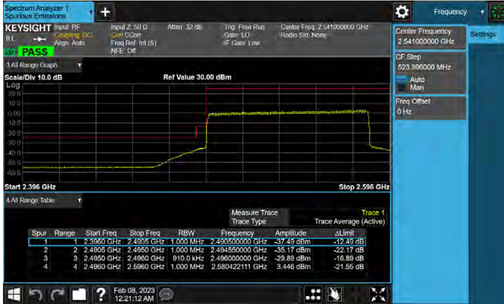
Plot 7-82. Lower ACP Plot (NR Band n41(PC3) - 90MHz CP-OFDM-QPSK – Full RB)
