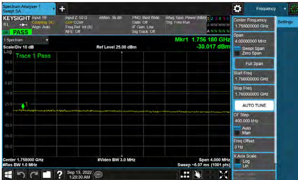
Plot 7-65. Upper Extended Band Edge Plot (LTE Band 4 - 20MHz QPSK – Full RB)
