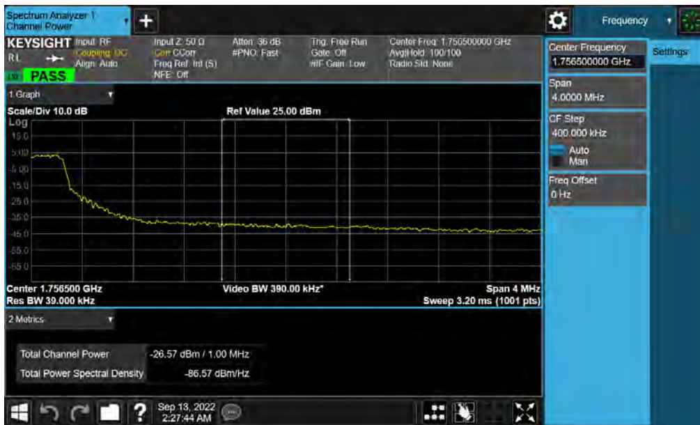
Plot 7-83. Upper Extended Band Edge Plot (LTE Band 4 - 5MHz QPSK – Full RB)
