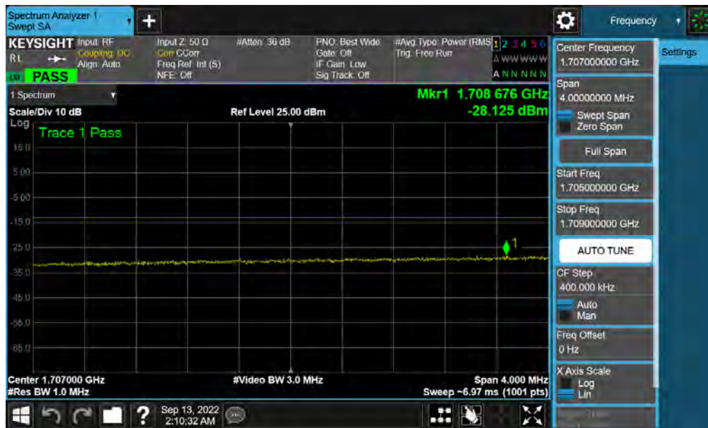
Plot 7-69. Lower Extended Band Edge Plot (LTE Band 66/4 - 15MHz QPSK – Full RB)
