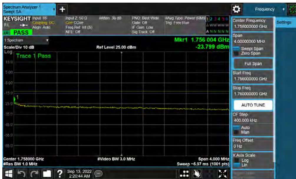
Plot 7-77. Upper Extended Band Edge Plot (LTE Band 4 - 10MHz QPSK – Full RB)
