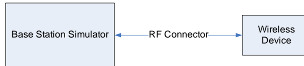
Figure 9-3 Power Measurement Setup
