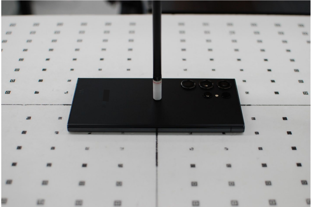
Figure G-14 Near Field Power Density Test Setup Photo – Back Side at 2 mm
