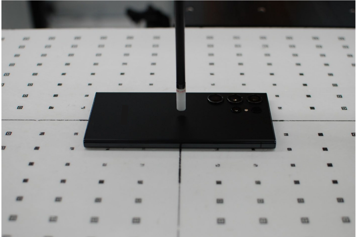
Figure G-15 Near Field Power Density Test Setup Photo – Back Side at 9.24 mm
