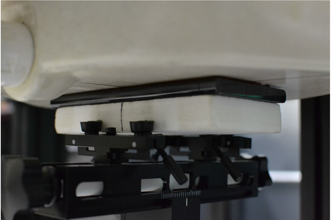
Figure G-8 SAR Test Setup Photo– Phablet, Back Side, 0 mm
