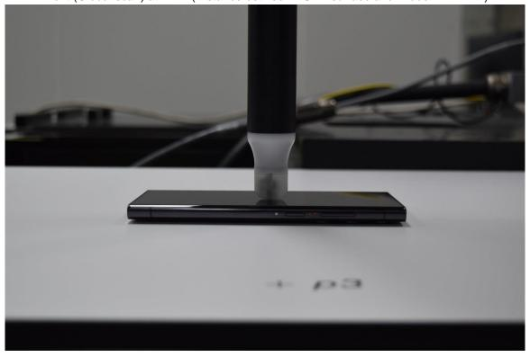
Front (Local scan with Spen) at 7mm (Distance between DUT's surface and Probe's element)
