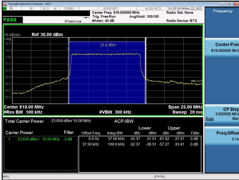
Plot 7-54. Channel Edge Plot (NR Band n26 - 10MHz DFT-s QPSK - Mid Channel)
