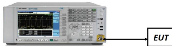
Figure 7-2. Test Instrument & Measurement Setup
