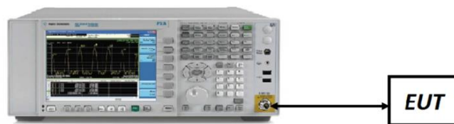
Figure 7-4. Test Instrument & Measurement Setup
