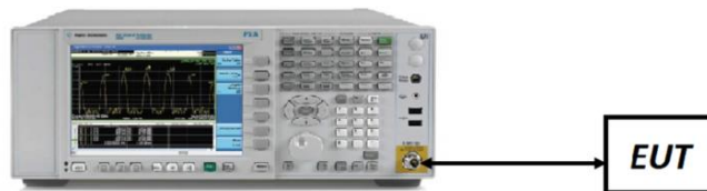
Figure 7-5. Test Instrument & Measurement Setup
