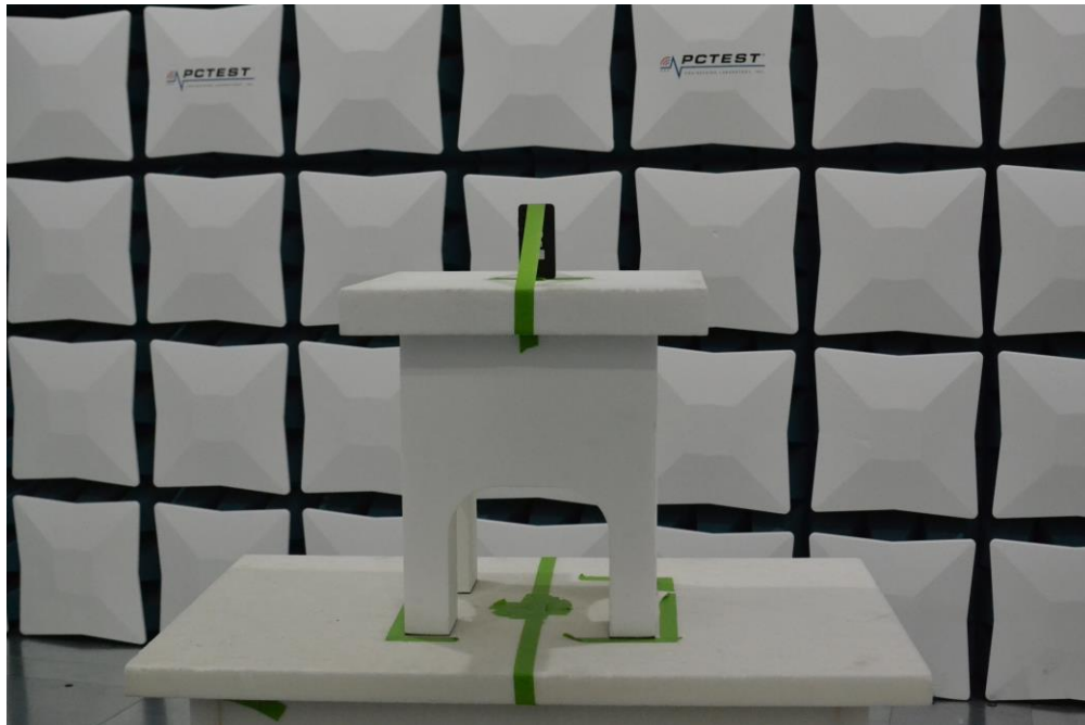
Figure 6. Test Setup – Z Position – 1GHz-18GHz
