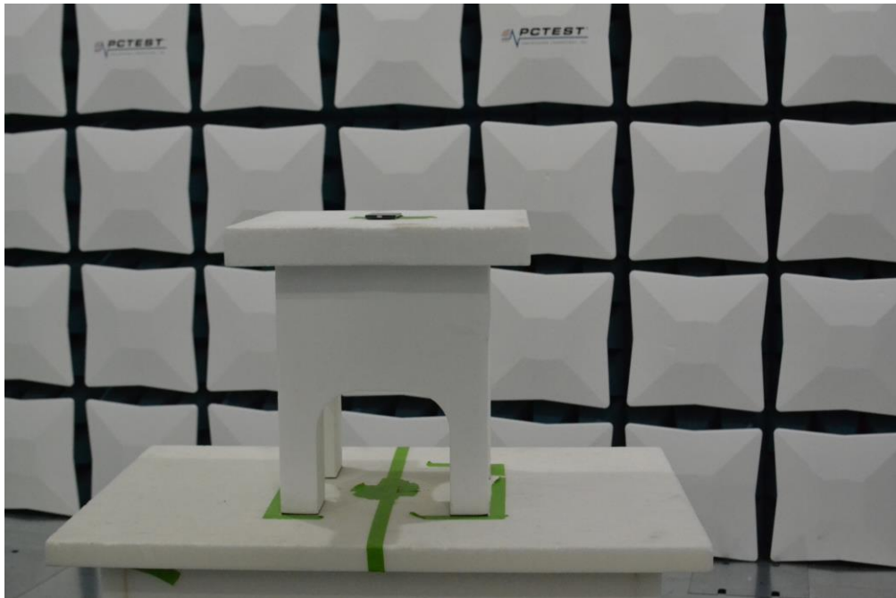
Figure 2. Test Setup – X Position – 1GHz-18GHz
