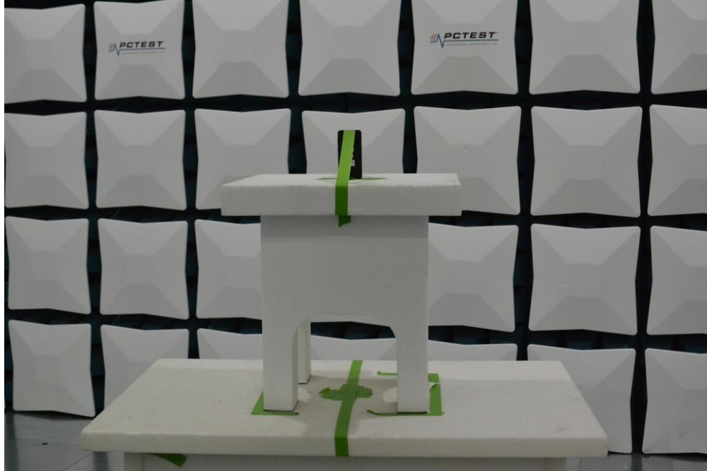
Figure 5. Test Setup – Z Position – 1GHz-18GHz
