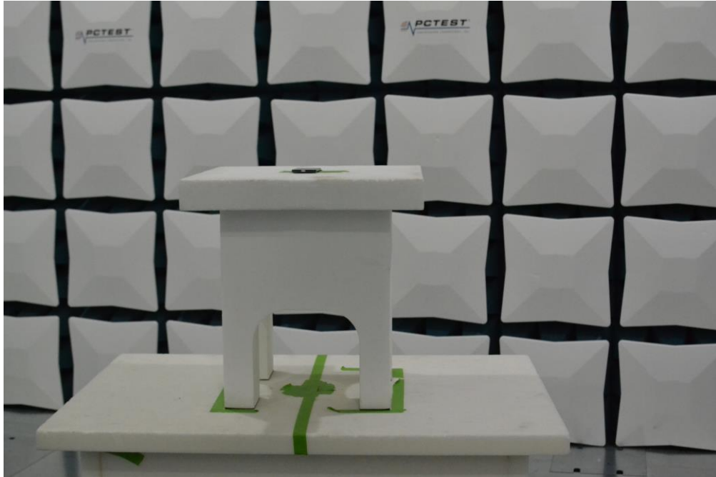
Figure 1. Test Setup – X Position – 1GHz-18GHz
