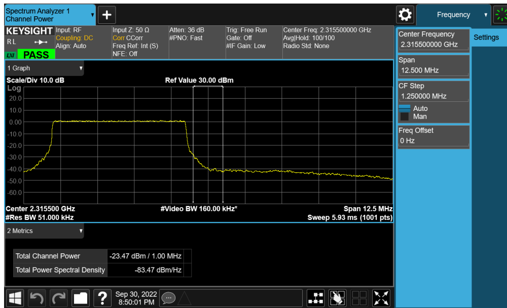
Plot 7-401. Upper Band Edge Plot (NR Band n30 - 5MHz CP-OFDM-QPSK – Full RB - Ant F)
