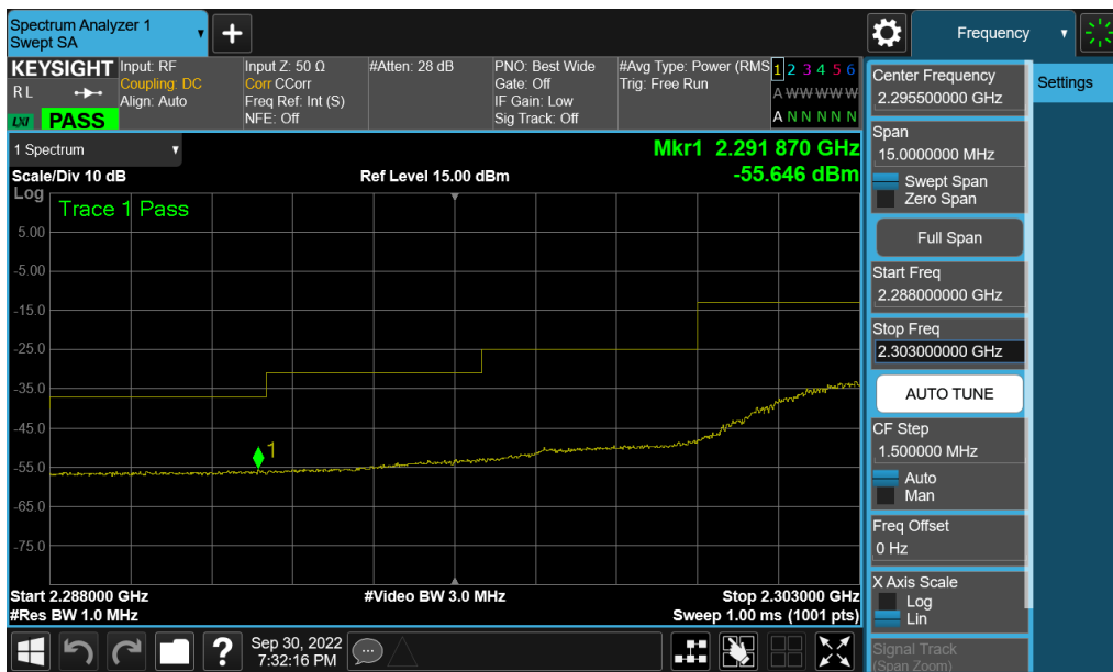
Plot 7-390. Extended Lower Band Edge Plot (NR Band n30 - 5MHz CP-OFDM-QPSK – Full RB - Ant A)
