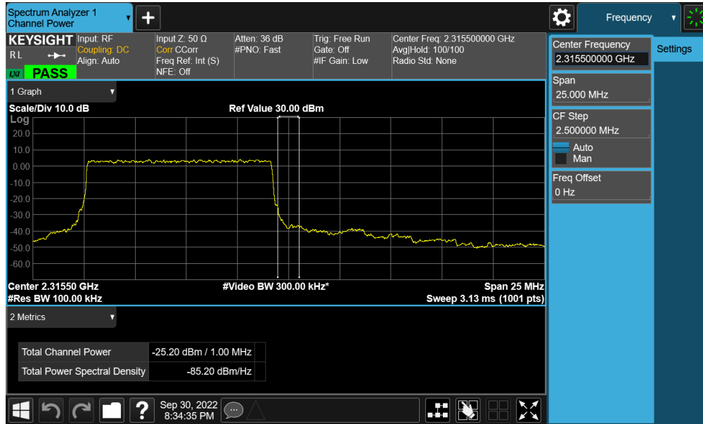
Plot 7-396. Upper Band Edge Plot (NR Band n30 - 10MHz CP-OFDM-QPSK – Full RB - Ant F)
