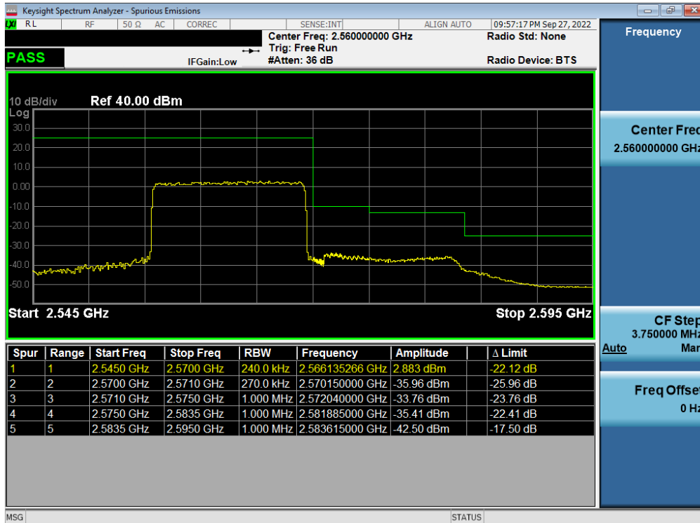
Plot 7-356. Upper ACP Plot (LTE Band 7 - 15MHz QPSK - Full RB - Ant B)
