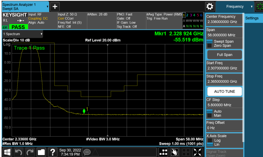
Plot 7-393. Extended Upper Band Edge Plot (NR Band n30 - 5MHz CP-OFDM-QPSK – Full RB - Ant A)
