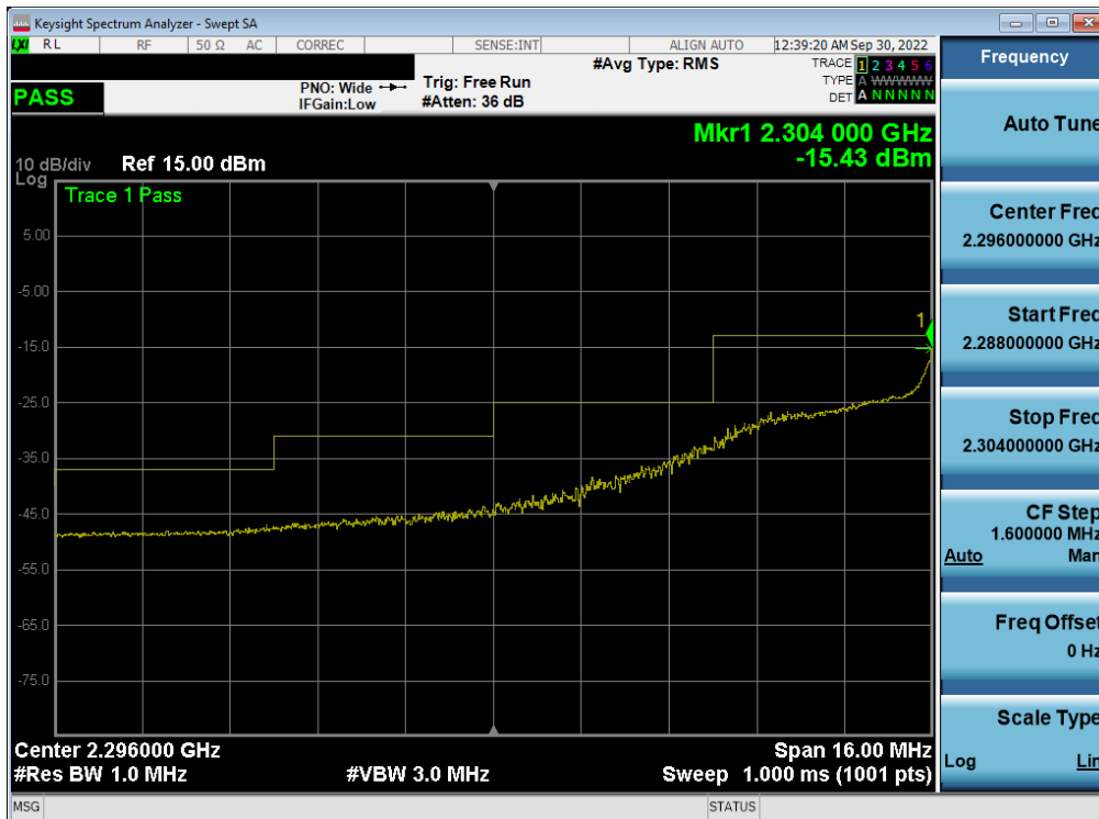
Plot 7-350. Extended Lower Band Edge Plot (LTE Band 30 - 5MHz QPSK – Full RB - Ant F)
