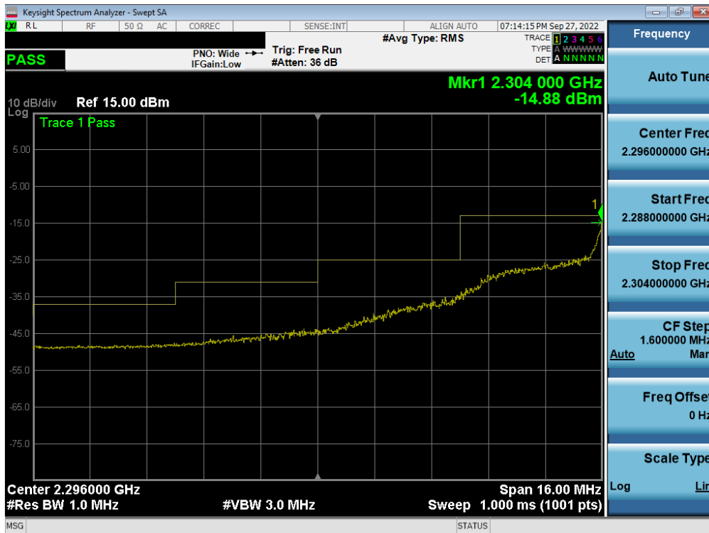
Plot 7-342. Extended Lower Band Edge Plot (LTE Band 30 - 5MHz QPSK – Full RB - Ant A)
