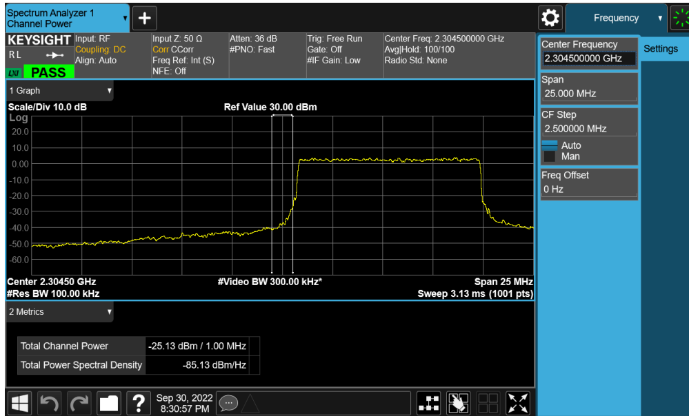
Plot 7-394. Lower Band Edge Plot (NR Band n30 - 10MHz CP-OFDM-QPSK – Full RB - Ant F)
