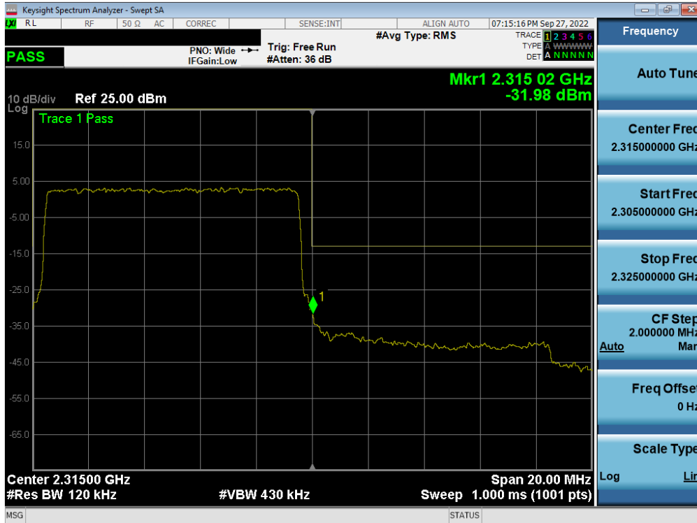
Plot 7-339. Upper Band Edge Plot (LTE Band 30 - 10MHz QPSK – Full RB - Ant A)
