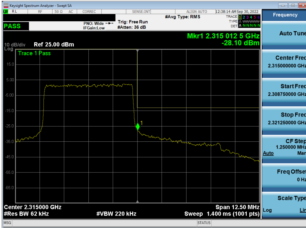
Plot 7-351. Upper Band Edge Plot (LTE Band 30 - 5MHz QPSK – Full RB - Ant F)
