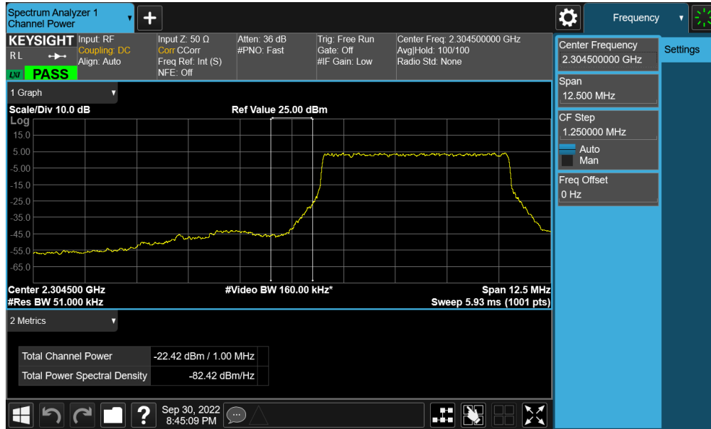
Plot 7-398. Lower Band Edge Plot (NR Band n30 - 5MHz CP-OFDM-QPSK – Full RB - Ant F)
