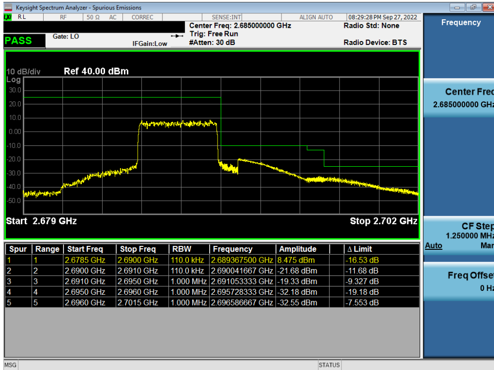
Plot 7-376. Upper ACP Plot (LTE Band 41(PC2) - 5MHz QPSK - Full RB - Ant B)
