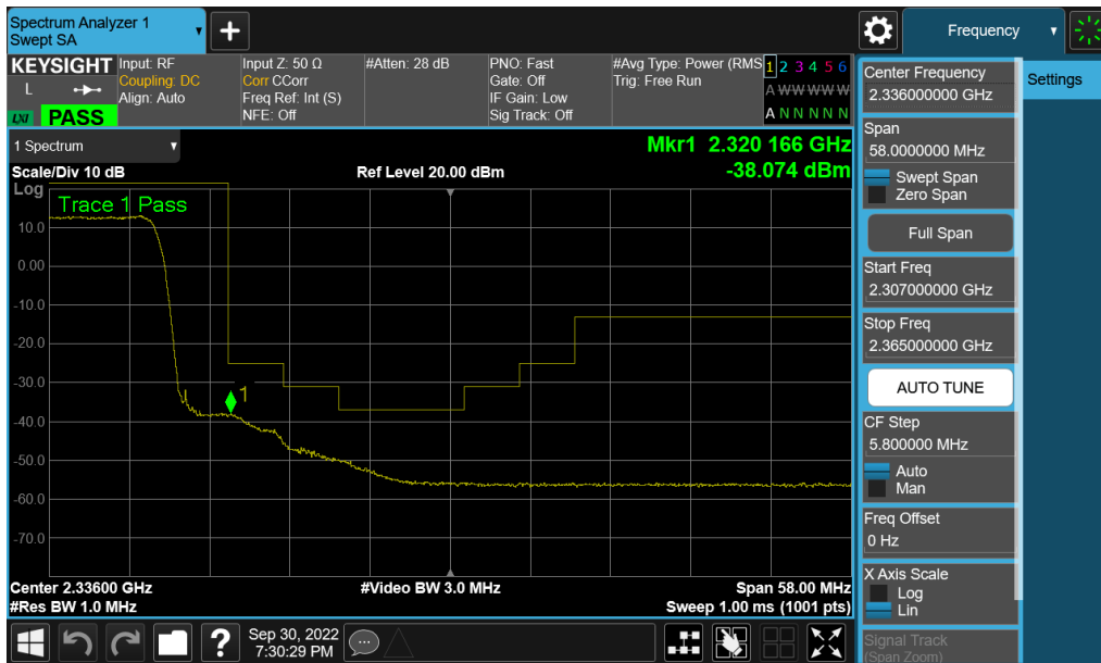
Plot 7-388. Extended Upper Band Edge Plot (NR Band n30 - 10MHz CP-OFDM-QPSK – Full RB - Ant A)
