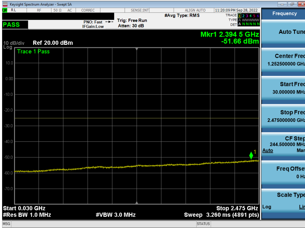
Plot 7-196. Conducted Spurious Plot (LTE Band 7 - 20MHz QPSK - RB Size 1, RB Offset 0 - Low Channel - Ant F)
