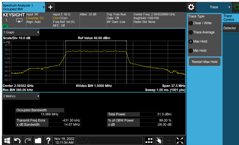
Plot 7-177. Occupied Bandwidth Plot (NR Band n41 - 15MHz 16-QAM - Full RB - Switching - Ant B)
