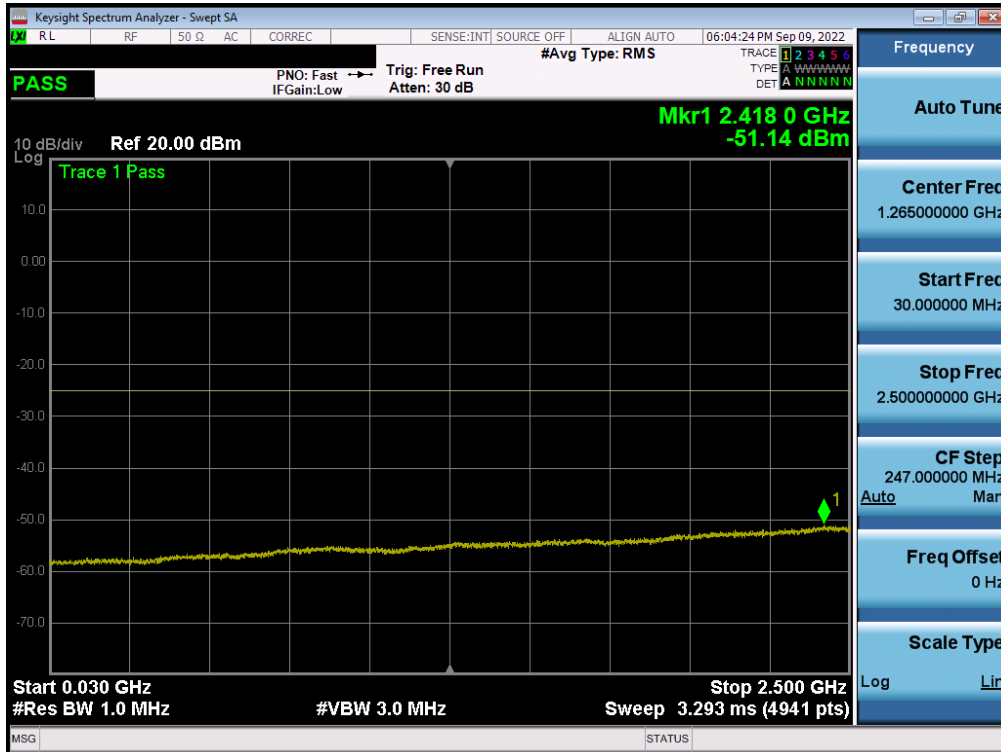
Plot 7-193. Conducted Spurious Plot (LTE Band 7 - 20MHz QPSK - RB Size 1, RB Offset 0 - High Channel - Ant B)
