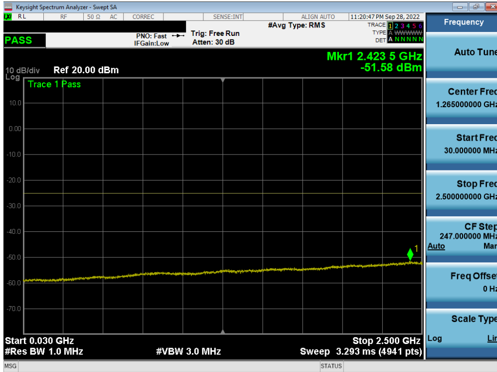
Plot 7-202. Conducted Spurious Plot (LTE Band 7 - 20MHz QPSK - RB Size 1, RB Offset 0 - High Channel - Ant F)
