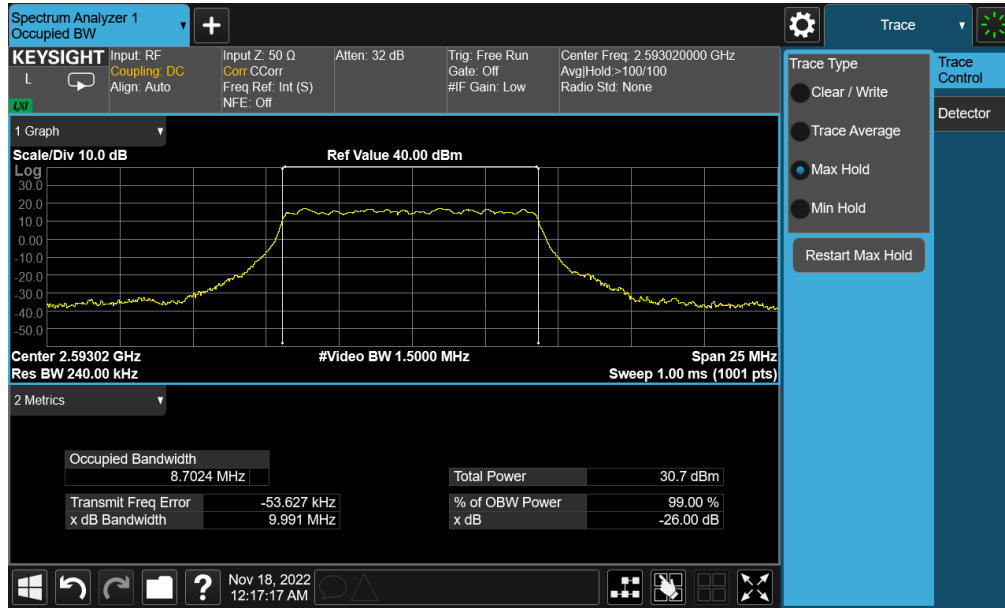
Plot 7-180. Occupied Bandwidth Plot (NR Band n41 - 10MHz 16-QAM - Full RB - Switching - Ant B)
