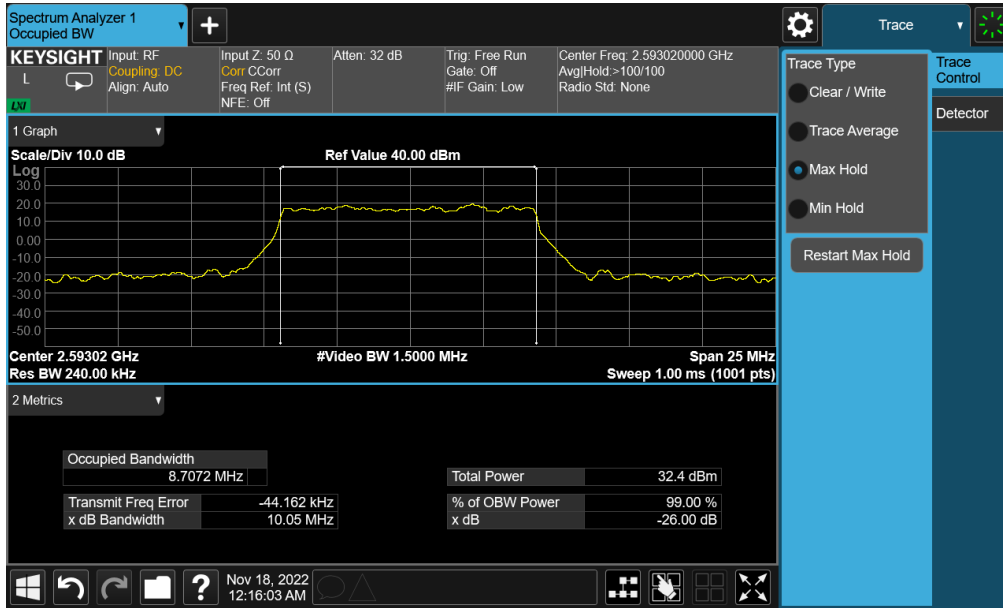
Plot 7-178. Occupied Bandwidth Plot (NR Band n41 - 10MHz \pi/2 BPSK - Full RB - Switching - Ant B)
