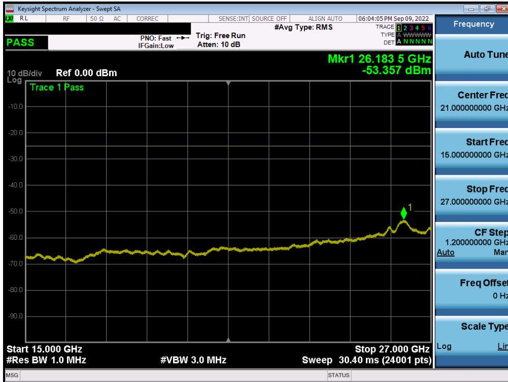
Plot 7-189. Conducted Spurious Plot (LTE Band 7 - 20MHz QPSK - RB Size 1, RB Offset 0 - Low Channel - Ant B)
