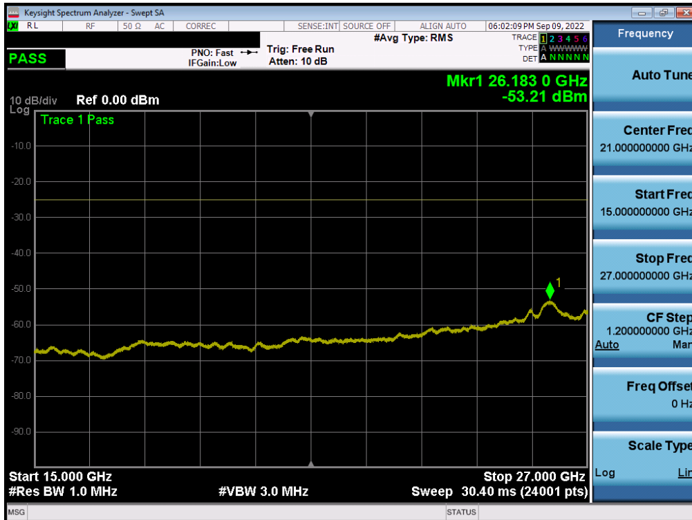
Plot 7-192. Conducted Spurious Plot (LTE Band 7 - 20MHz QPSK - RB Size 1, RB Offset 0 - Mid Channel - Ant B)
