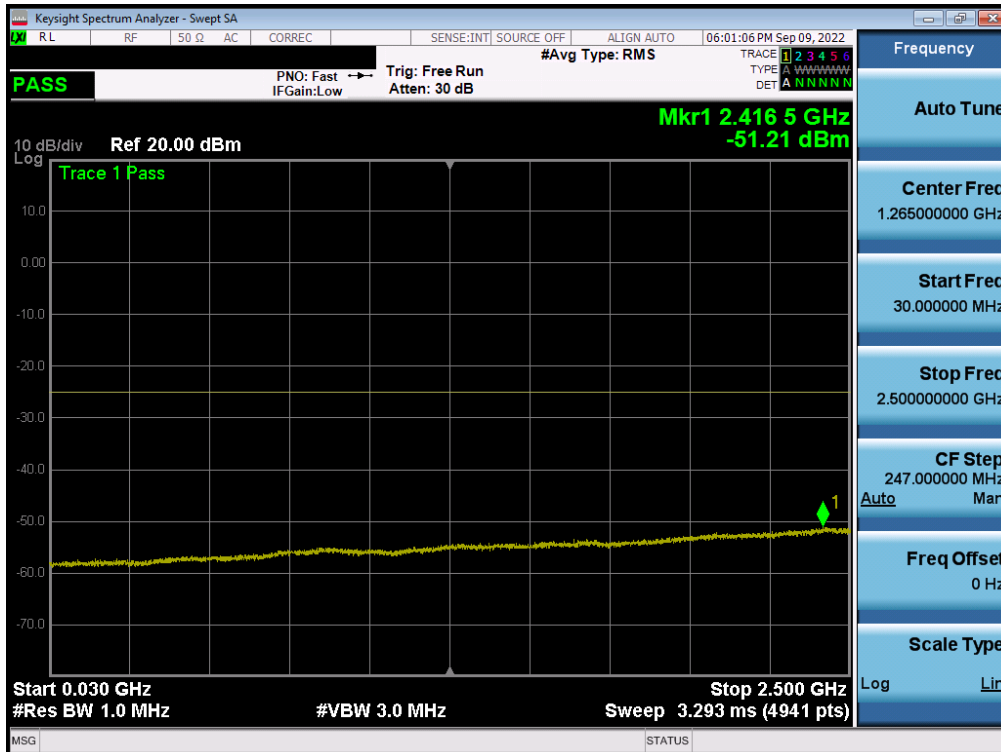
Plot 7-190. Conducted Spurious Plot (LTE Band 7 - 20MHz QPSK - RB Size 1, RB Offset 0 - Mid Channel - Ant B)
