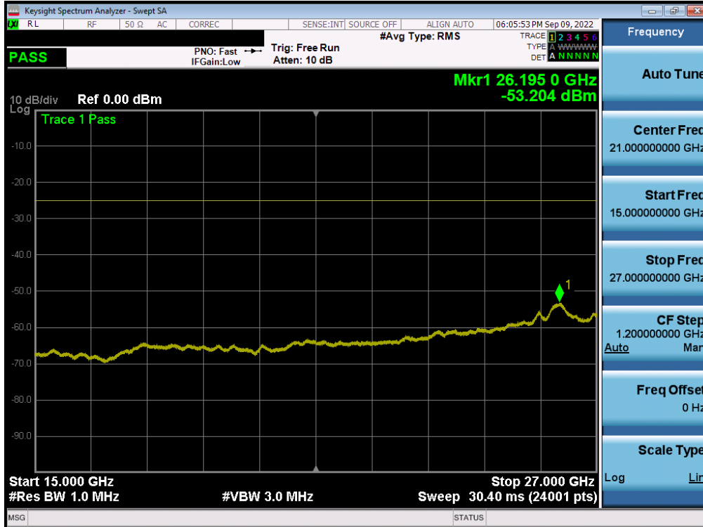
Plot 7-195. Conducted Spurious Plot (LTE Band 7 - 20MHz QPSK - RB Size 1, RB Offset 0 - High Channel - Ant B)
