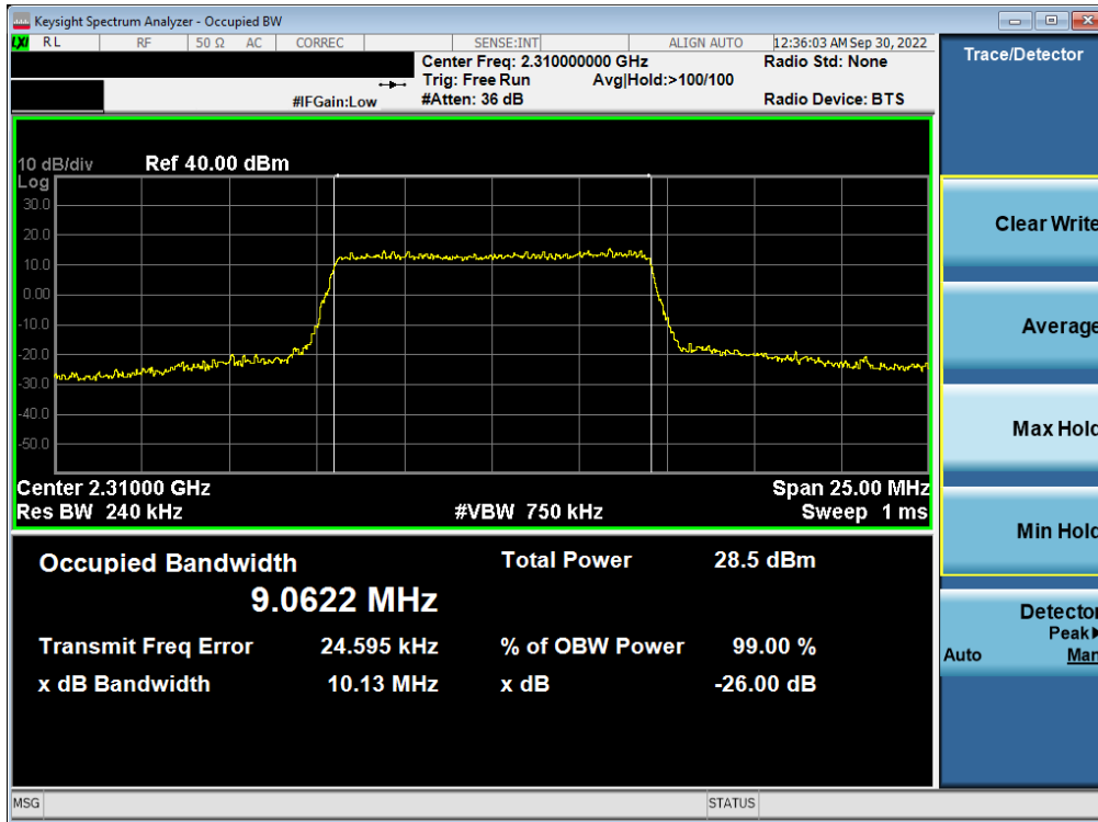
Plot 7-9. Occupied Bandwidth Plot (LTE Band 30 - 10MHz QPSK - Full RB – Ant F)
