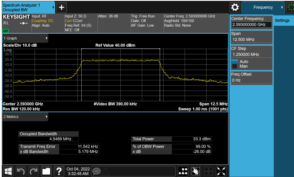
Plot 7-43. Occupied Bandwidth Plot (LTE Band 41(PC2) - 5MHz QPSK - Full RB - Ant F)
