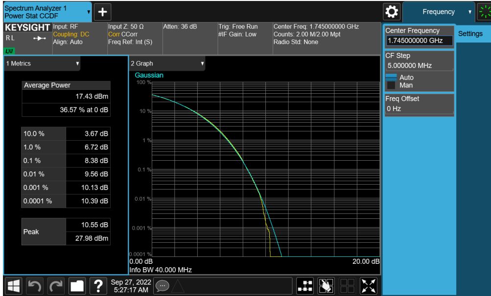
Plot 7-406. PAR Plot (NR Band n66 - 40.0MHz CP-OFDM 256-QAM - Full RB - ANT A)
