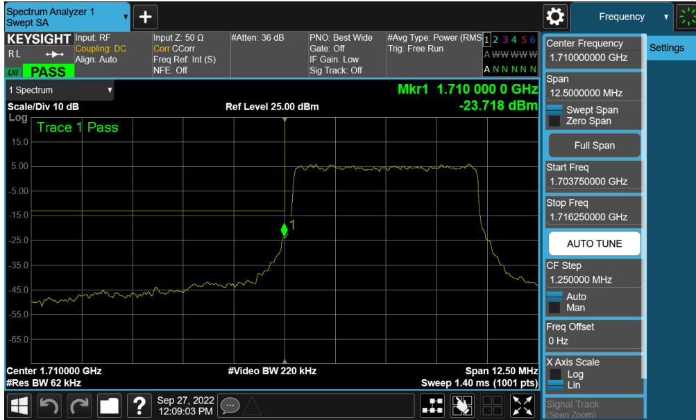
Plot 7-383. Lower Band Edge Plot (NR Band n66 – 5.0MHz - Full RB - Ant F)
