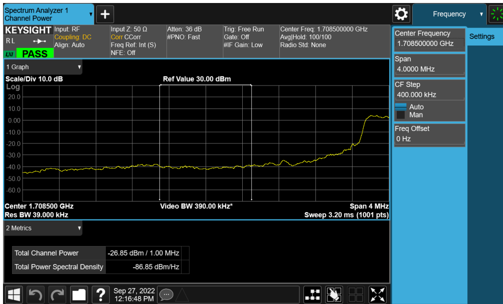
Plot 7-384. Lower Extended Band Edge Plot (NR Band n66 – 5.0MHz - Full RB - Ant F)
