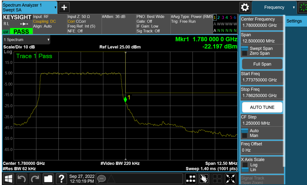
Plot 7-385. Upper Band Edge Plot (NR Band n66 – 5.0MHz - Full RB - Ant F)
