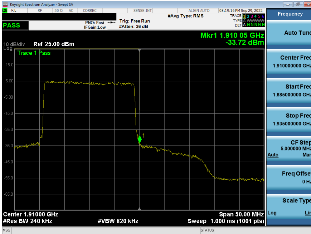
Plot 7-204. Upper Band Edge Plot (LTE Band 2 - 20MHz QPSK – Full RB - Ant F)
