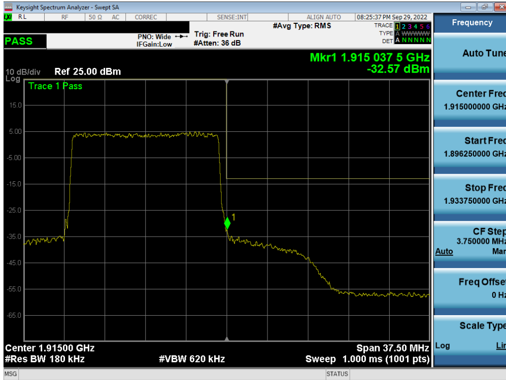
Plot 7-212. Upper Band Edge Plot (LTE Band 25 - 15MHz QPSK – Full RB - Ant F)
