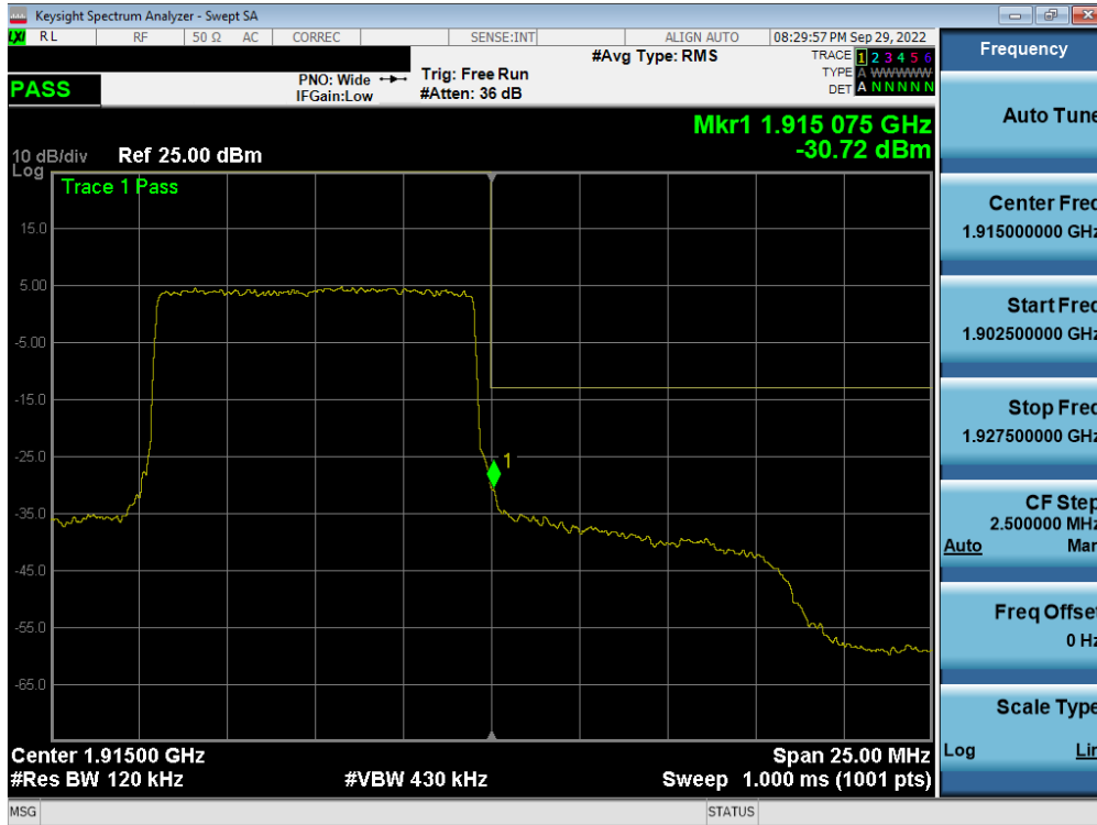
Plot 7-218. Upper Band Edge Plot (LTE Band 25 - 10MHz QPSK – Full RB - Ant F)
