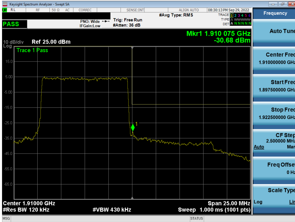
Plot 7-216. Upper Band Edge Plot (LTE Band 2 - 10MHz QPSK – Full RB - Ant F)
