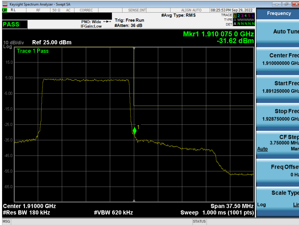
Plot 7-210. Upper Band Edge Plot (LTE Band 2 - 15MHz QPSK – Full RB - Ant F)
