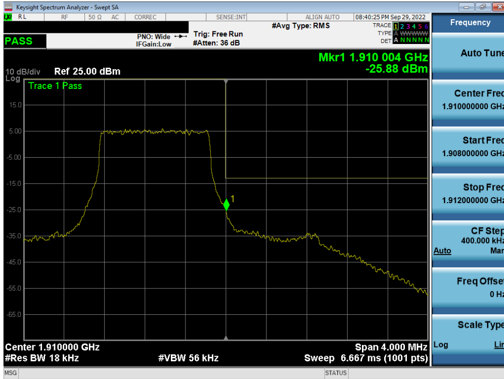
Plot 7-234. Upper Band Edge Plot (LTE Band 2 – 1.4MHz QPSK – Full RB - Ant F)
