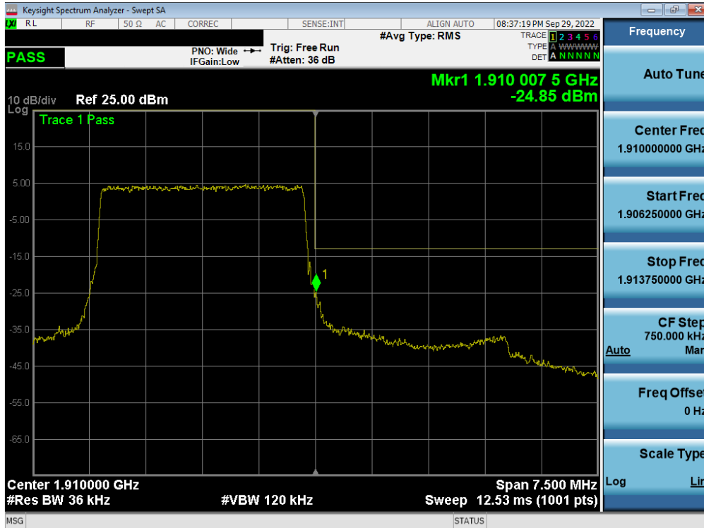
Plot 7-228. Upper Band Edge Plot (LTE Band 2 - 3MHz QPSK – Full RB - Ant F)
