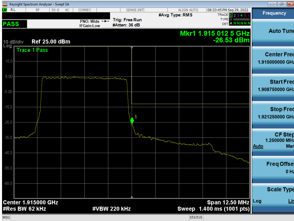
Plot 7-224. Upper Band Edge Plot (LTE Band 25 - 5MHz QPSK – Full RB - Ant F)
