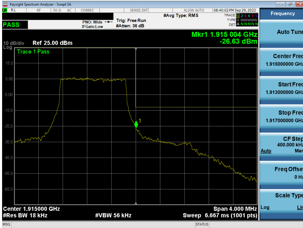
Plot 7-236. Upper Band Edge Plot (LTE Band 25 – 1.4MHz QPSK – Full RB - Ant F)
