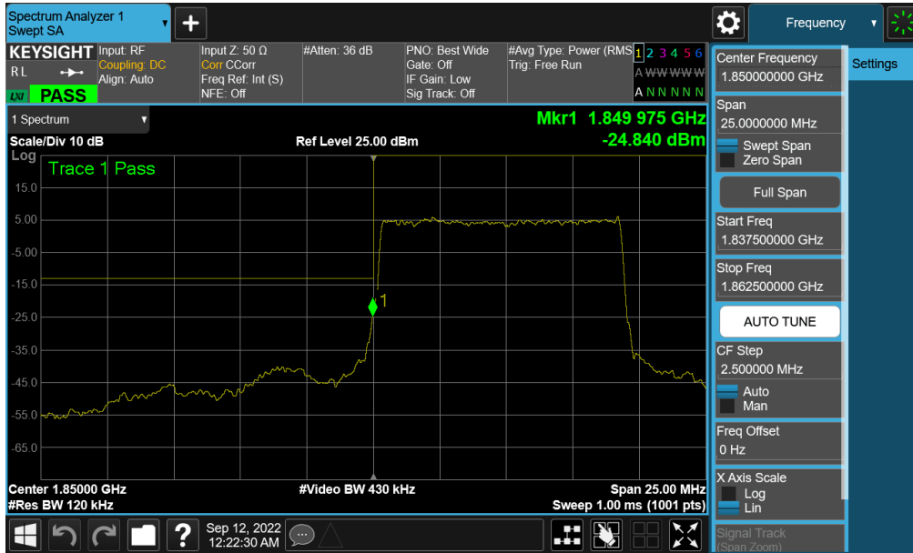
Plot 7-184. Lower Band Edge Plot (NR Band n25/2 - 10MHz QPSK – Full RB - Ant A)
