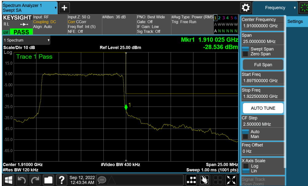
Plot 7-186. Upper Band Edge Plot (NR Band n2 - 10MHz QPSK – Full RB - Ant A)
