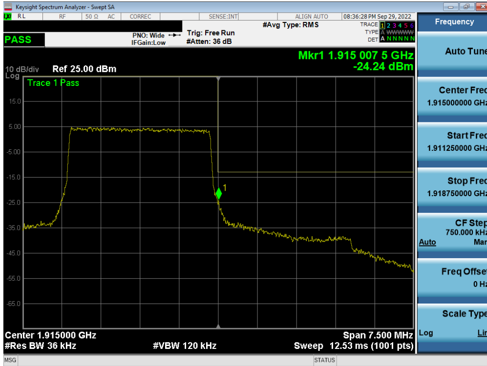
Plot 7-230. Upper Band Edge Plot (LTE Band 25 - 3MHz QPSK – Full RB - Ant F)
