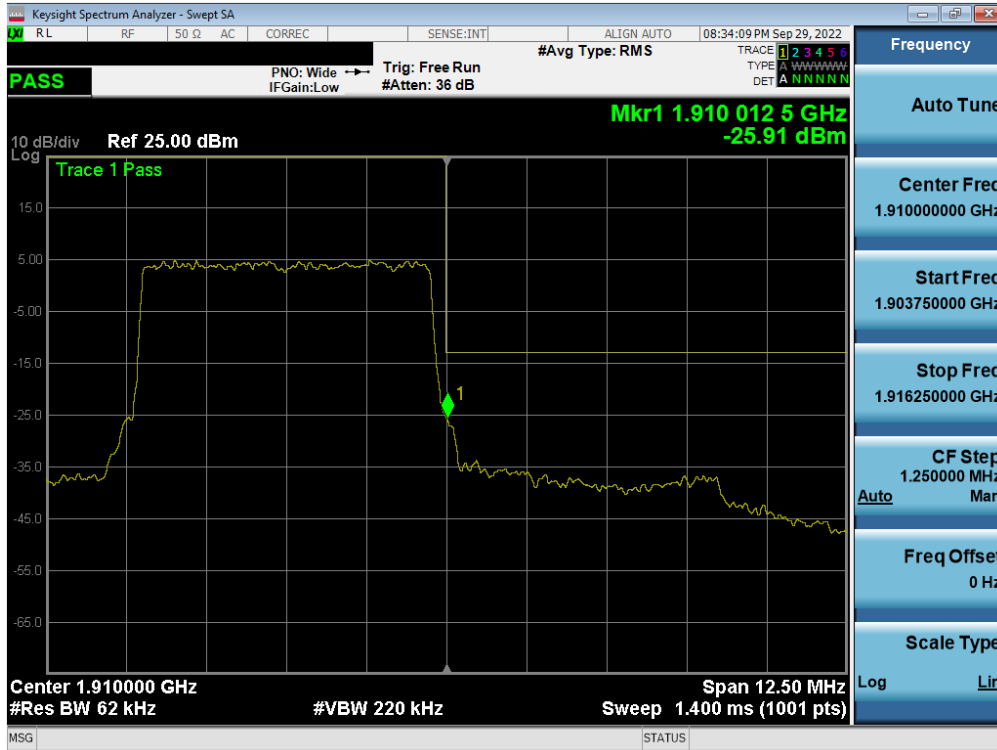
Plot 7-222. Upper Band Edge Plot (LTE Band 2 - 5MHz QPSK – Full RB - Ant F)
