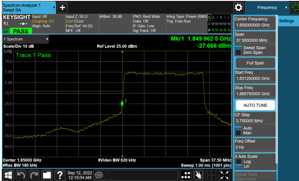
Plot 7-178. Lower Band Edge Plot (NR Band n25/2 - 15MHz QPSK – Full RB - Ant A)
