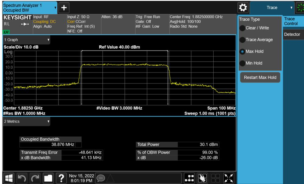
Plot 7-15. Occupied Bandwidth Plot (NR Band n25 - 40.0MHz CP-OFDM 16QAM - Full RB - Ant A)
