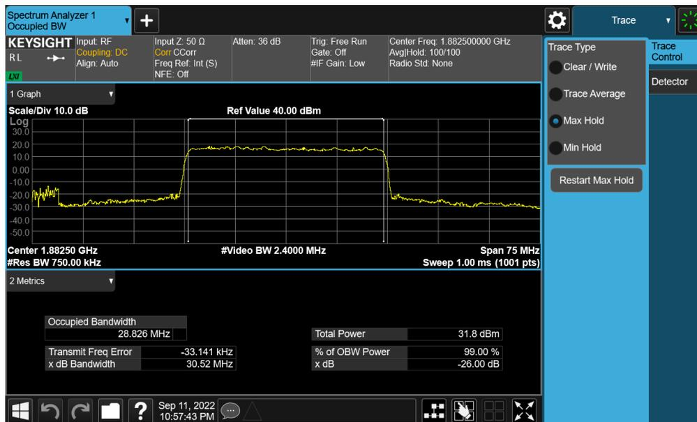
Plot 7-16. Occupied Bandwidth Plot (NR Band n25 - 30.0MHz DFT-s-OFDM BPSK - Full RB - Ant A)
