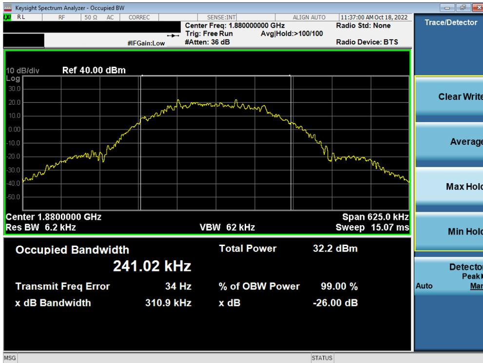
Plot 7-35. Occupied Bandwidth Plot (EDGE, Ch. 661)
