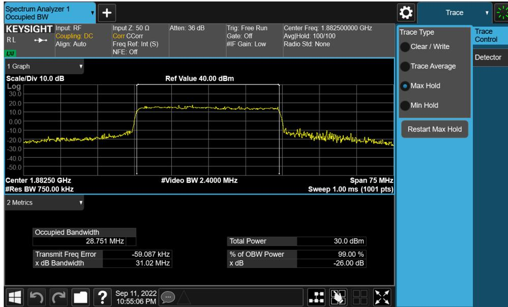
Plot 7-17. Occupied Bandwidth Plot (NR Band n25 - 30.0MHz CP-OFDM QPSK - Full RB - Ant A)
