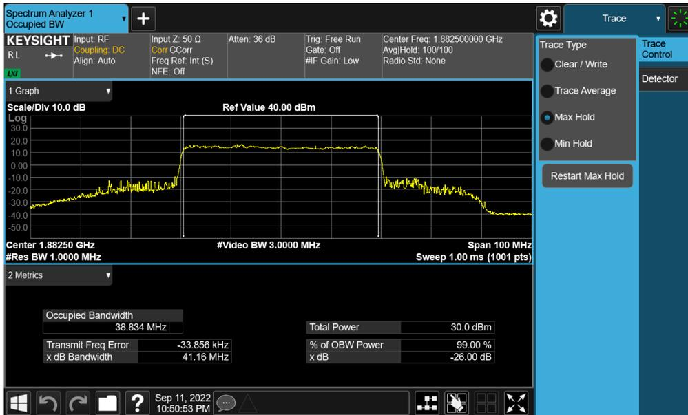
Plot 7-14. Occupied Bandwidth Plot (NR Band n25 - 40.0MHz CP-OFDM QPSK - Full RB - Ant A)
