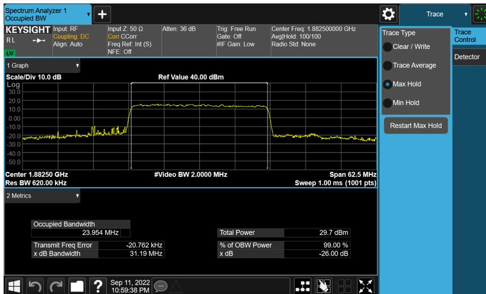
Plot 7-20. Occupied Bandwidth Plot (NR Band n25 - 25.0MHz CP-OFDM QPSK - Full RB - Ant A)
