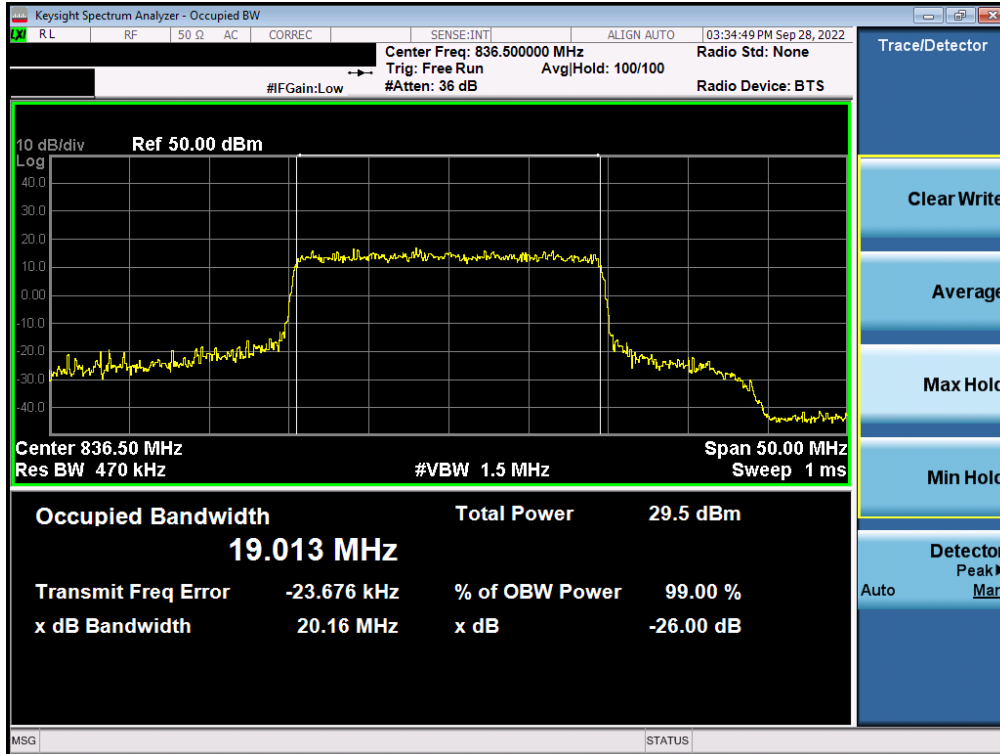
Plot 7-13. Occupied Bandwidth Plot (NR Band n26/5 - 20MHz 16-QAM - Full RB Configuration)
