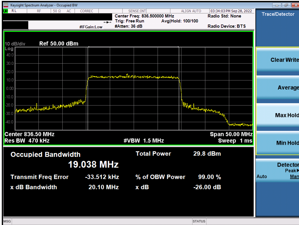
Plot 7-12. Occupied Bandwidth Plot (NR Band n26/5 - 20MHz QPSK - Full RB Configuration)
