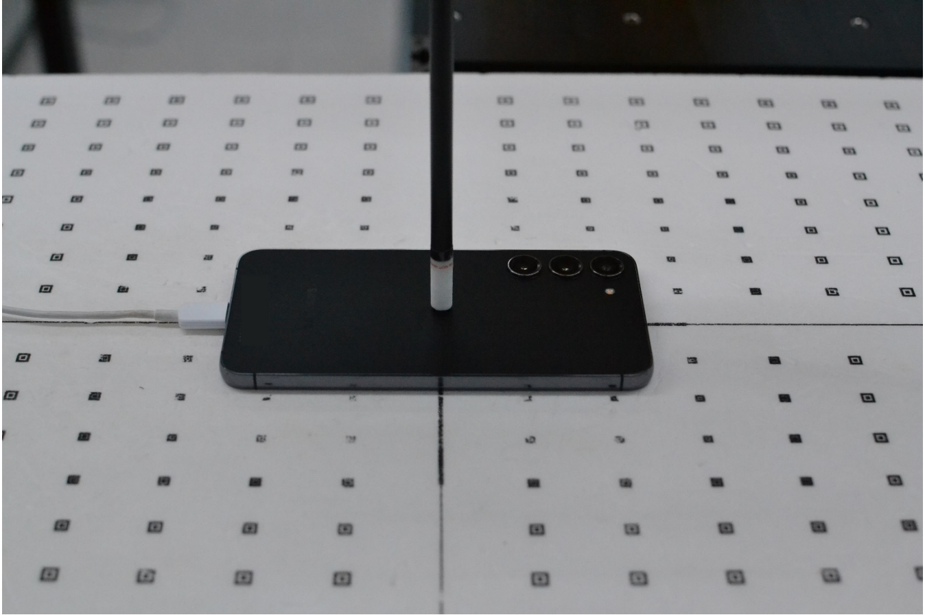
Figure E-4 Near Field Power Density Test Setup Photo – Back Side at 2 mm
