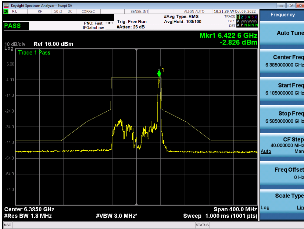
Plot 7-445. In-Band Emission Plot MIMO ANT1 (80MHz BW 802.11ax (26 Tones) (UNII Band 5) – Ch. 87) – LPI
