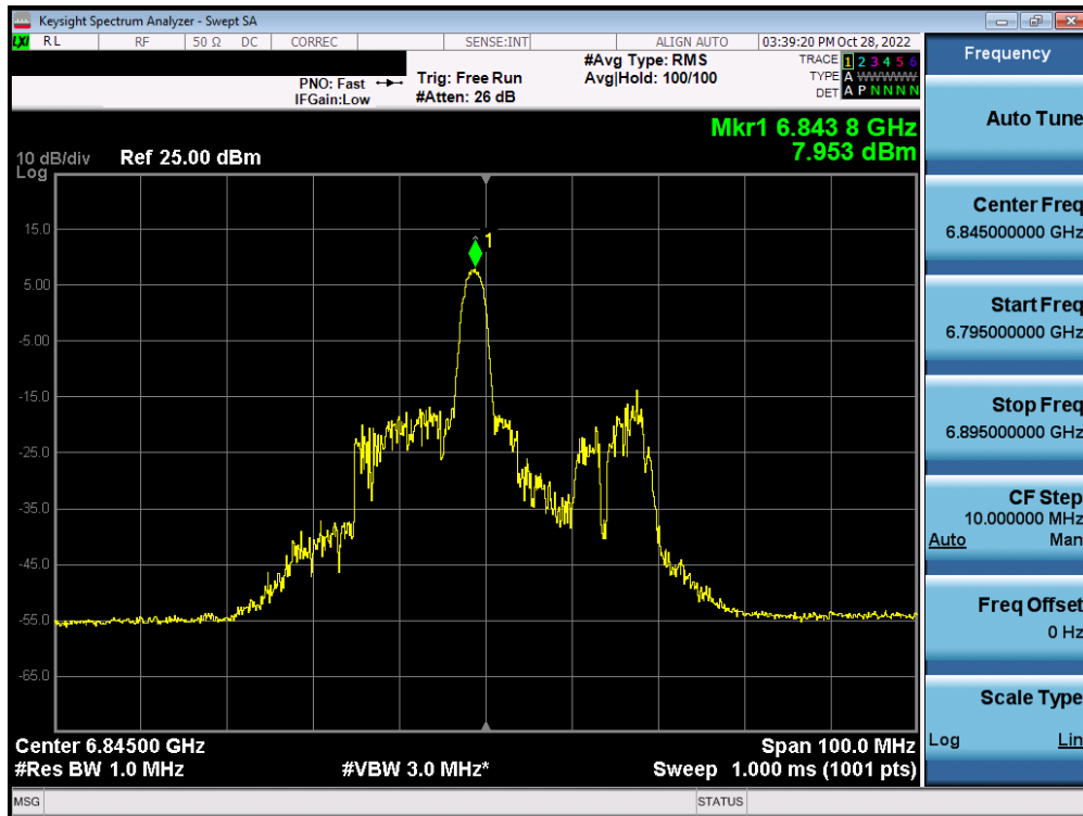
Plot 7-385. Power Spectral Density Plot MIMO ANT2 (40MHz BW 802.11ax (26 Tones) (UNII Band 7) – Ch. 179) – SP
