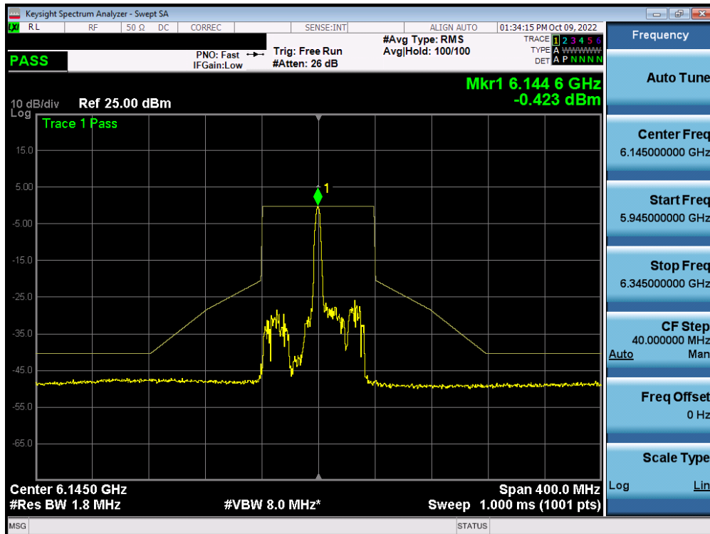
Plot 7-444. In-Band Emission Plot MIMO ANT1 (80MHz BW 802.11ax (26 Tones) (UNII Band 5) – Ch. 39) – LPI
