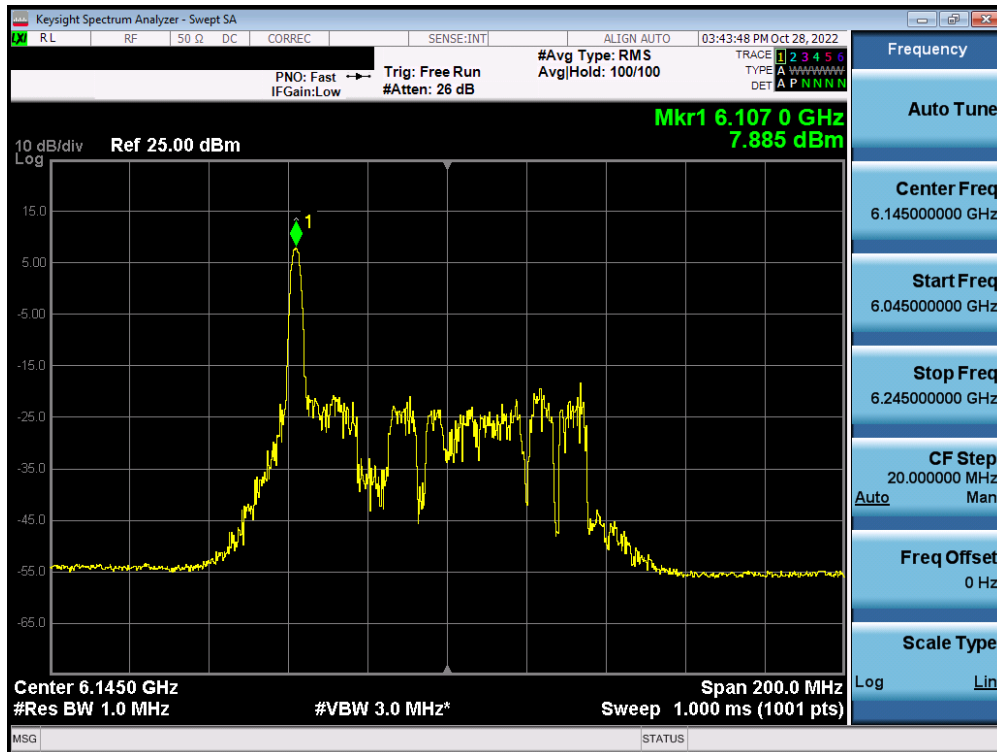
Plot 7-375. Power Spectral Density Plot MIMO ANT2 (80MHz BW 802.11ax (26 Tones) (UNII Band 5) – Ch. 39) – SP
