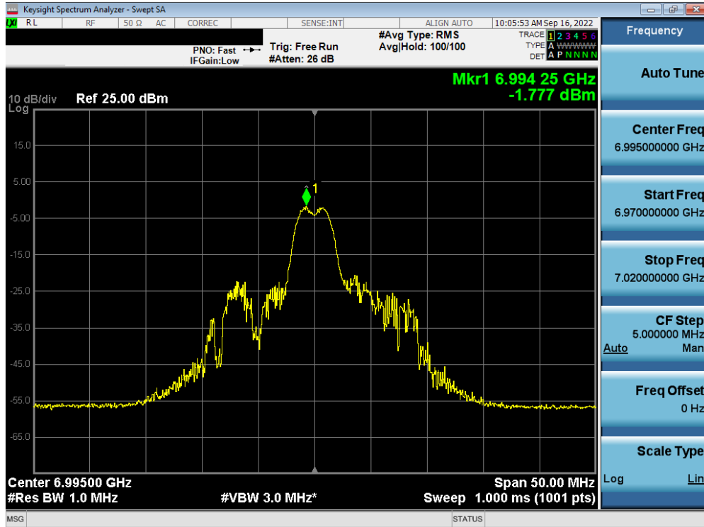
Plot 7-360. Power Spectral Density Plot MIMO ANT2 (20MHz BW 802.11ax (26 Tones) (UNII Band 8) – Ch. 209) – LPI
