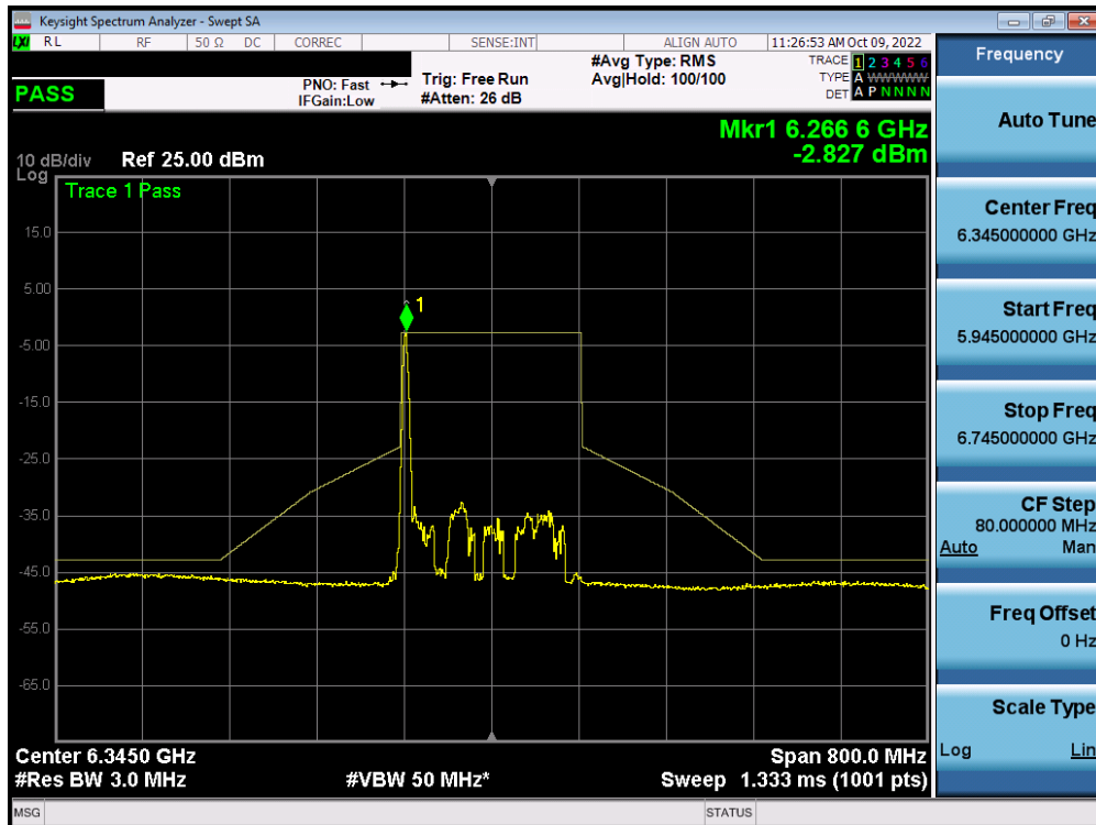
Plot 7-448. In-Band Emission Plot MIMO ANT1 (160MHz BW 802.11ax (26 Tones) (UNII Band 5) – Ch. 79) – LPI
